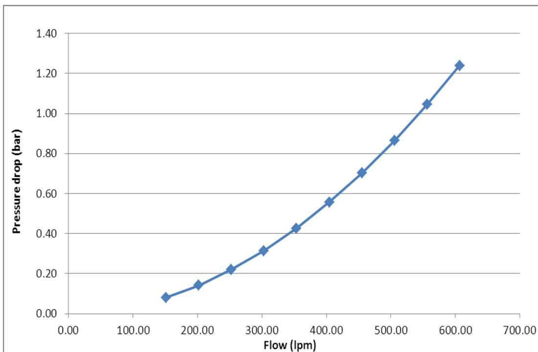
Figure 3: Pressure drop curve over the engine
