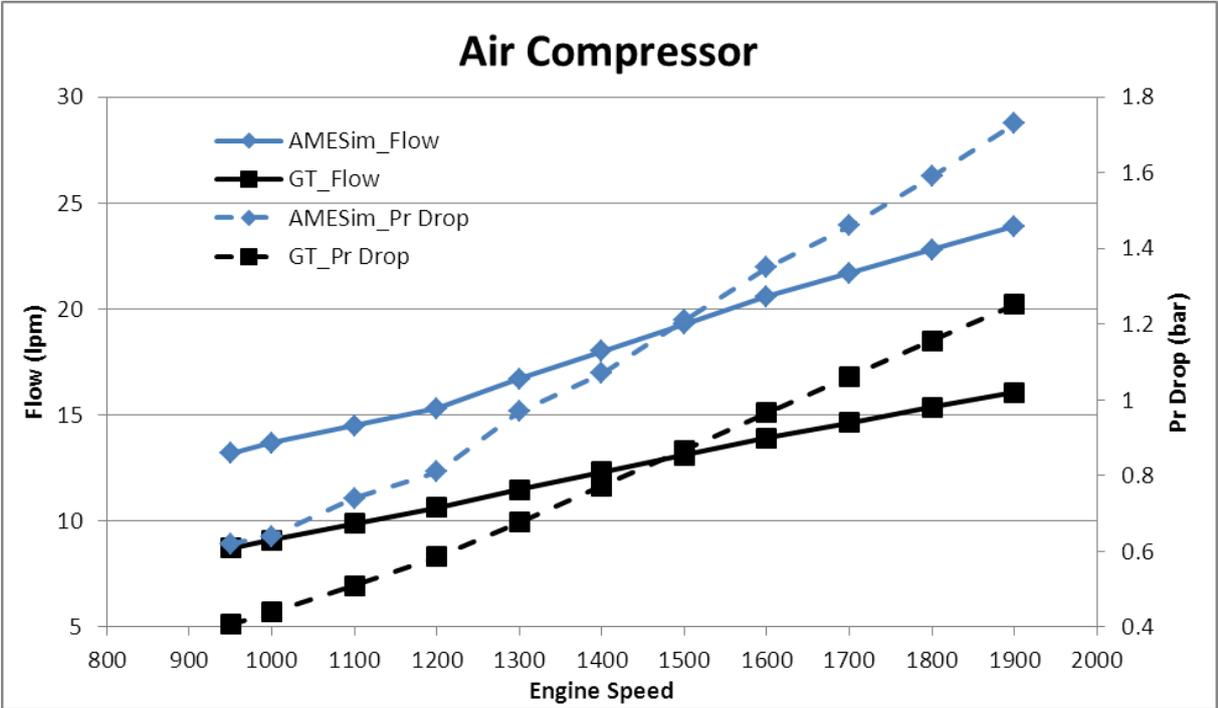
The reason for such a huge divergence in the above air compressor result is the difference in pressure drop values between the two tools. Added to this is the overall lower flow rate caused due to the low flow rate from the coolant pump as shown in GT Cool. The same reason can be attributed to the results of transmission oil cooler shown below.
