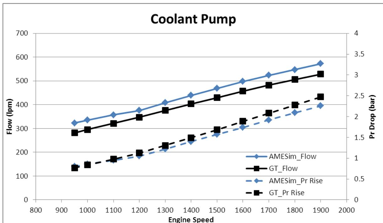
Figure 14: Pressure Rise, Flow Vs Engine speed
