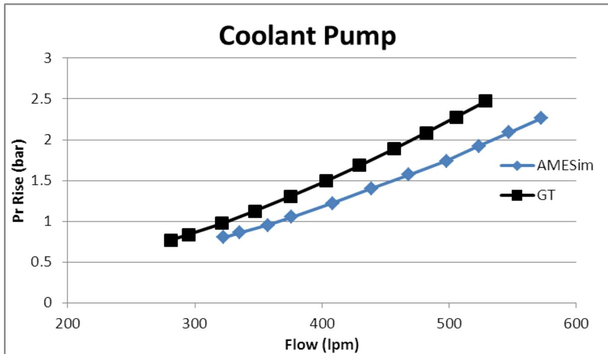
Figure 15: Pressure rise Vs Flow
