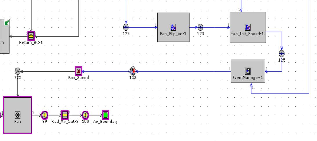
Event Manager basically evaluates the coolant temperature and based on that, controls the fan speed. This way of implementation lead to a lot of fluctuations as the whole system reacts a bit slowly from the Event Manager. The front radiator, charge air cooler, main radiator and fan cluster is arranged in the following manner as per the architecture shown in Figure 12 below.
