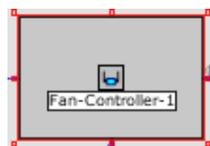
The PID controller is used in the model to control the fan speed. The PID controller based on the Proportional, Integral gains tries to bring the fan speed to a steady state value. In general the Derivative gain is not used and set to 'ign' (ignore) in the element. Basically it tries to bring the input signal to a value such that a target parameter can be achieved as soon as possible.
