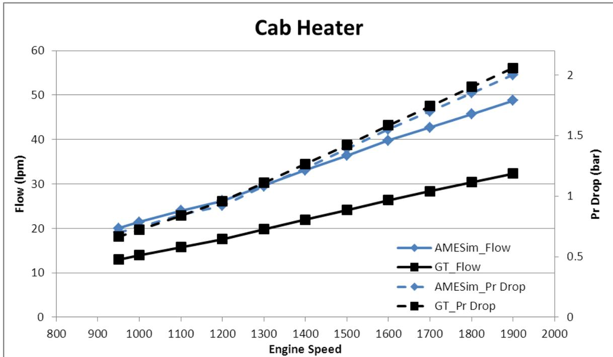
The flow through cab heater shown by GT Cool is low compared to AMESim which is attributed to overall low flow coming from the coolant pump. The reason why the pressure drop curve is matching is because of the additional pressure drop calculated by GT Cool in pipe/hoses connecting the cab heater which inturn actually lifts the GT Cool curve and matches it with AMESim.
