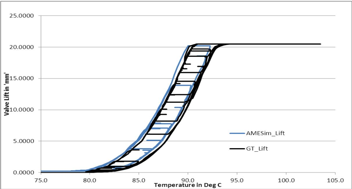
Figure 26: Thermostat lift fluctuation - AMESim Vs GT Cool
