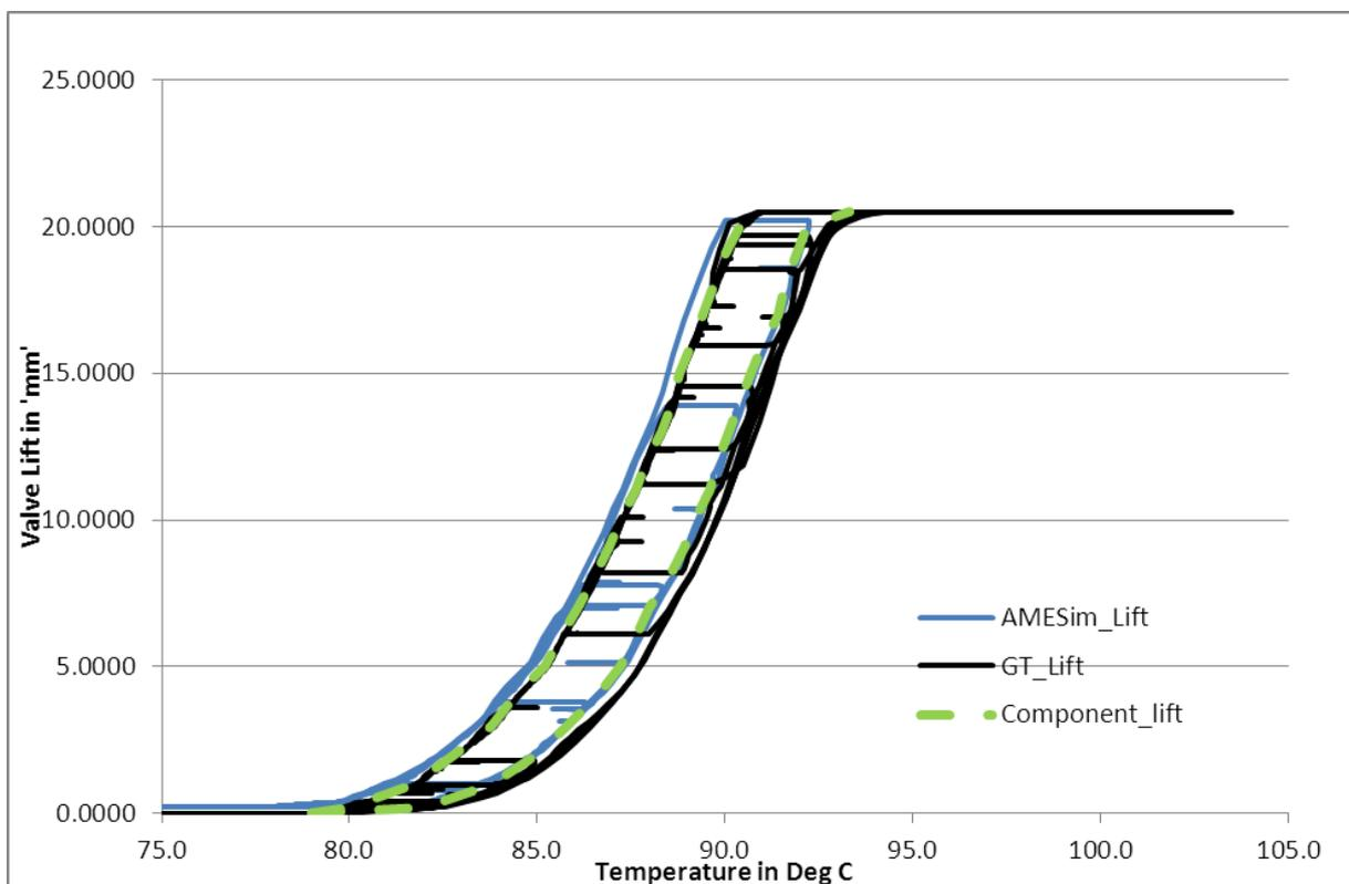
Figure 24: Thermostat lift fluctuation and hysteresis curve
