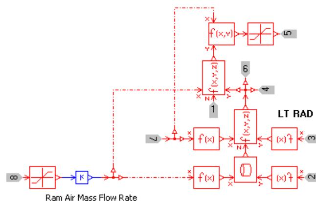
The inputs 2 and 8 which are the mass flow rate of ram air and mass flow rate of coolant are fed into the performance map of the front radiator which gives the heat load data. But the performance map is generated for the radiator at a temperature difference (between coolant and ram air temp) of 50 deg Celsius and hence the heat load values generated from the map needs to be adjusted for the real temperature difference occurring in the model. Similar
