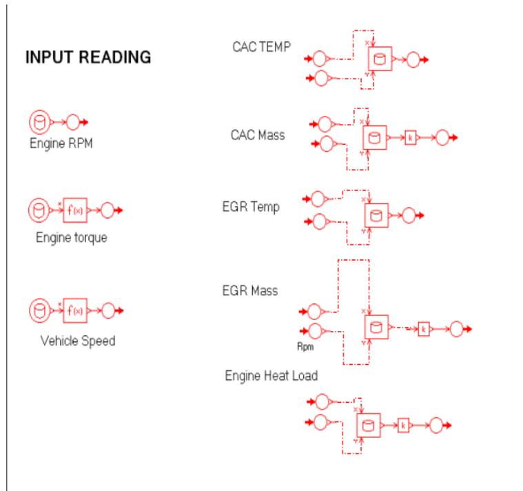
Figure 8: Input data as seen in AMESim
