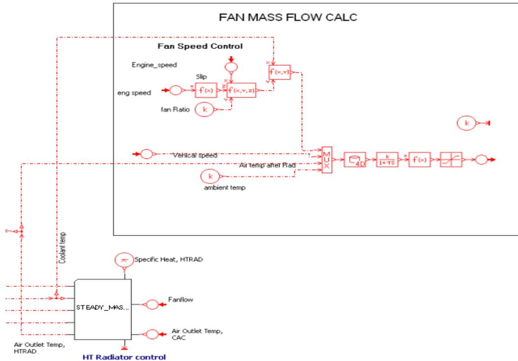
Figure 10: Fan model as implemented in AMESim
