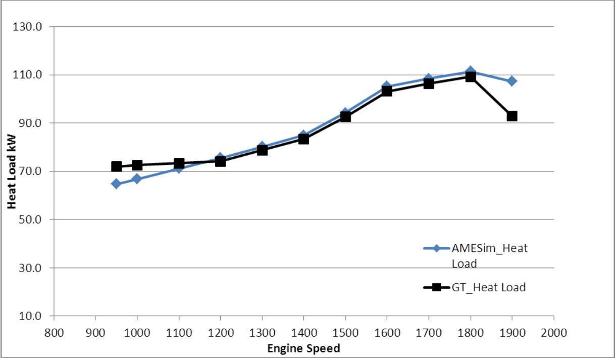
Figure 19: EGR Cooler Heat load
