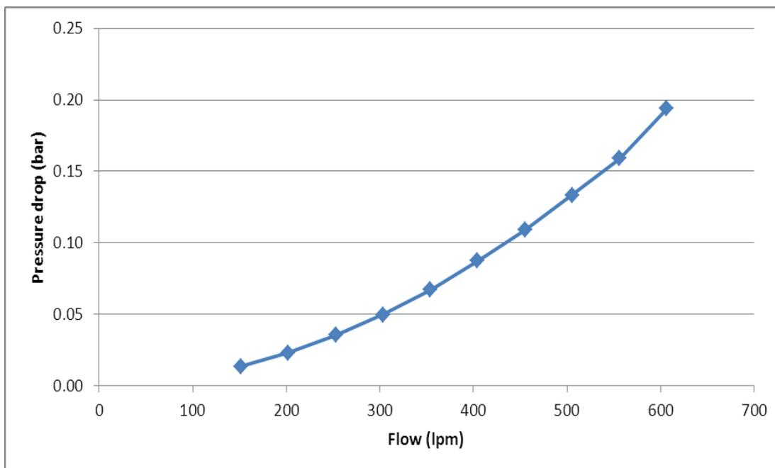
Figure 7: Pressure drop over Engine Oil cooler
