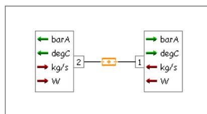
This particular element is used extensively in the model representing the coolant pipes and hoses. This represents the pressure loss in a pipe due to friction. The basic inputs to this element are the diameter, initial temperature, initial pressure, relative roughness, wall thickness etc. The output of this element is the Flow rate, temperature at both inlet and outlet, pressure at inlet and outlet, Reynolds number etc.
