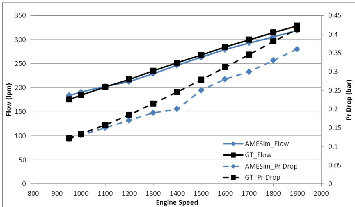
Figure 18: Pressure drop across engine
