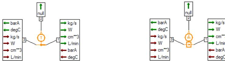
The element above represents the temperature and mass flow sensors. It has the pressure and temperature as inputs. The out puts include mass flow rate, temperature etc.
