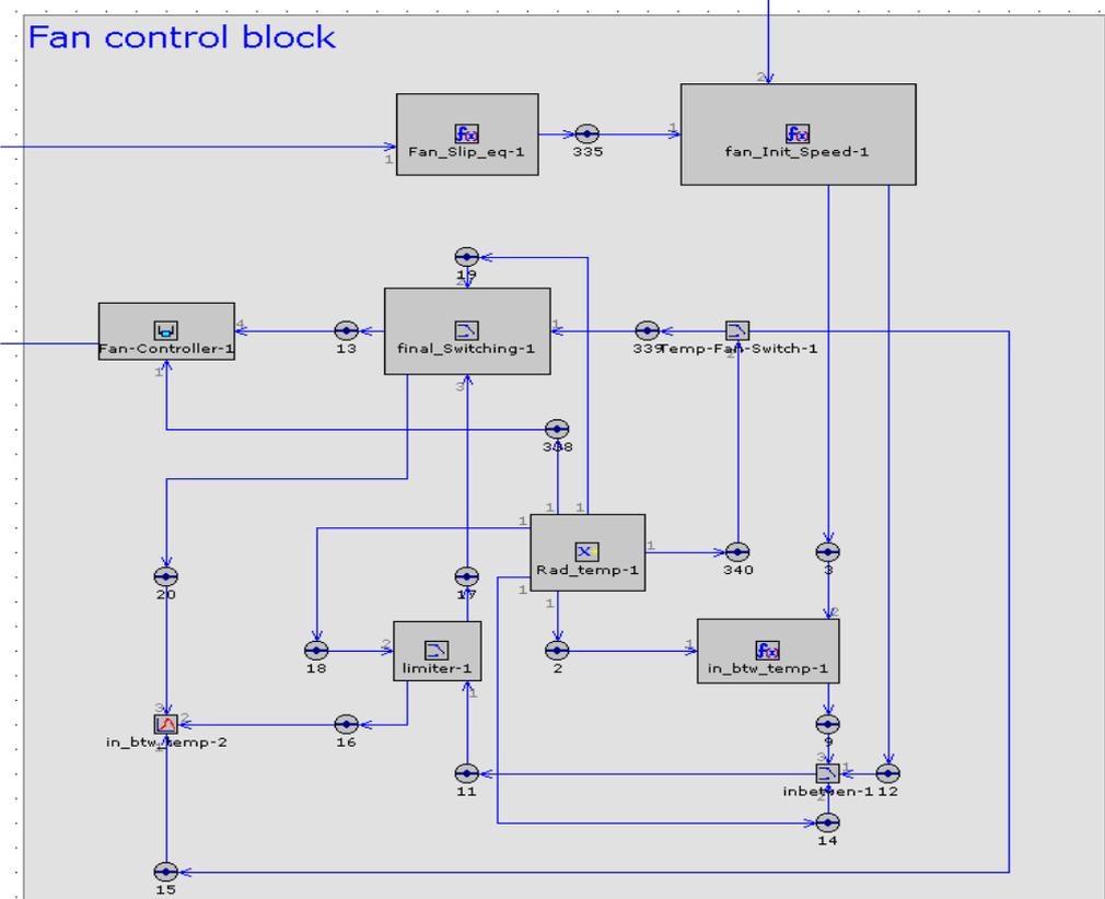
Figure 11: Fan model as implemented in GT Cool
