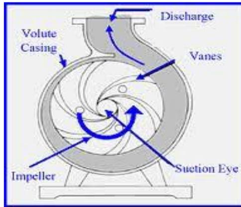
The pump has two components namely the impeller and the diffuser or volute. The impeller generates the kinetic energy and the diffuser converts into a pressure energy, which means the pump makes the coolant flow at particular flow rate and pressure through the circuit. The pump characteristic curve is shown in Figure 4 where each curve represents different pump speed.
