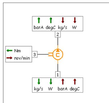
This element represents the centrifugal pumps generally used in automobile applications. The inputs to this element include a file which basically is a series of 3D data representing the
