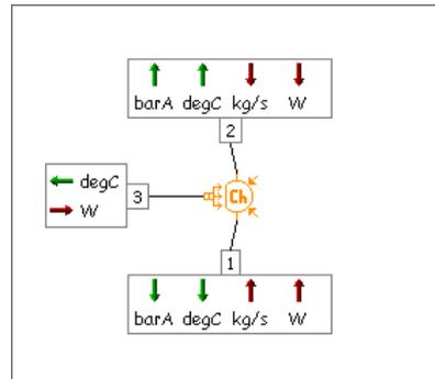
This element represents the volume, for example the coolant volume in the engine block, coolant volume in the radiator etc. The input include, pressure, temperature and the coolant volume. The output includes mass flow rate, Heat load, pressure etc.
