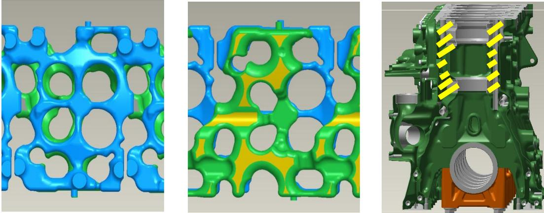
Figure 9: Cylinder Head and Block coolant flow geometry
