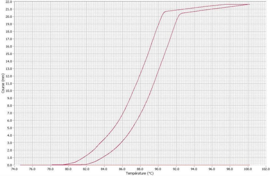
Figure 5: Thermostat hysteresis curve
