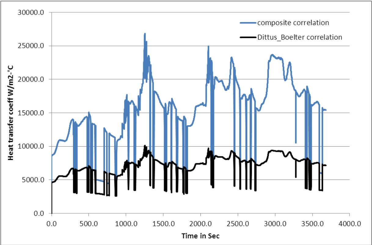
Figure 32: Standard Heat transfer coeff Vs Composite correlation – For Cylinder Head
