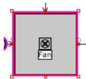
The above element is used to model the fan. The data is given in the form of a map which basically includes parameters like fan speed, mass flow rate, pressure rise and efficiency of the fan. In the model, the fan speed has been controlled using a PID controller.
