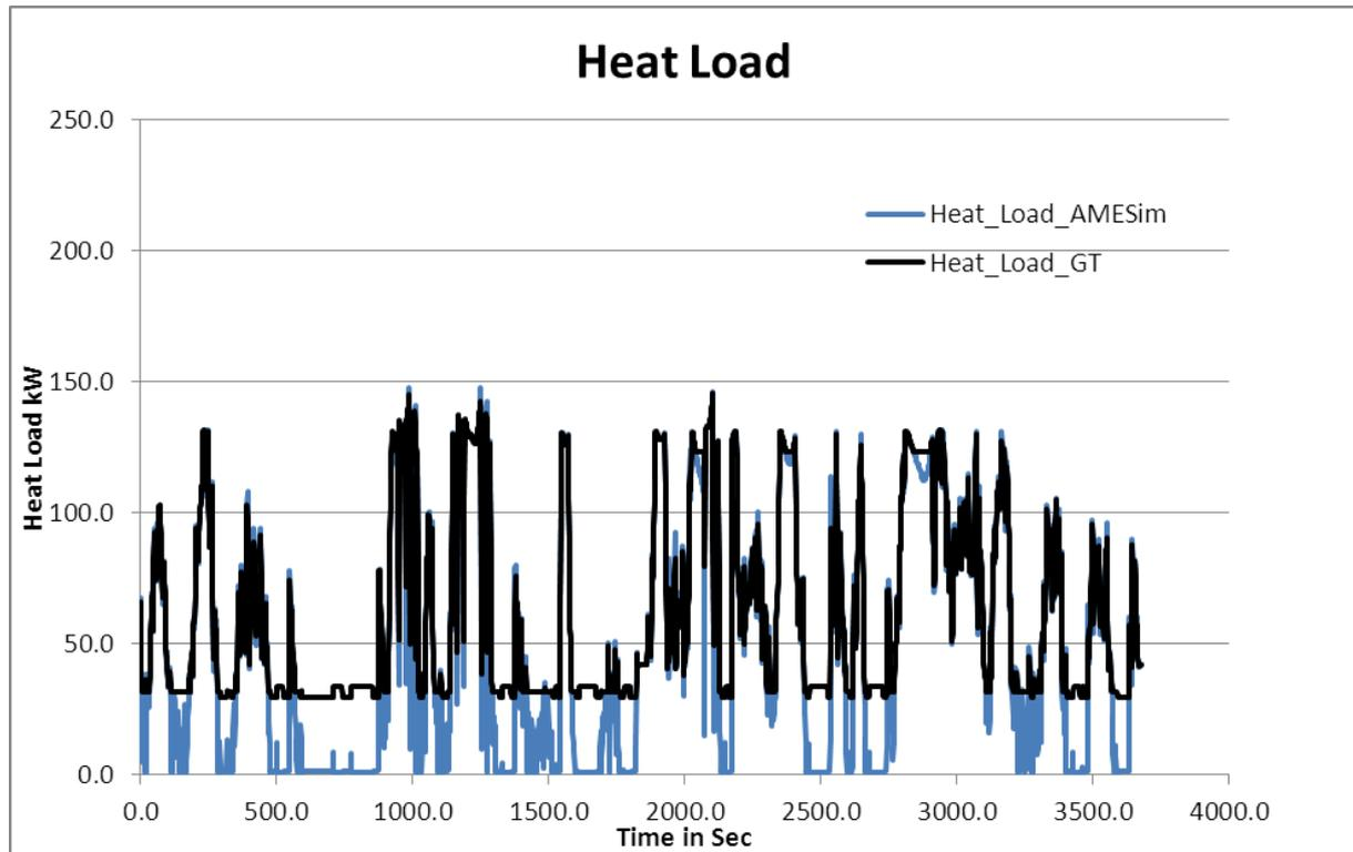
As was discussed in the steady state simulations, GT Cool does not extrapolate the heat load values outside the boundary data set in the map and instead outputs the boundary data set in the map for all inputs outside the boundary data. In this case, the boundary is set in terms of torque and engine speed. It can be seen that for all values within this bounds, both the tools gives similar results, but for inputs outside the bounds, both the tools follows different procedure.
