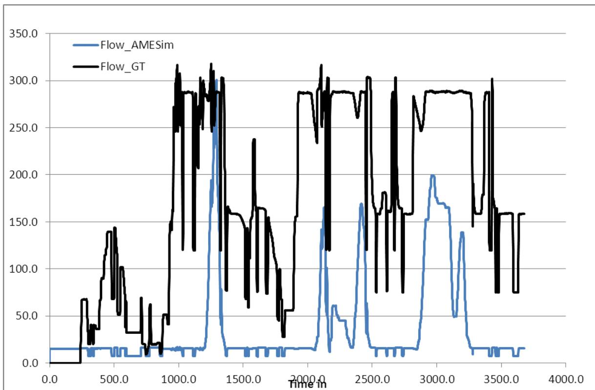
Figure 27: Coolant flow through Radiator
