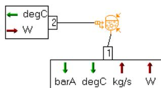
This element is the thermal hydraulic accumulator which is used as an expansion tank in the model. As the expansion tank has two volumes involved (gas and coolant), here also the inputs include the volume of coolant present in the whole accumulator volume.
