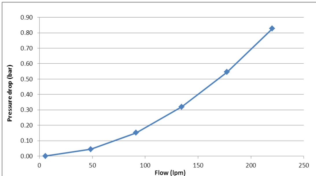
Figure 6: Pressure drop over the EGR cooler
