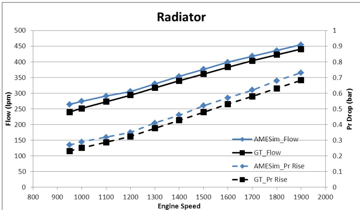
The flow and pressure drop values across the radiator shown by both the tools follows the same trend as shown in the results for the coolant pump. Similar results were found for retarder circuit which is in series to the radiator. But the results above have been shown for an
