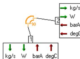
This element is used to simulate bends in the pipes. AMESim library has basically 3 different types of bends – 90 deg, 45 deg and 30 deg apart from a generic element where user defined angles can be used. The main input to this element is the radius of curvature and diameter. As an output, one gets mass flow rate at inlet and outlet, pressure at inlet and outlet, temperatures at inlet and outlet etc.
