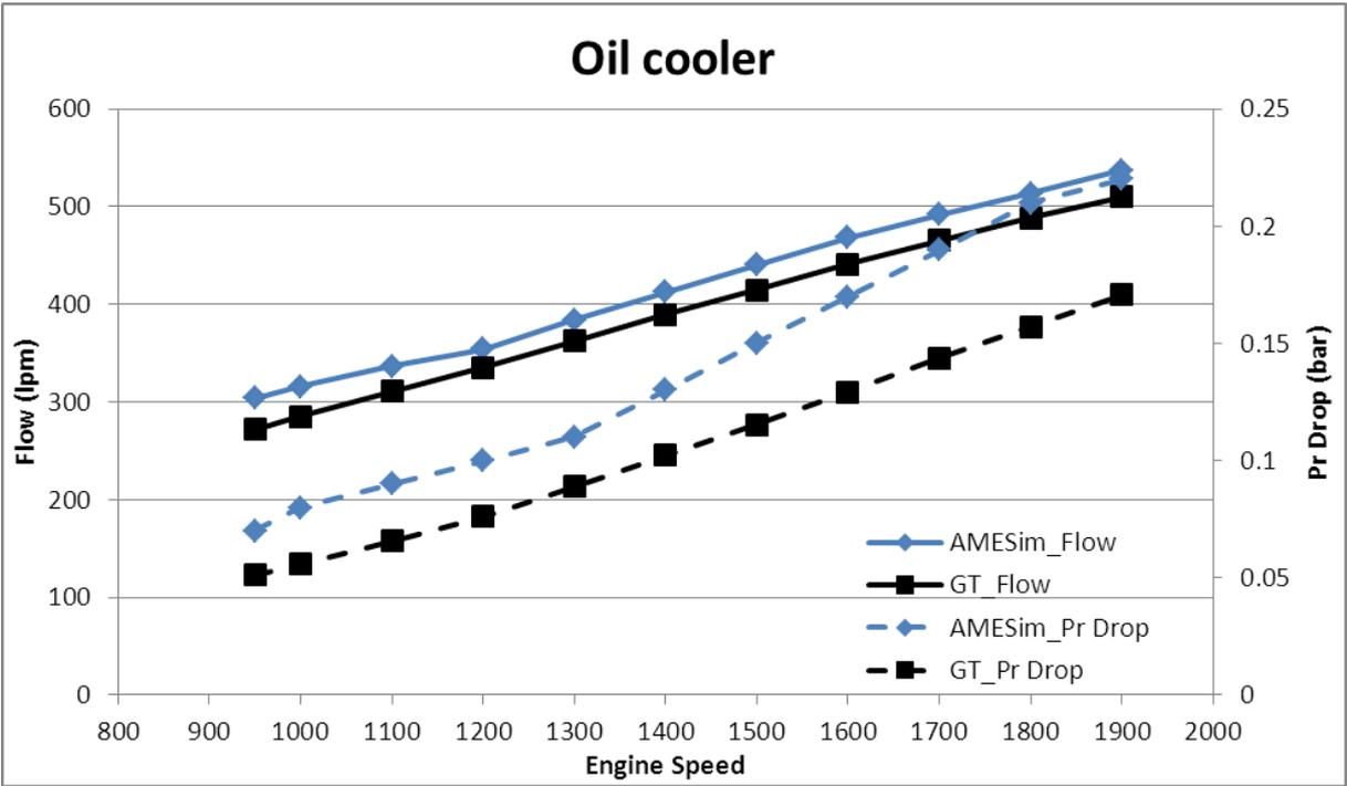
The lower coolant flow rate from the coolant pump shown by GT Cool results in a lower coolant flow rate across oil cooler. As shown in the graph above the flow through oil cooler is lower resulting in a lower pressure drop as compared to the result in AMESim.
