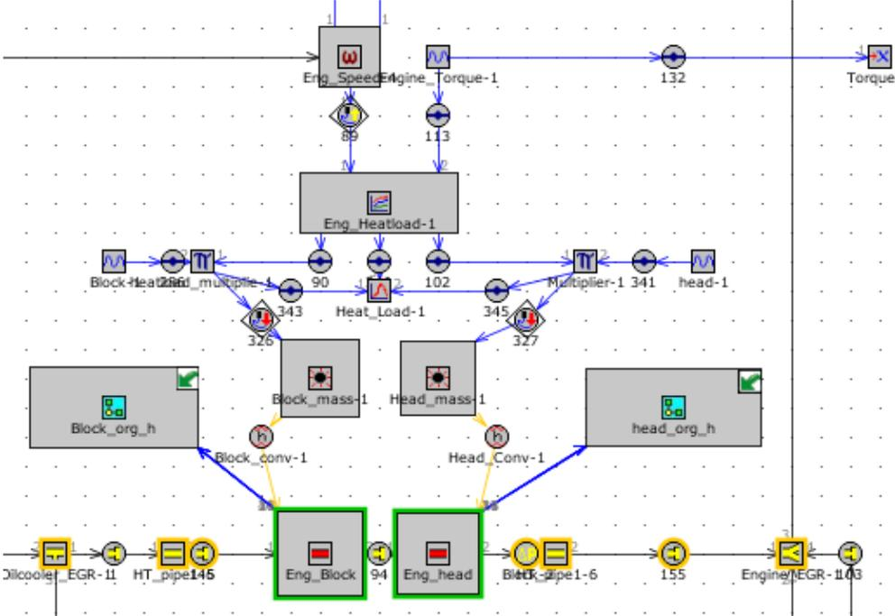
Figure 13: Coposite correlation implementation for Engine warm up behaviour representation
