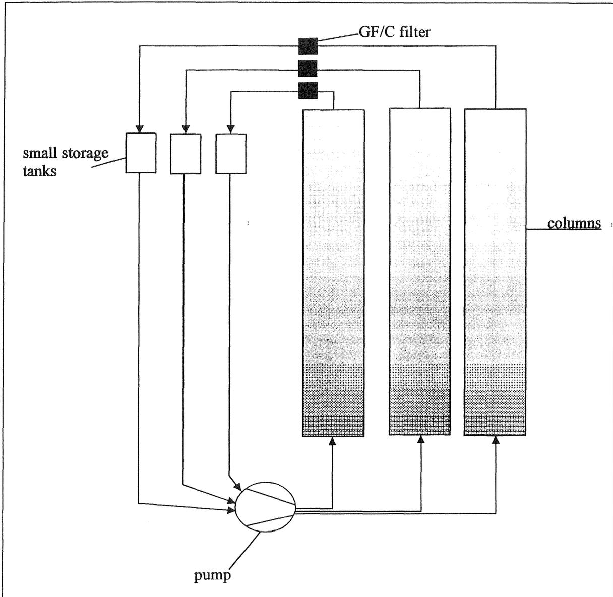
Figure 4 Set-up of the testing plant for the recirculation experiments including a filter system
