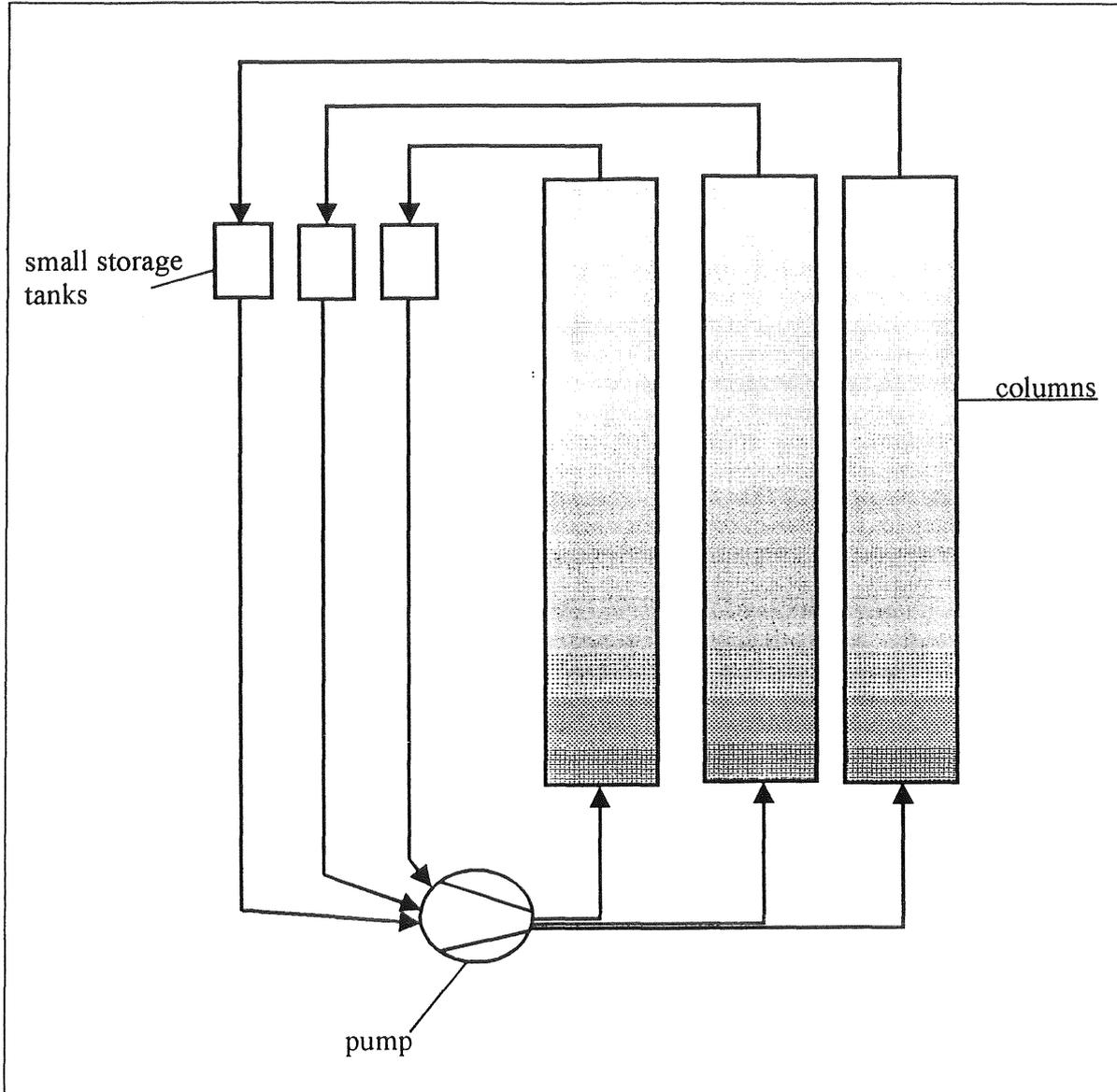
Figure 3 Set-up of the testing plant for the recirculation experiments
