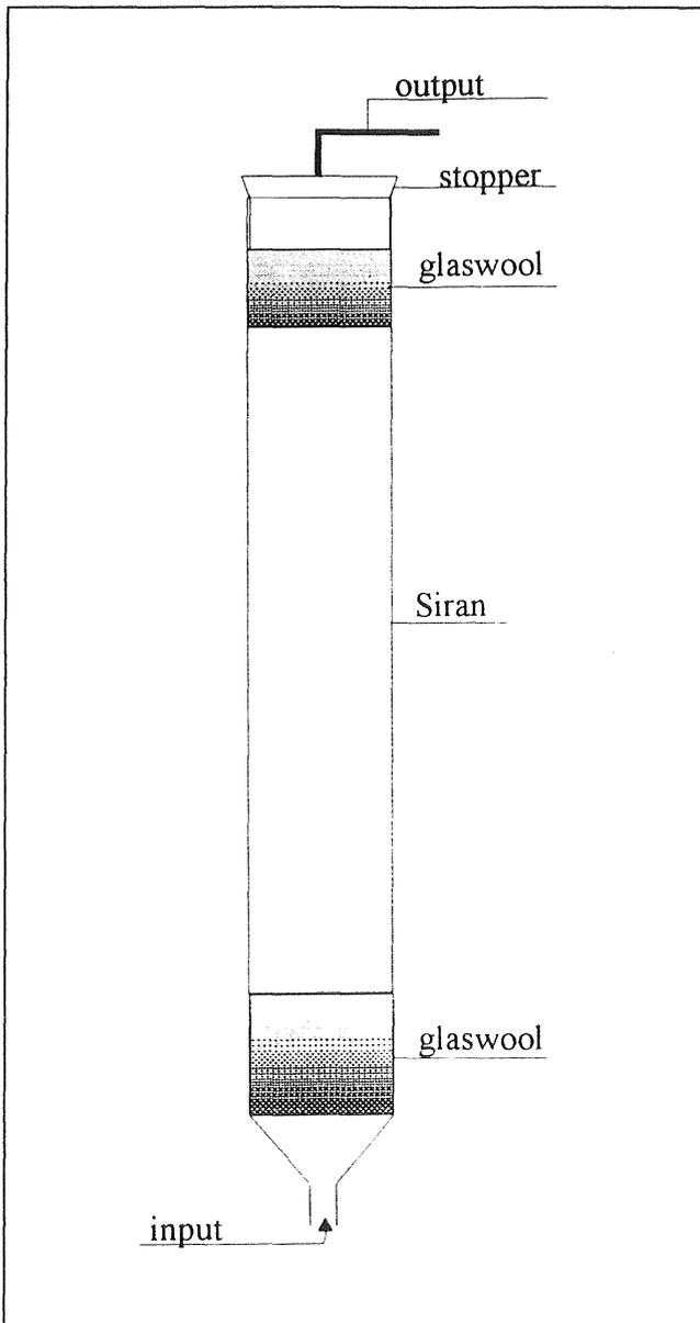
For the study a continuous flow biofilm reactor (CFBR) has been used. Six reactors were constructed (three for each sampling site) after the description of Kaplan and Newbold (1995) from 63 cm sections of 2.5 cm diameter glass tubes (see figure 1) with a volume of 310 cm<sup>3</sup>.
