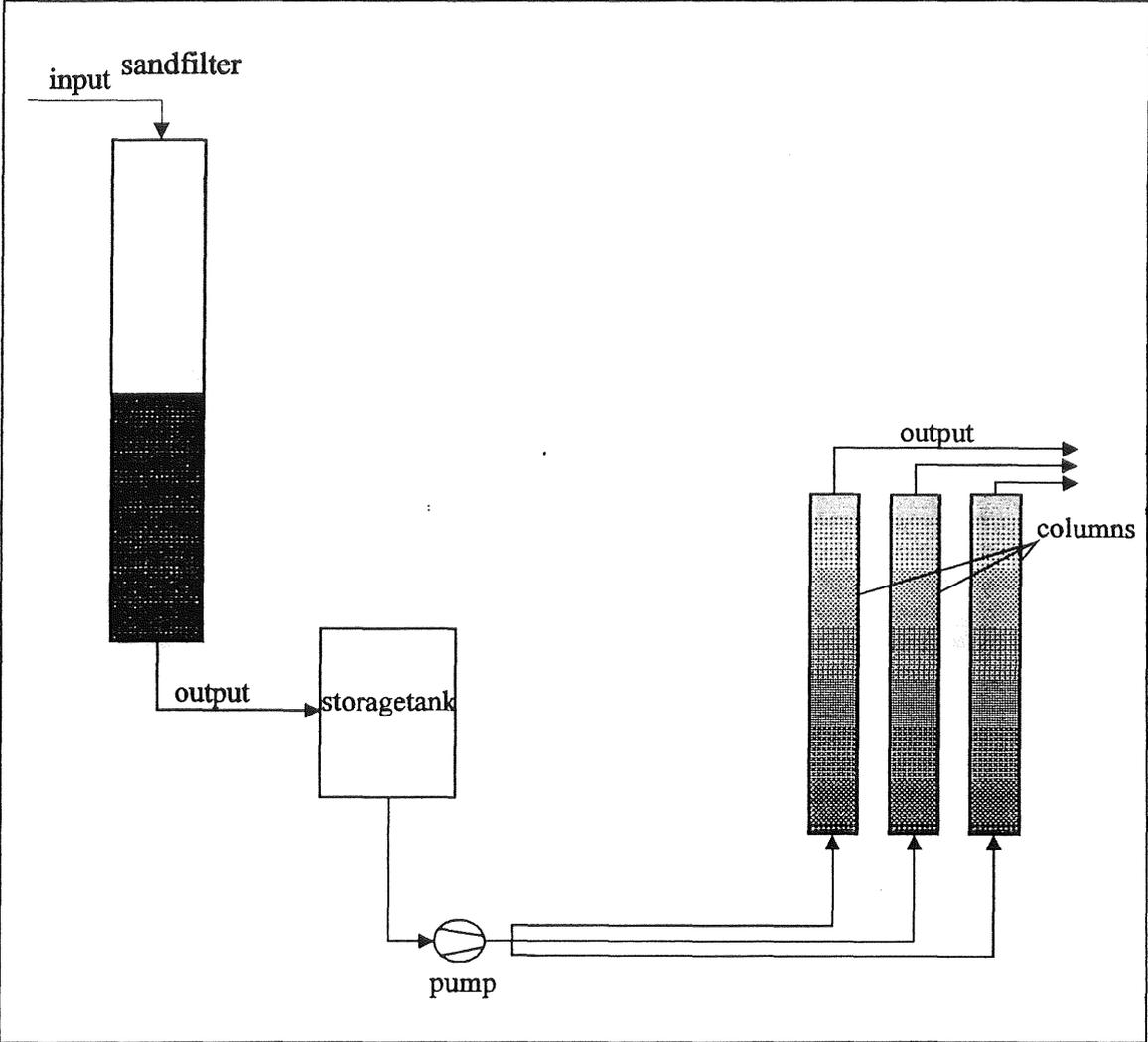
Figure 2 Set-up of the testing plant
