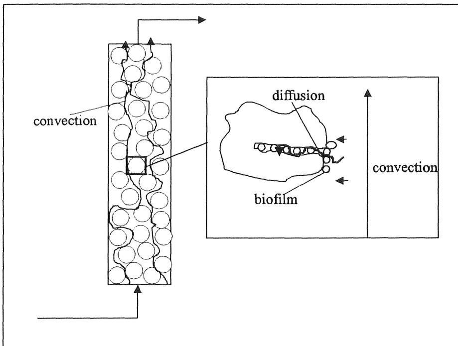
Figure 20 Convective and diffusive transport mechanisms in the columns
