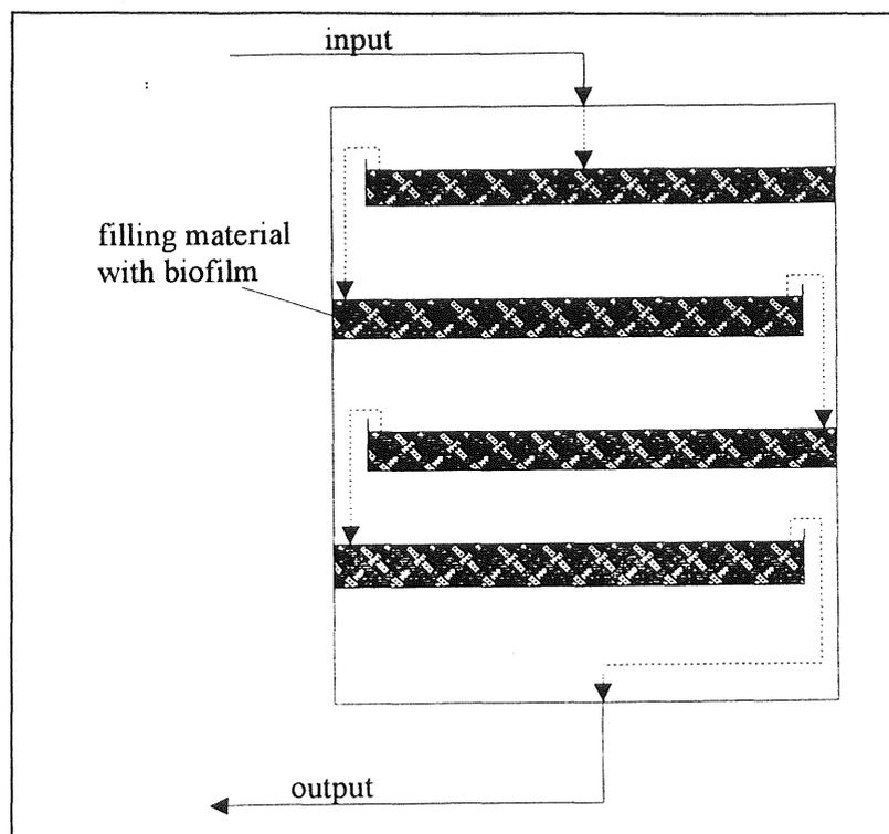
Figure 22 Semi-batch bioreactor
