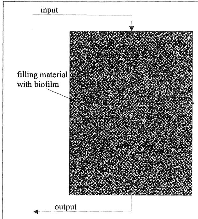
Figure 23 Trickling bioreactor
