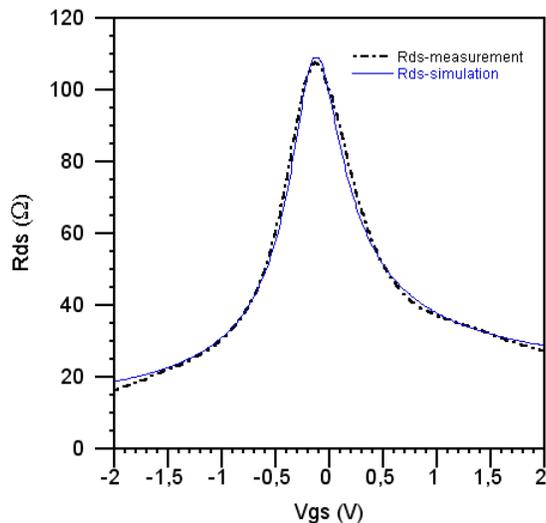
Figure 4.12: Measured and simulated  $R_{ds}$  versus gate bias voltage obtained at  $V_{ds} = 0.1$  V.
