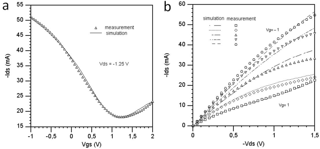
Figure 3.13: a) Transfer function at  $V_{ds} = -1.25$  V, b) output characteristics at  $V_{gs} = 1$  V (top) to  $V_{gs} = -1$  V (bottom),  $L_g = 1 \mu m$   $W_g = 60 \mu m$ .
