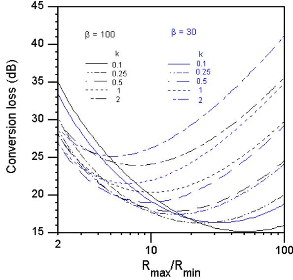
Figure 4.8: CL versus  $R_{max}/R_{min}$  for fixed  $k = R_{min}/Z_0$  for  $\beta = 30$  and 100. All mixing terms generated in the mixer are terminated with the same impedance,  $Z_0$ .
