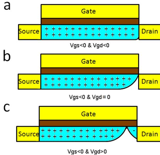
Figure 3.9: a) p-type channel b) channel pinch-off c) bipolar channel.
