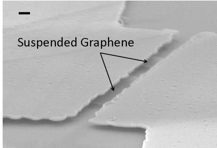
Figure 2.5: A SEM image of a suspended graphene film, scale bar  $1 \mu m$  [62].
