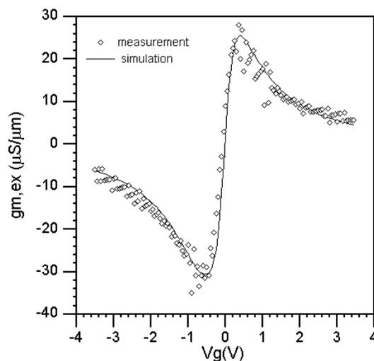
Figure 4.20: A typical G-FET transconductance  $V_{DS} = 0.1$  V [paper A].
