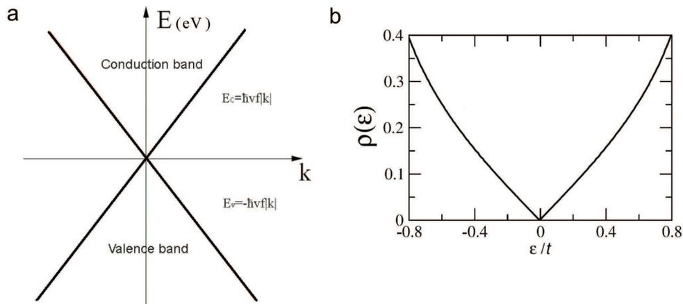
Figure 2.3: a) Energy dispersion model, b) Density of states versus energy [49].
