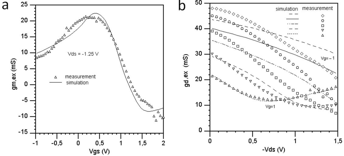
Figure 3.14: a) Device transconductance, b) output conductance.
