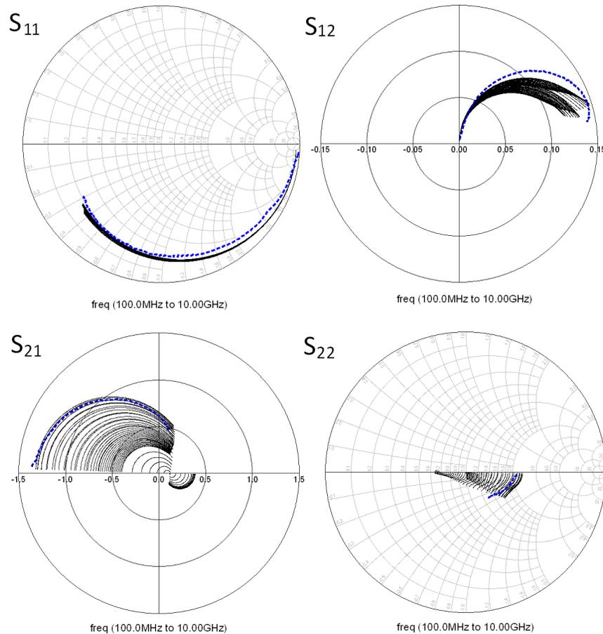
Figure 4.3: Simulated S-parameters versus gate voltage  $\in [-1 \text{ V}, 2 \text{ V}]$  and measured values (dotted line) at  $V_{gs} = 0.3 \text{ V}$  for  $V_{ds} = -1.25 \text{ V}$ .
