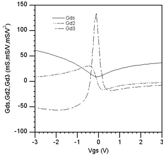
Figure 4.18: Simulated  $G_{ds}$ ,  $G_{d2}$  and  $G_{d3}$  versus  $V_{gs}$  at  $V_{ds} \approx 0$ .
