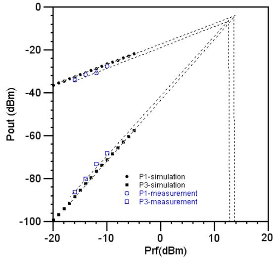
Figure 4.17: Measured and modelled linear and third order response.  $P_{LO} = 15$  dBm.
