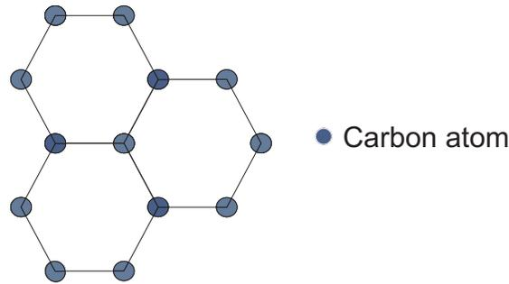
Figure 2.1: Graphene lattice structure.
