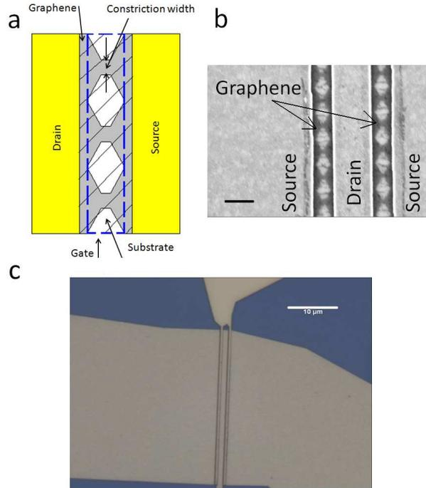
Figure 4.11: a) A schematic of the G-FET with the nanoconstriction channels. The hatched lines indicate the gate dielectric and the dashed line is the gate area. NB! Figure is not to scale. b) SEM image of graphene nanoconstrictions in the G-FET channel before gate-dielectric deposition, scale bar  $1 \mu\text{m}$ . c) Complete G-FET, scale bar  $10 \mu\text{m}$ .
