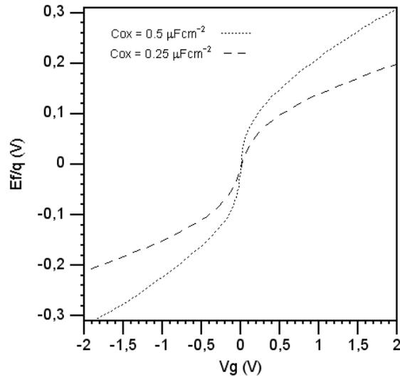
Figure 3.3:  $E_f/q$  versus gate voltage for an ideal metal-oxide-graphene contact with  $C_{ox} = 0.25$  and  $0.5 \mu F cm^{-2}$ .
