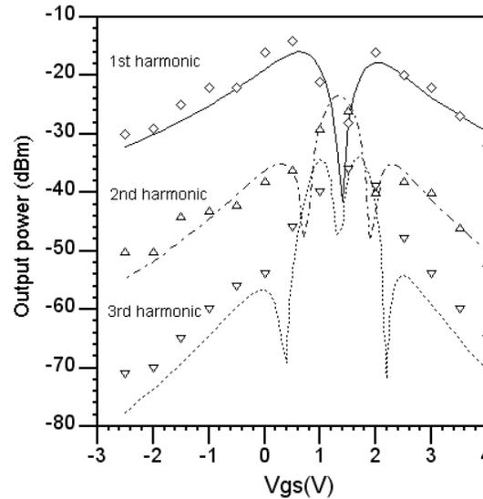
Figure 4.21: Measured and modelled power spectrum,  $P_{in} = 0$  dBm,  $V_{ds} = 0.5$  V [paper A].
