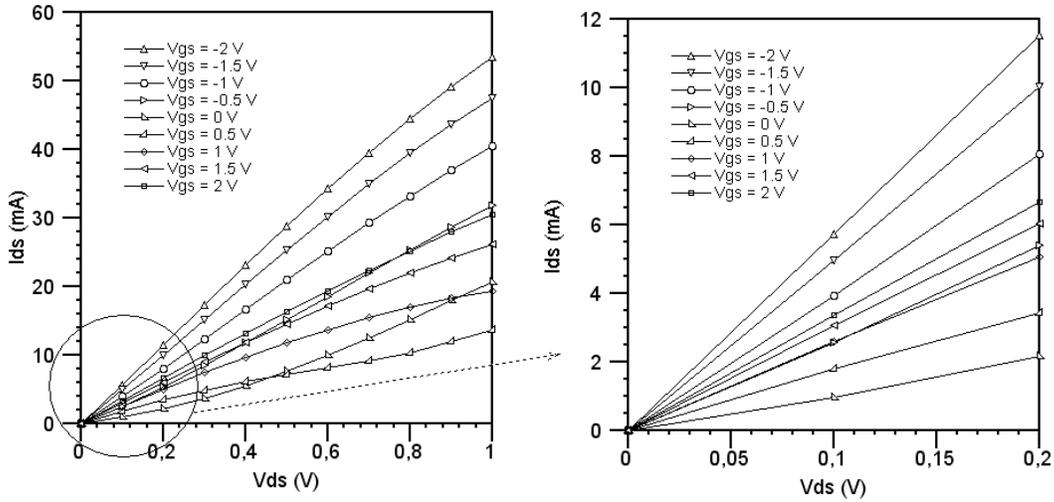
Figure 4.16: Measured DC output characteristics of the G-FET at different gate bias voltages where the linear transport region is identified.
