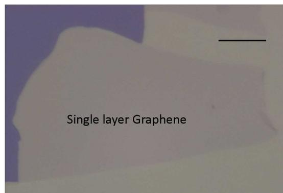
Figure 3.10: A single layer graphene on  $SiO_2/Si$ , scale bar  $10 \mu m$  .
