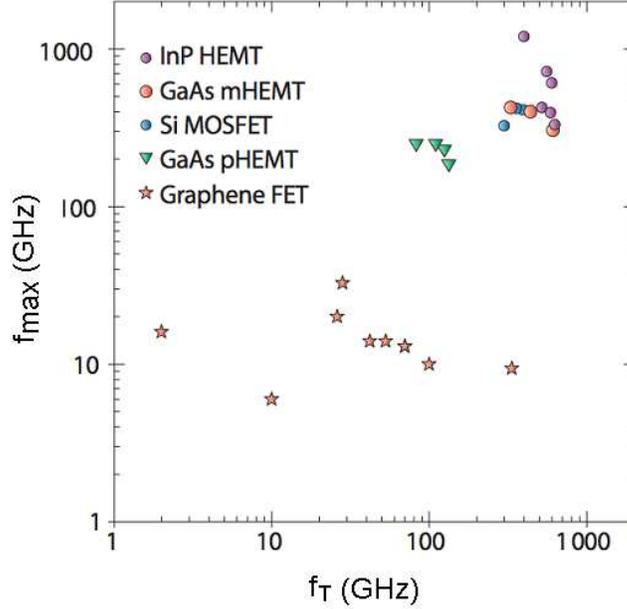
Figure 1.1: Intrinsic performance of the demonstrated G-FETs, where both  $f_{MAX}$  and  $f_T$  are available, versus mature CMOS and HEMT technologies [35].
