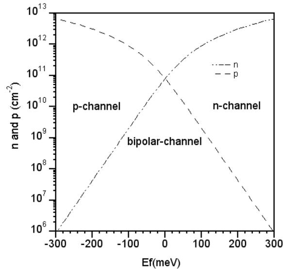
Figure 2.4: Electron concentration ( $n$ ) and hole concentration ( $p$ ) versus Fermi level at room temperature.
