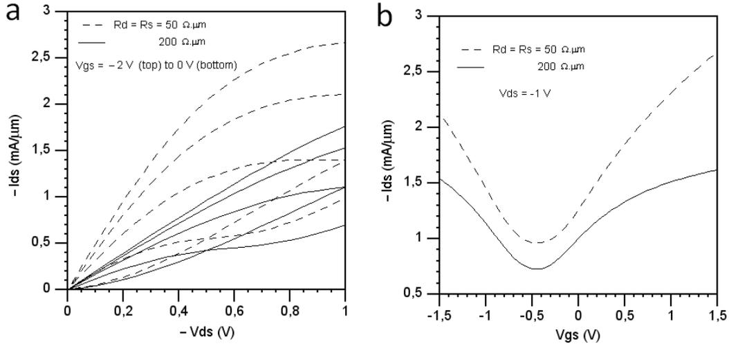
Figure 3.8: a) Simulated  $I_{ds}$ - $V_{ds}$ ,  $V_{gs} = -2$  V (top) to  $V_{gs} = 0$  V (bottom), b) simulated  $I_{ds}$ - $V_{gs}$  at  $V_{ds} = -1$  V, with  $R_d = R_s = 50$  and  $200 \Omega \cdot \mu\text{m}$ ,  $L_g = 0.5 \mu\text{m}$ , and  $\mu = 5,000 \text{ cm}^2/\text{Vs}$ .
