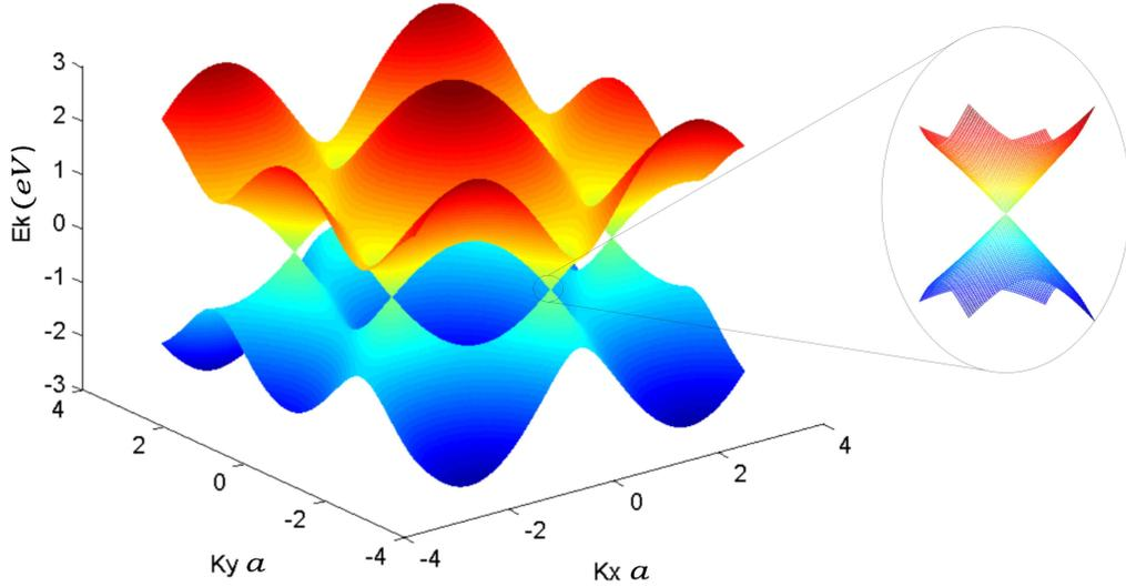
Figure 2.2: Left: Electronic dispersion in the honeycomb lattice, Right: lattice zoom in of the energy bands close to one of the Dirac points.
