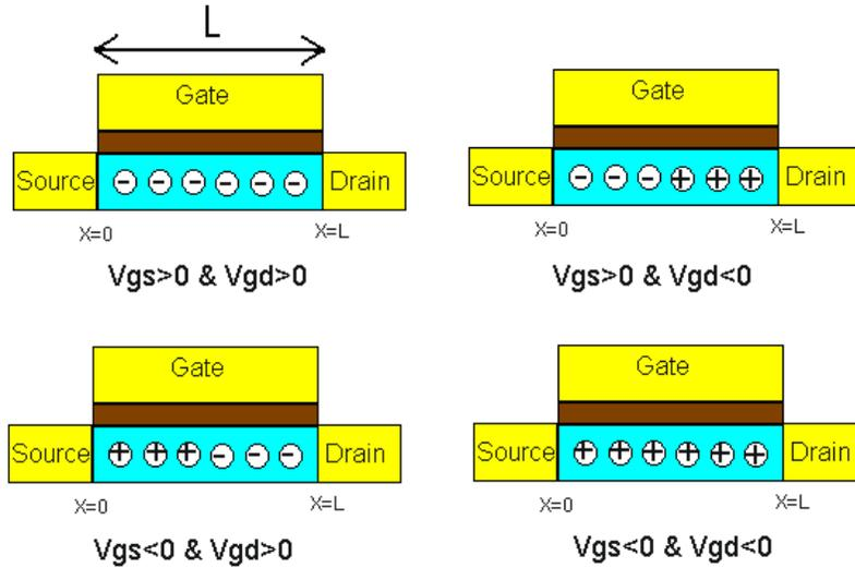
Figure 3.6: Carrier type in a G-FET channel at 4 different quadrants of the  $V_{gs}$ - $V_{gd}$  plane.
