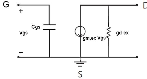
Figure 4.2: A simplified small-signal model of a FET.
