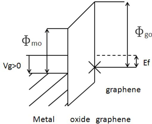
Figure 3.2: Band diagram of a metal-oxide-graphene structure.
