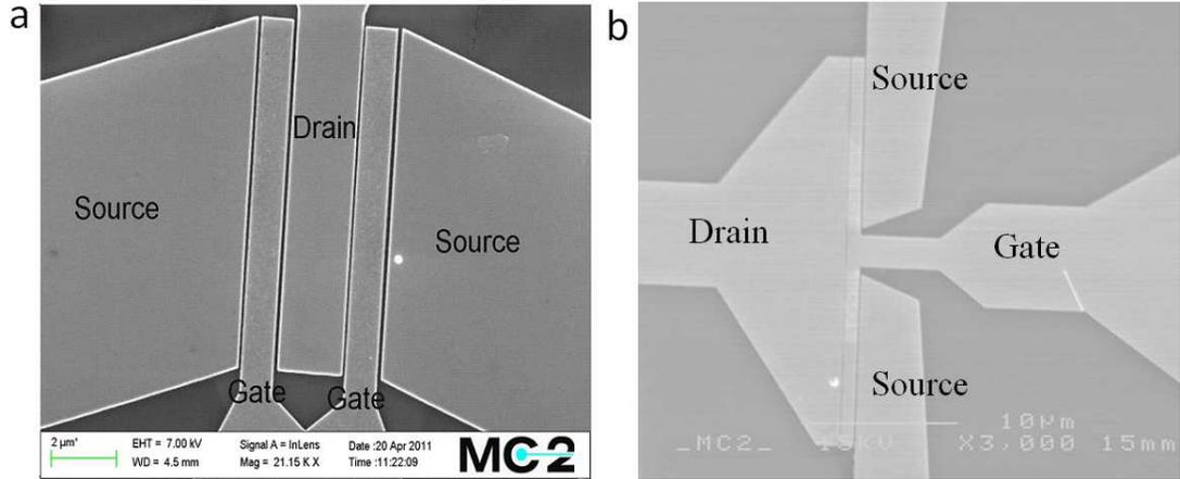
Figure 3.12: a) a G-FET with  $\text{Al}_2\text{O}_3$  gate dielectric  $L_g = 1\ \mu\text{m}$ ,  $W_g = 20\ \mu\text{m}$ , b) a G-FET with silicon nitride gate dielectric,  $L_g = 1\ \mu\text{m}$ ,  $W_g = 15\ \mu\text{m}$ .
