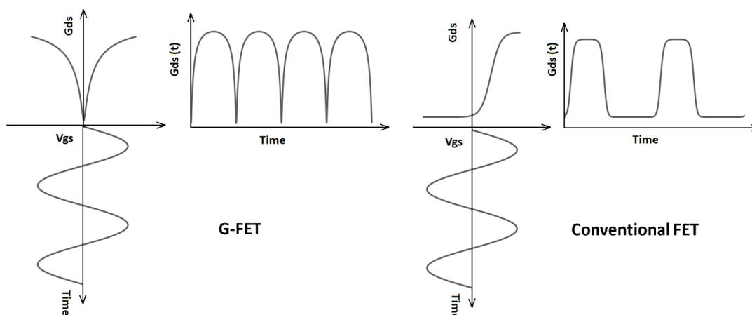
Figure 4.6: The channel conductance and the corresponding conduction wave for a G-FET and a conventional FET.
