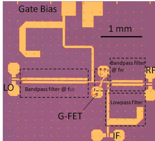
Figure 4.14: Photomicrograph of the fabricated subharmonic mixer on high resistivity silicon substrate. The chip measures  $3.4 \times 3.2 \text{ mm}^2$ .
