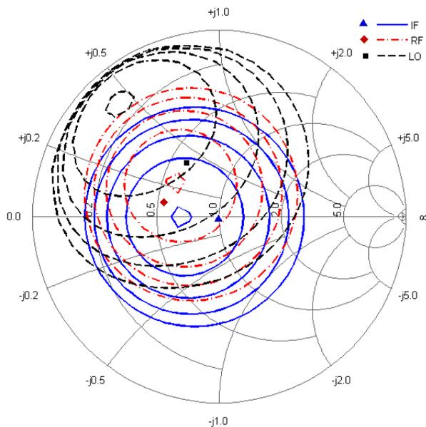
Figure 4.13: Simulated CL contour plots for LO, RF and IF embedding impedances. The inner contour is for  $CL \approx 17$  dB and the outer contour is for  $CL \approx 19$  dB (0.5-dB step),  $P_{LO} = 10$  dBm and all other mixing terms are terminated with  $50 \Omega$ . The RF, LO and IF selected embedding impedances for the designed circuit are also depicted.
