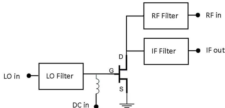
Figure 4.5: General topology for a down-converting single-ended resistive FET mixer.
