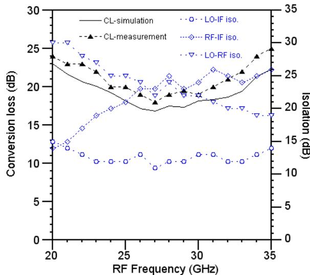
Figure 4.15: Conversion loss and port isolations versus frequency at 10 dBm LO-power with  $f_{IF} = 100 \text{ MHz}$ ,  $f_{LO} = (f_{RF} - f_{IF})/2$ .
