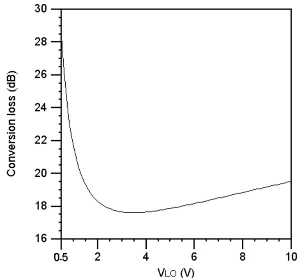
Figure 4.9: CL versus gate  $V_{LO}$  for  $\beta_0 = 5 \text{ V}^{-2}$ ,  $R_{max}/R_{min} = 10$  and  $k = R_{min}/Z_0 = 0.5$ . All mixing terms generated in the mixer are terminated with the same impedance,  $Z_0$ .
