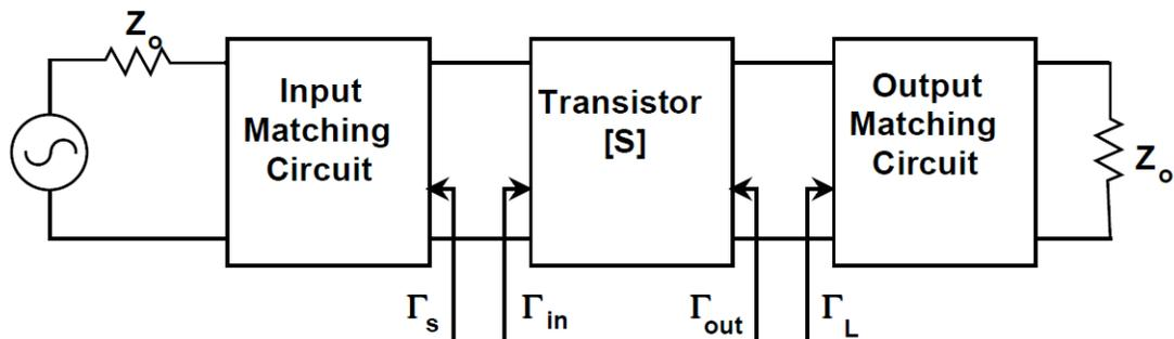
Figure 4.1: A single-stage microwave transistor amplifier diagram.
