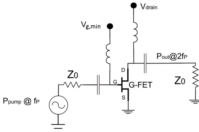
Figure 4.22: Circuit structure of a G-FET frequency doubler.
