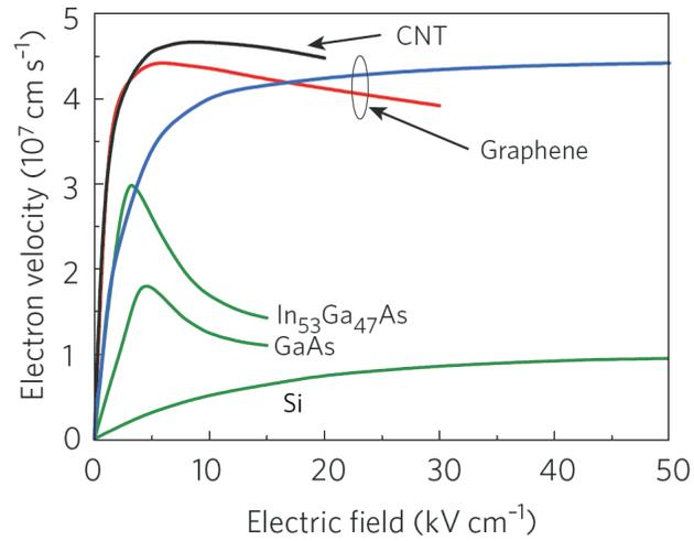
Figure 2.6: Electron drift velocity versus electric field [32].
