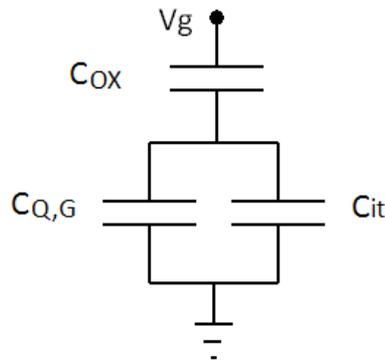
Figure 3.4: The metal-oxide-graphene capacitive network.
