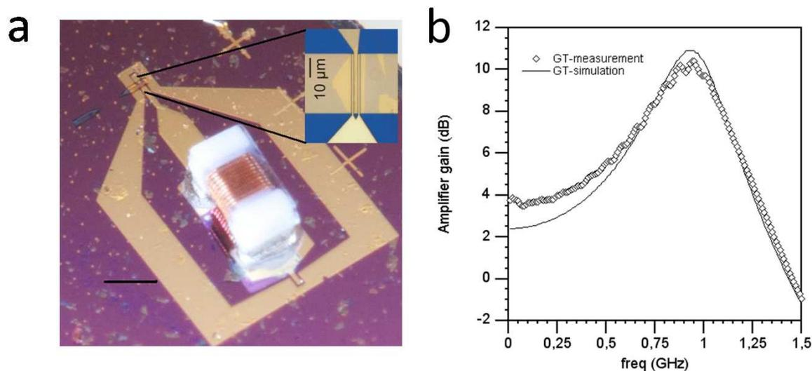
Figure 4.4: a) G-FET amplifier, b) Amplifier gain at  $V_{gs} = 0.3$  V,  $V_{ds} = -1.25$  V
