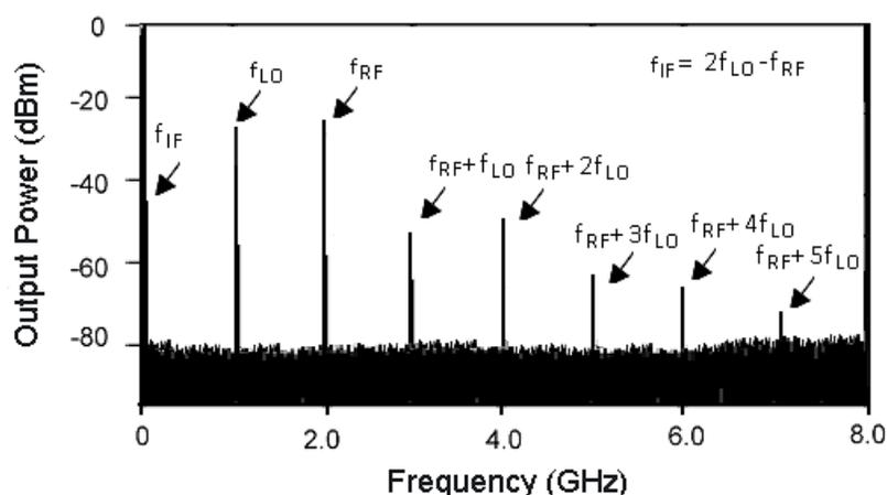
Figure 4.10: Spectrum of the reflected signal,  $V^-(t)$  and the LO leakage ( $P_{LO} = 15$  dBm,  $P_{RF} = -20$  dBm,  $f_{RF} = 2$  GHz,  $f_{LO} = 1.01$  GHz).
