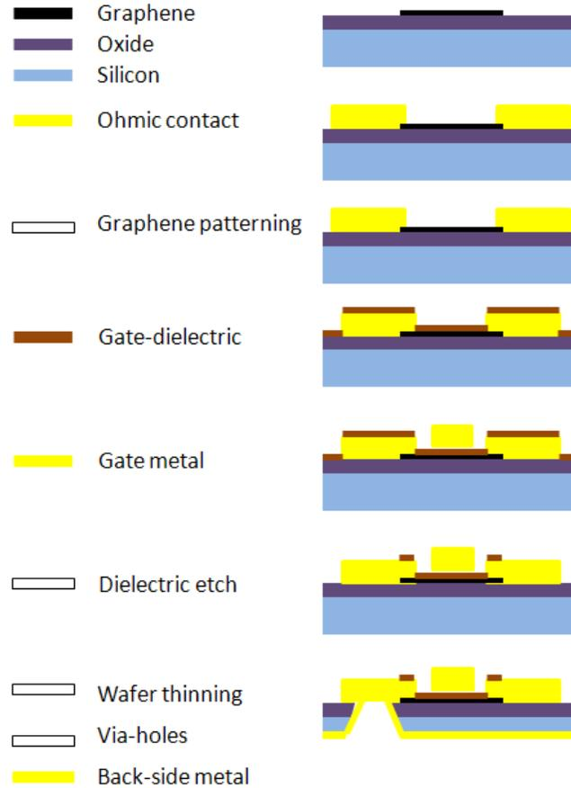
Figure 3.11: Fabrication process sequence.
