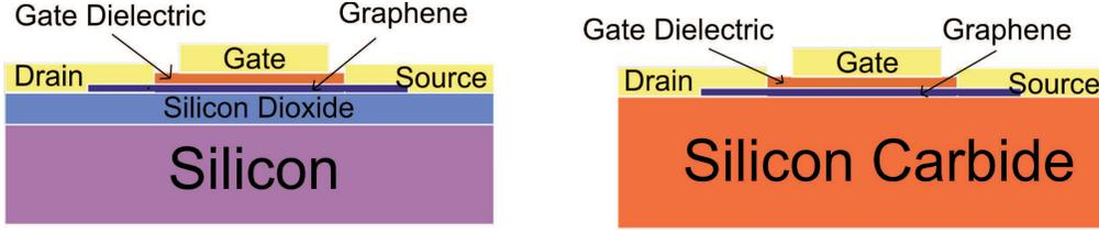
Figure 3.1: The layer structure of G-FETs based on, transferred graphene (left), and sublimation of SiC (right).
