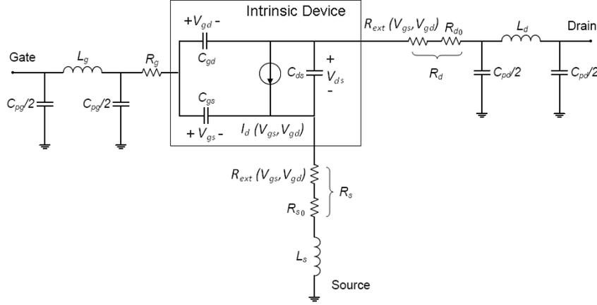
Figure 3.7: Equivalent circuit of a G-FET device.
