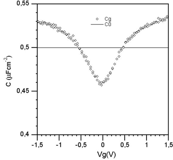
Figure 3.5: Measured CV for a metal-oxide-graphene capacitive network with 8 nm  $Al_2O_3$  gate dielectric.
