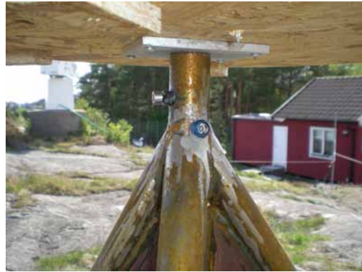
(b) Prism mounting at the top of the mast
