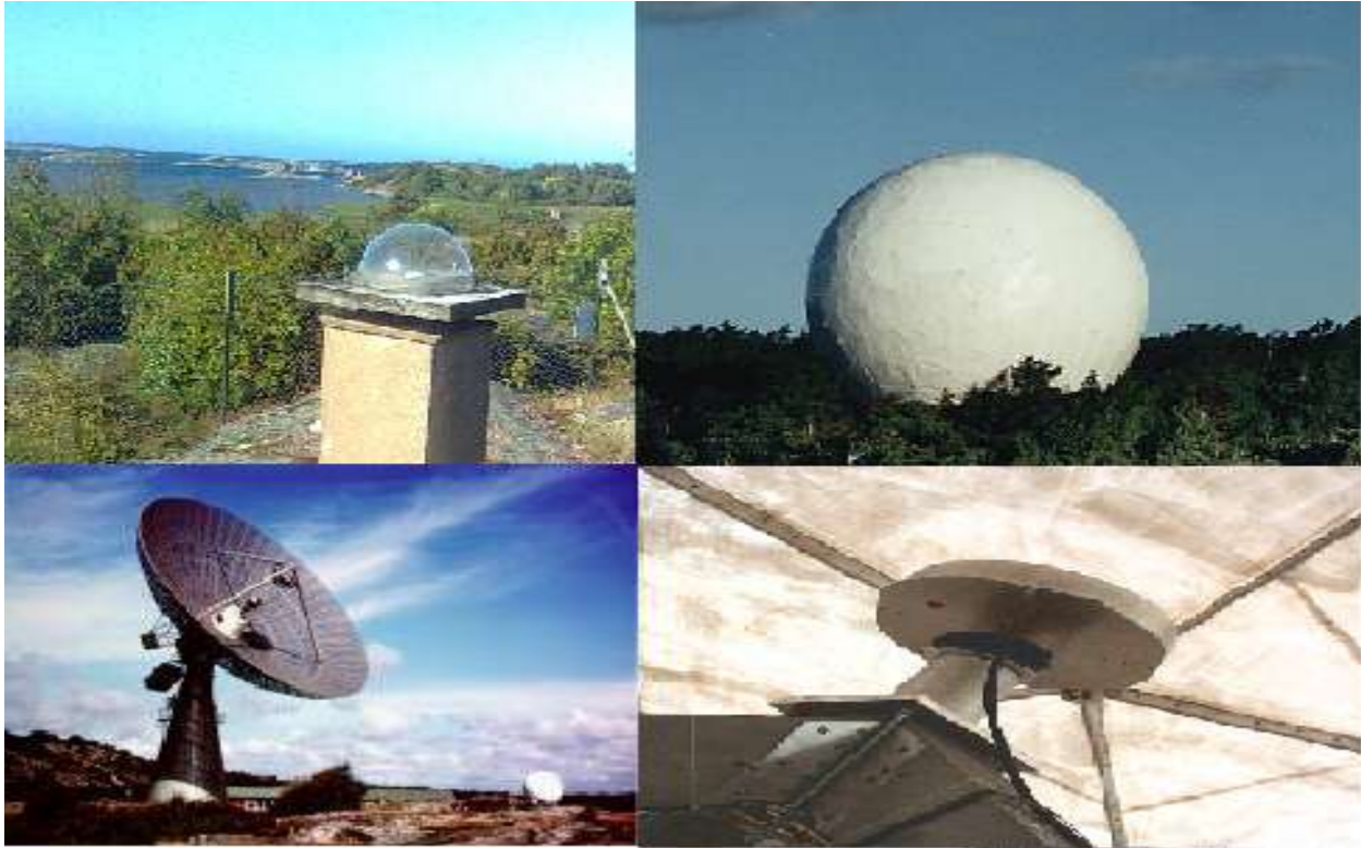
Figure 1.1: The IGS station (top-left), the radome enclosed 20 meter radio telescope (top-right), the 25 meter radio telescope (bottom-left), the GNSS antenna on top of the 20 meter radio telescope (bottom- right)
