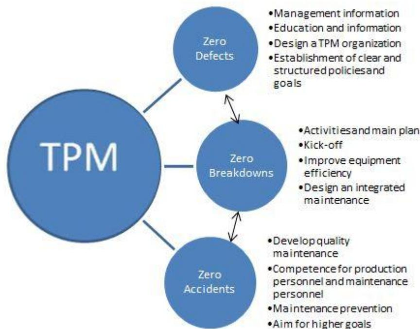
Figure 16. TPM consists of three basic goals; Zero product defects, Zero breakdowns and Zero Accidents. Furthermore TPM have 12 activities coupled to the basic goals.
