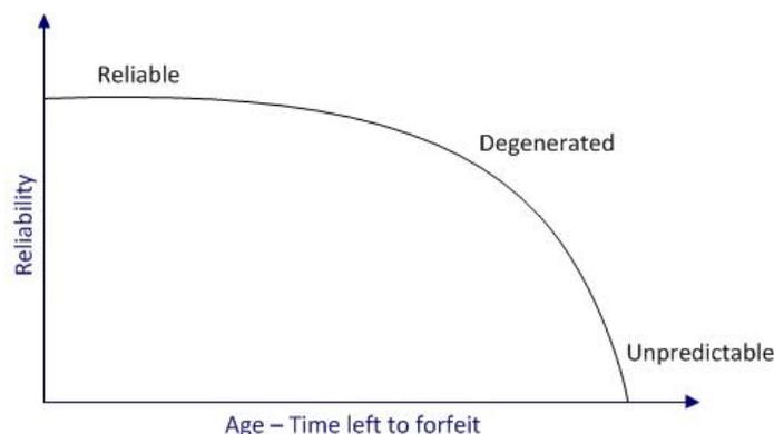
**Figure 23. With increased age the reliability will be decreased, and finally the asset will have passed the three phases, reliable, degenerated and unpredictable.**
