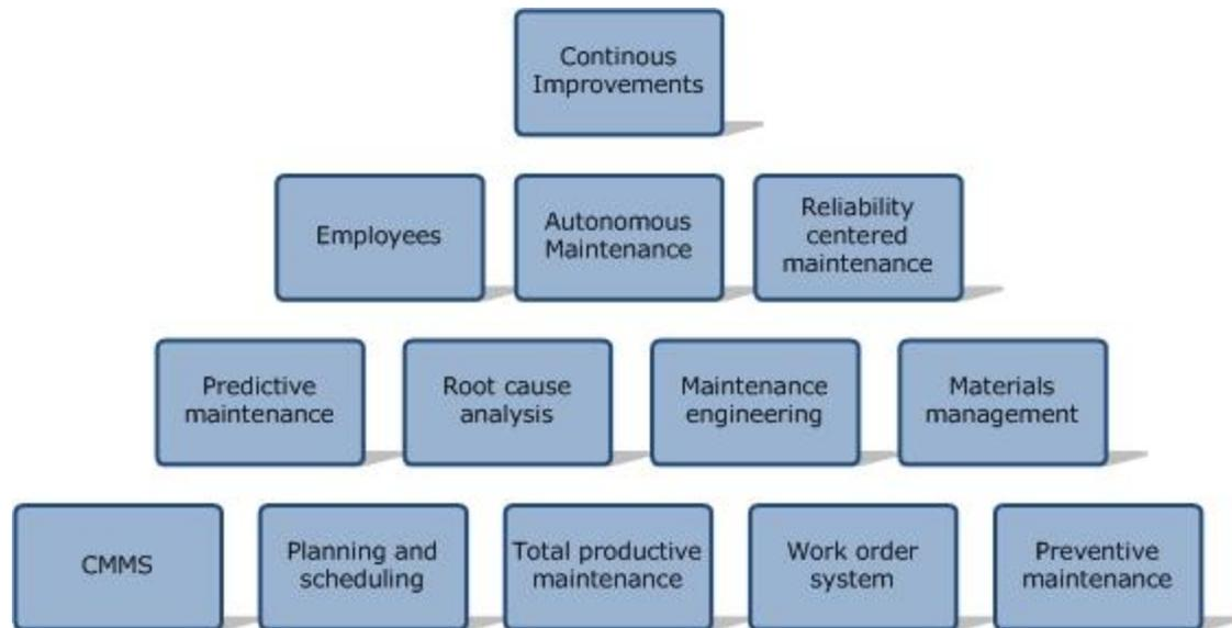
Figure 19. Maintenance management pyramid, according to Smith (2004). Each internal part makes up the concept of lean maintenance.
