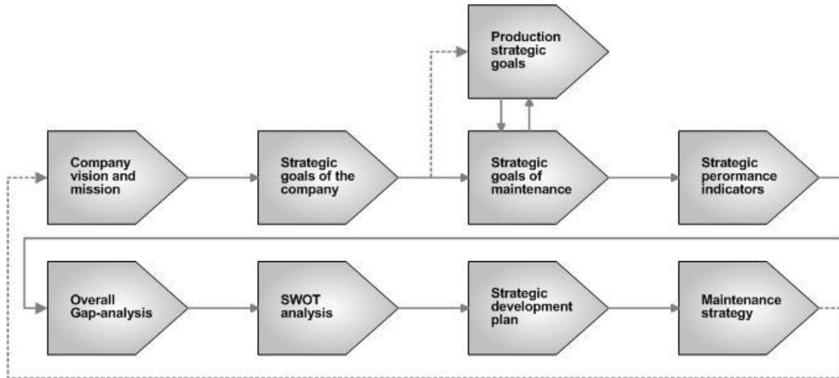
Figure 5. A schematic view of the work-process when formulating a maintenance strategy (Salonen, 2009)
