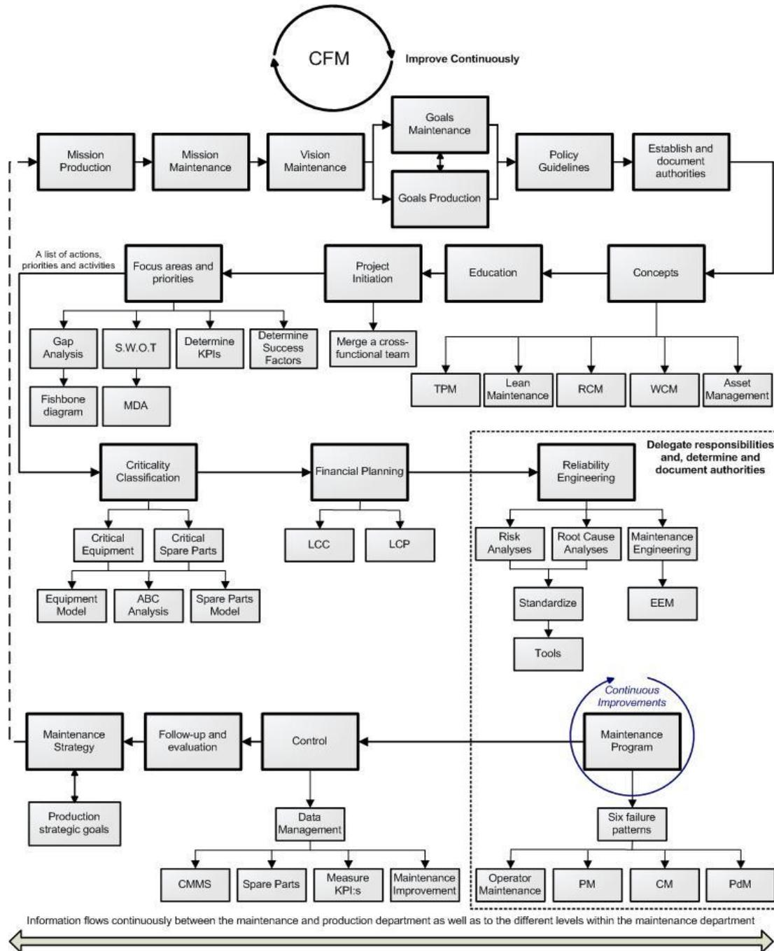
Figure 44. A Customer Focused Model for the formulation of a maintenance strategy.
