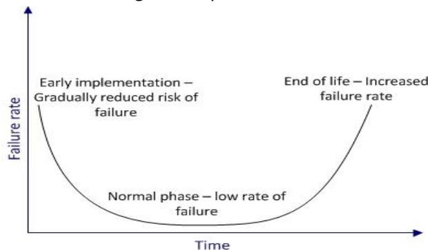
Figure 26. Life cycle cost for an asset. Higher level of failures discloses itself in early implementation phases and in the end of the assets life.
