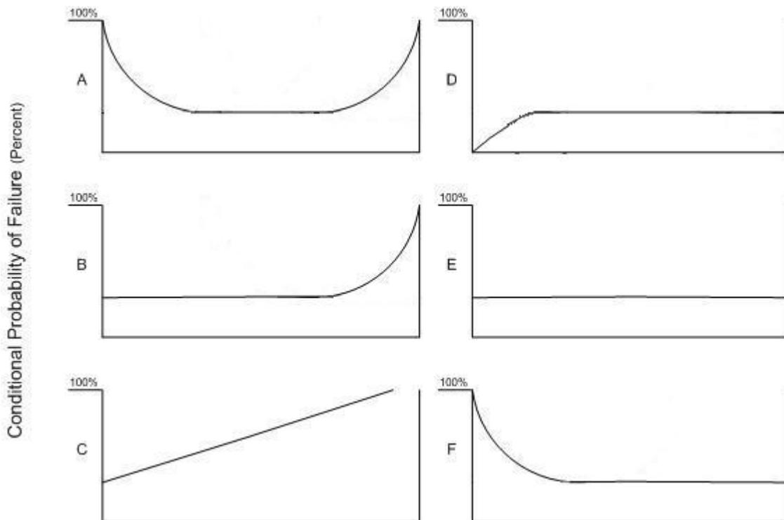
**Figure 20. RCM Failure Patterns – The six failure patterns included in RCM methodology, each curve is plotted as probability of failure against age (Moubray, 1997; NASA, 2008).**
