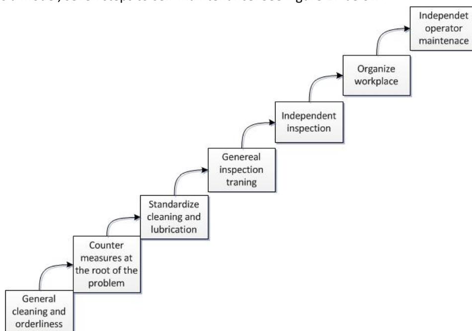
Figure 17. Reaching independent operator maintenance is based on starting with simple tasks and develops as the operator raises the level of competence (Nord, C., Pettersson, B., Johansson, B., 1997)
