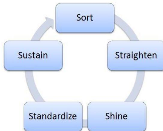
Figure 18. The process-chain for 5S is intended to continue to run continuously and have hence no apparent end. (Liker, J.K, 2004) (pp. 151, Figure-13-1)
