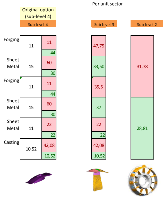
Figure 61 First Application: Example 2- cost & producibility number until whole TEC assembly level
