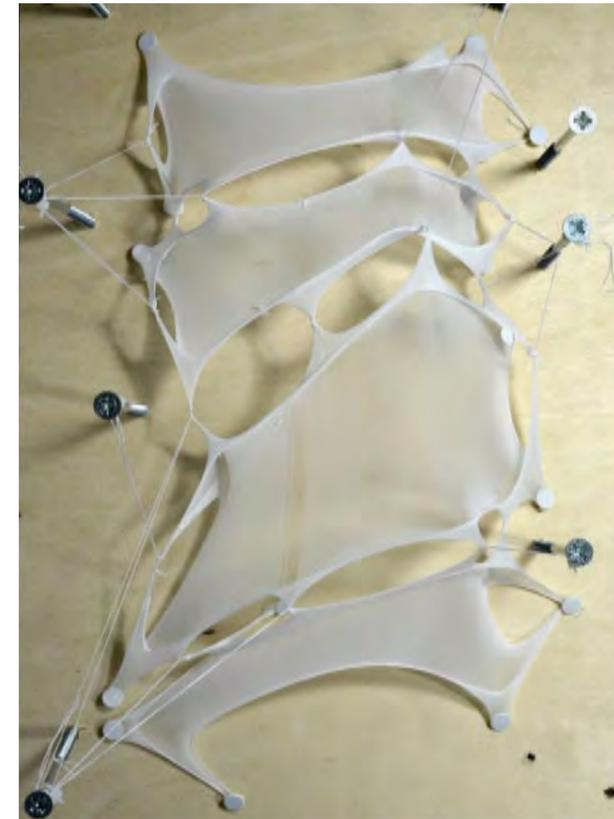
Fig. 42, fabric model made with 15 den stocking, stretched with strings
