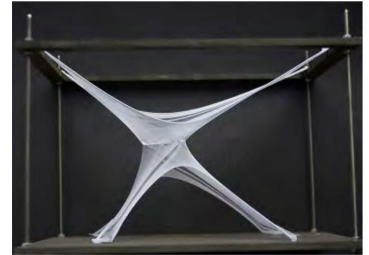
2 surfaces with 1 intersecting constraint and controlled ripping
