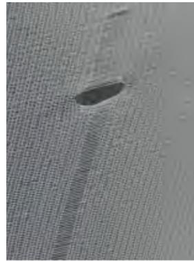
Fig. 38, The direction punctures spreads along the fabric. Density 15 denier
