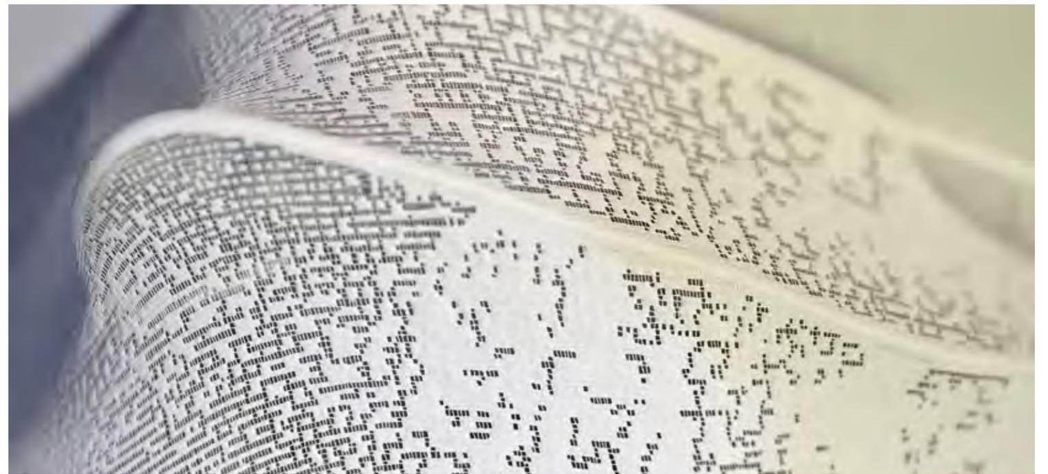
One hardened surface with controlled ripping, broad point constraints, 3 4 point knots and internal predetermined geometric constraints. The hardening process (achieved through a spray filler) creates a pixelated texture as a result of the fabric's weave.
