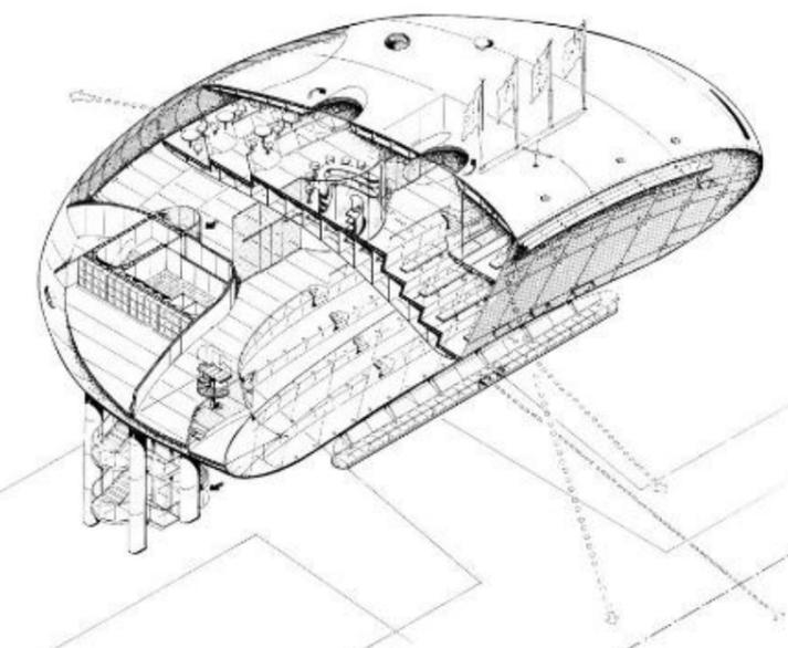
Fig. 26, Natwest Media Centre, Lord's Cricket Ground, by Future Systems is a semi-monocoque construction
