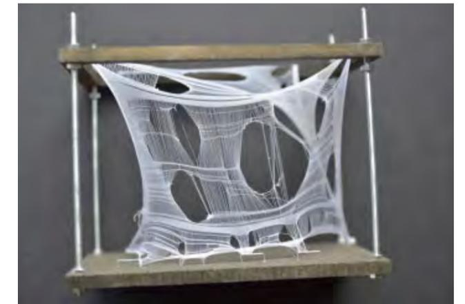
Various point constraints on the XY plane and 1 upper point constraint
