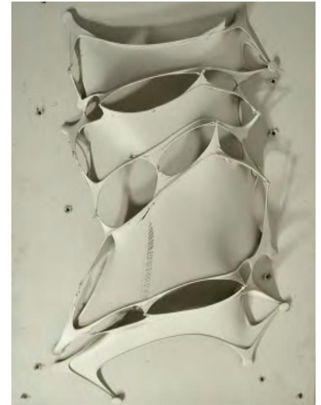
Fig. 43, stiffened fabric with a type of plaster spray. The strings are removed and the model supports itself
