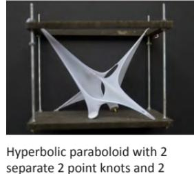
Hyperbolic paraboloid with 2 separate 2 point knots and 2 broad point constraints on the XY plane
