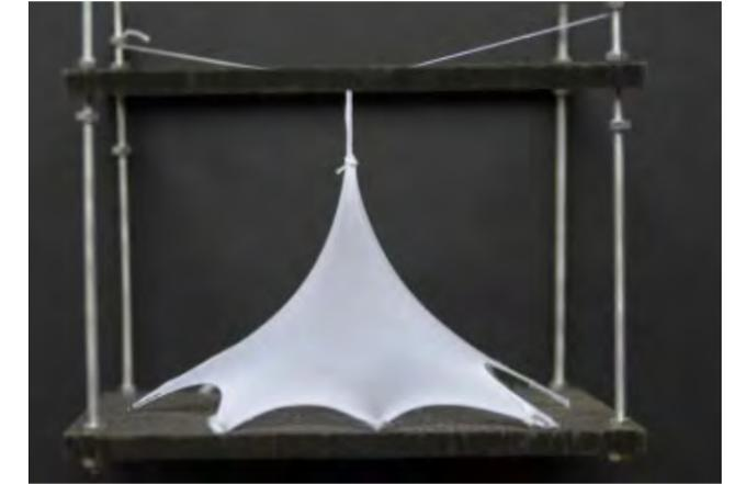
4 planar and 1 broad point constraint on 2 XY planes
