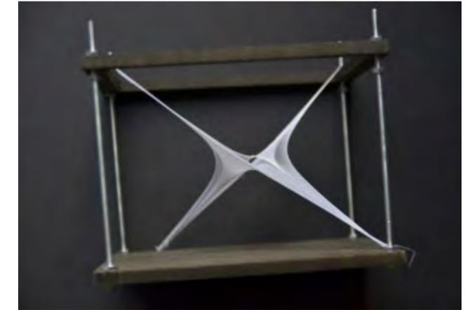
Hyperbolic paraboloid with 2 separate 2 point knots
