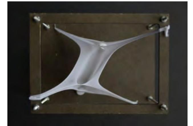
Hyperbolic paraboloid with a 4 point knot
