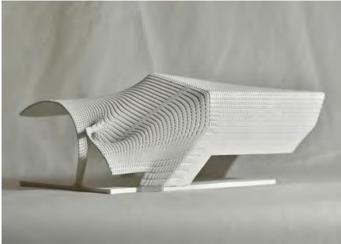
3D print of a section of the final design. Using a plug-in to Autodesk's Maya called Ncloth, which is a digital simulation of fabric, a polygon surface was produced. This surface was then further subdivided into smaller quadrilaterals whose faces have been individually manipulated to create the texture.
