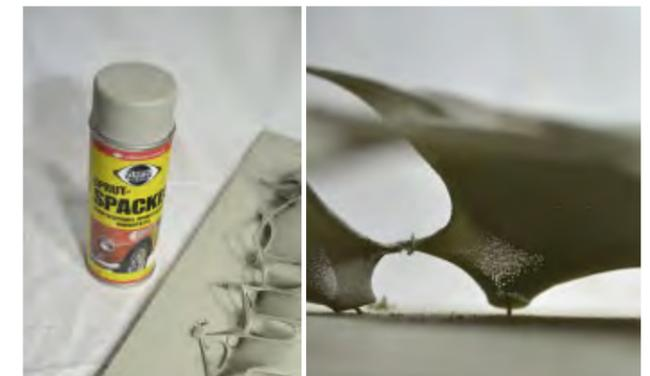
Fig. 47, Plaster spray. The weave in the fabric leaves holes that lets light through
