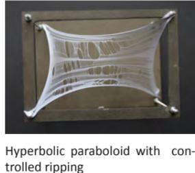
Hyperbolic paraboloid with controlled ripping
