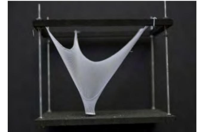
Mirrored scherk-like surfaces with intersecting constraints
