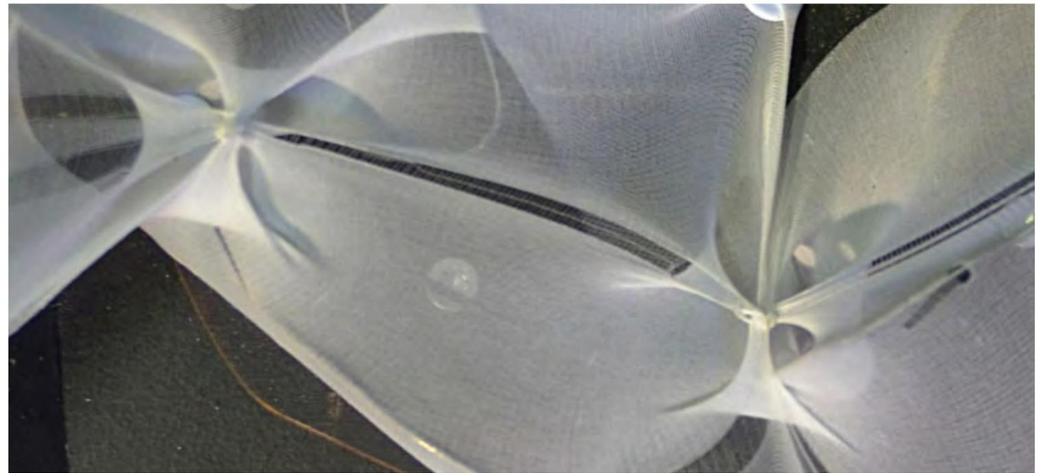
One surface with controlled ripping, broad point constraints, 3 and 4 point knots and internal predetermined geometric constraints
