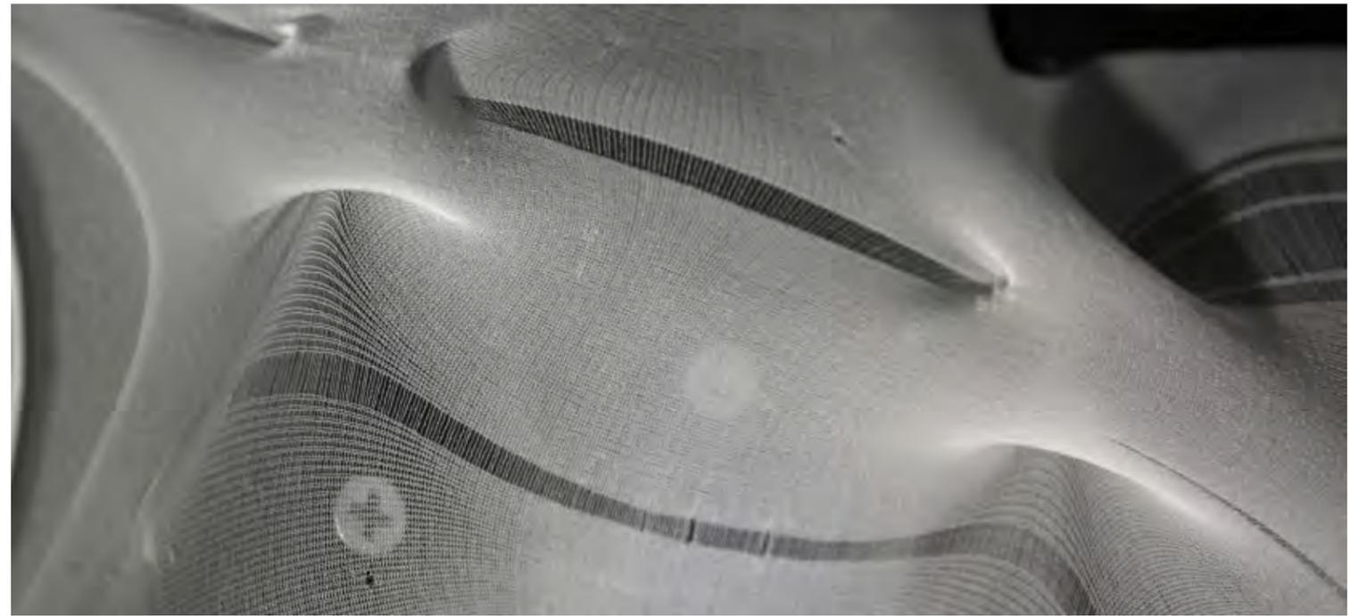
One surface with controlled ripping, broad point constraints, reverse point knots and internal predetermined geometric constraints
