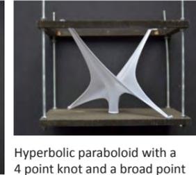
Hyperbolic paraboloid with a 4 point knot and a broad point constraint on the XY plane
