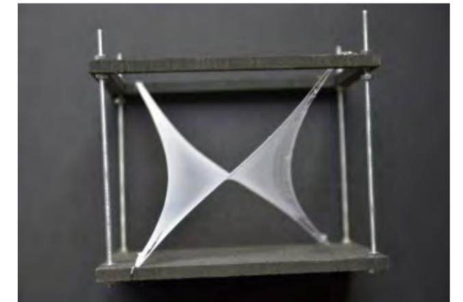
Hyperbolic paraboloid with controlled ripping 2
