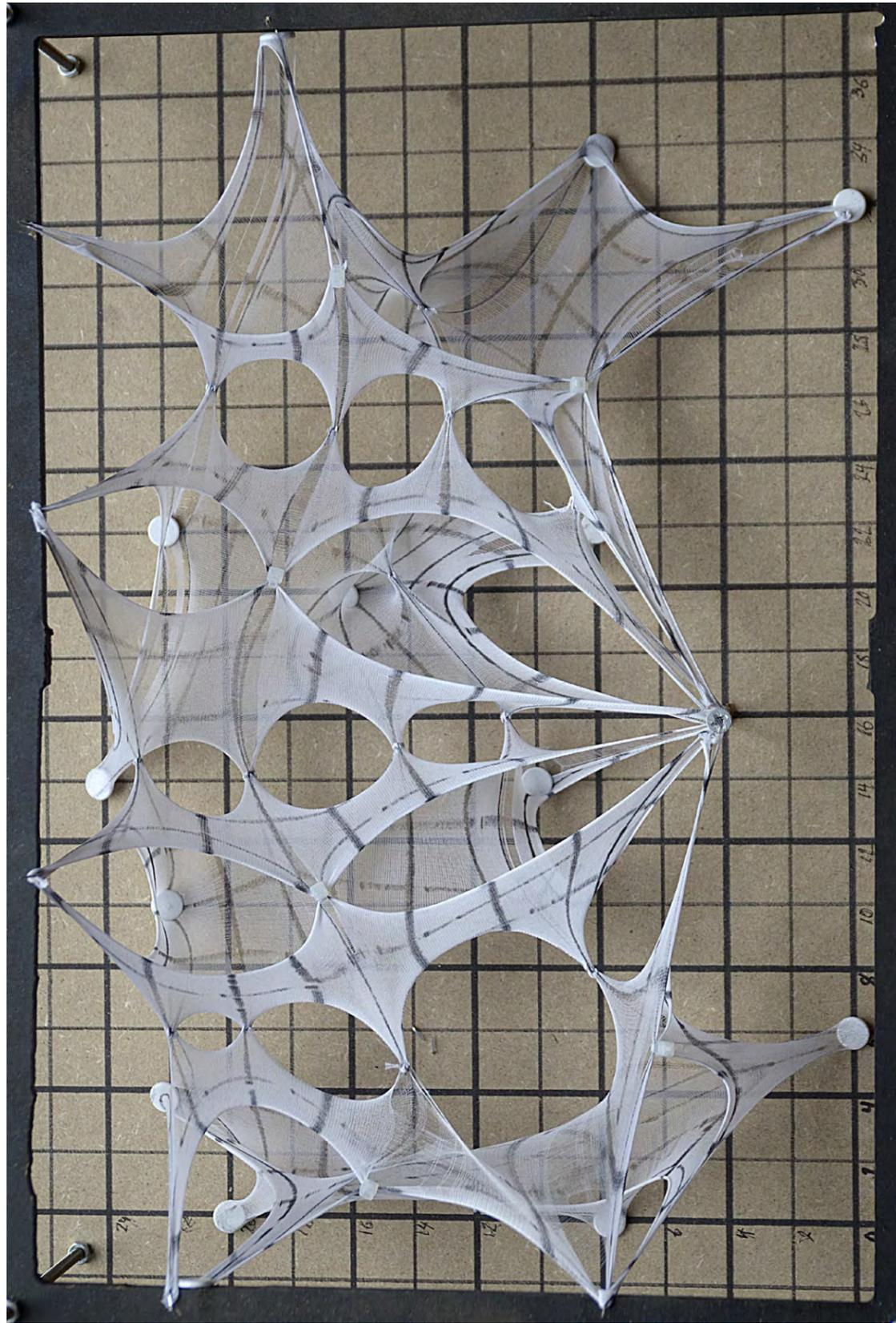
Multiple surfaces with intersecting point constraints. A grid was marked out onto the fabric prior to the model making in order to analyse directional behaviours in the fabric.
