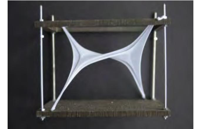
Hyperbolic paraboloid with 2 separate 2 point knots and 2 broad point constraints on the XY plane
