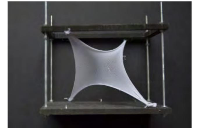
Hyperbolic paraboloid with a 2 point knot
