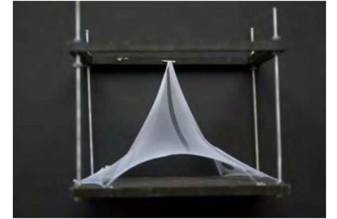
Canal surface with 8 point constraints on the XY plane and 1 upper point constraint
