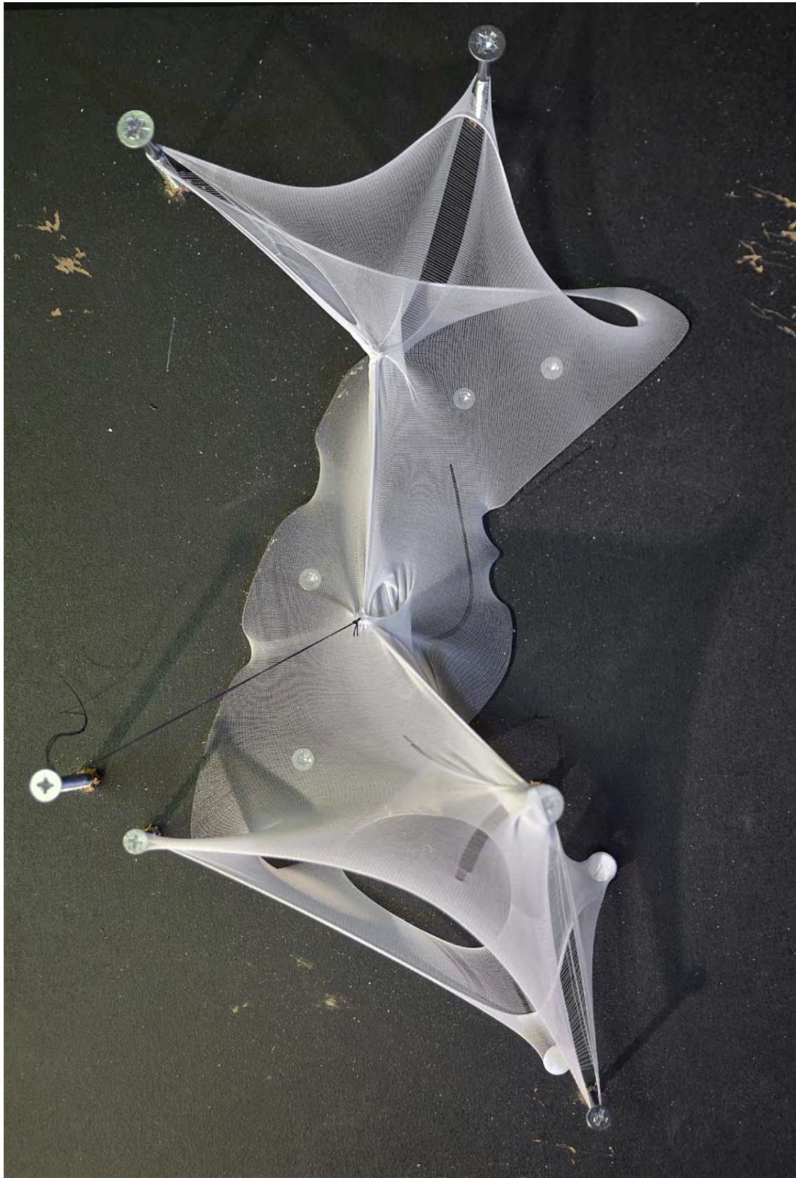
One surface with broad point constraints, various point knots and internal predetermined geometric constraints
