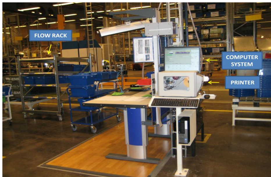
Figure 21: Startelement station after implementation
