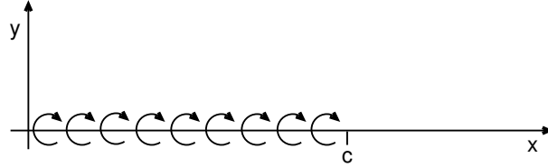
Figure 2.7.2: Vortex distribution along the camber line on the x-axis
