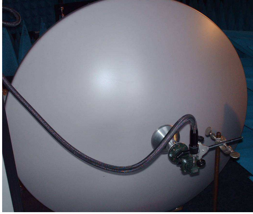
Figure 5.2: Monolayer radome under test. Manufactured by Arkivator AB.
