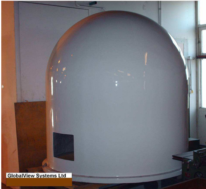
Figure 5.3: Sandwich radome with access hatch for satellite earth station. Manufactured by Art&Technology.
