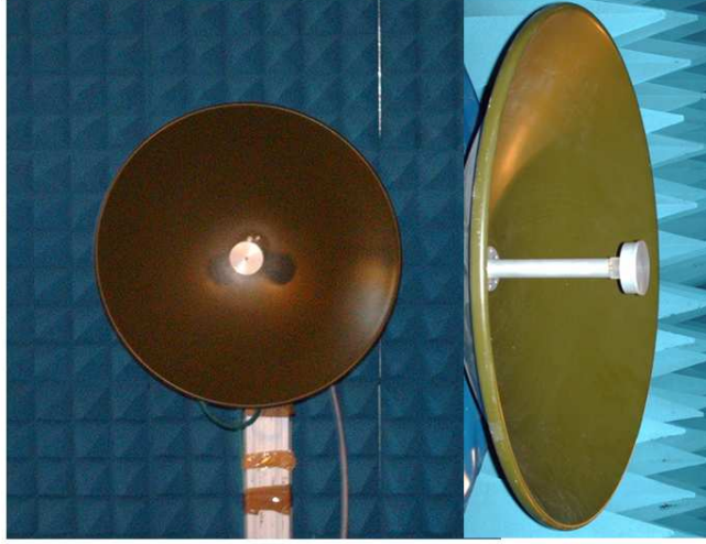
Figure 6.15: Hat-fed reflector antenna under test in anechoic chamber.
