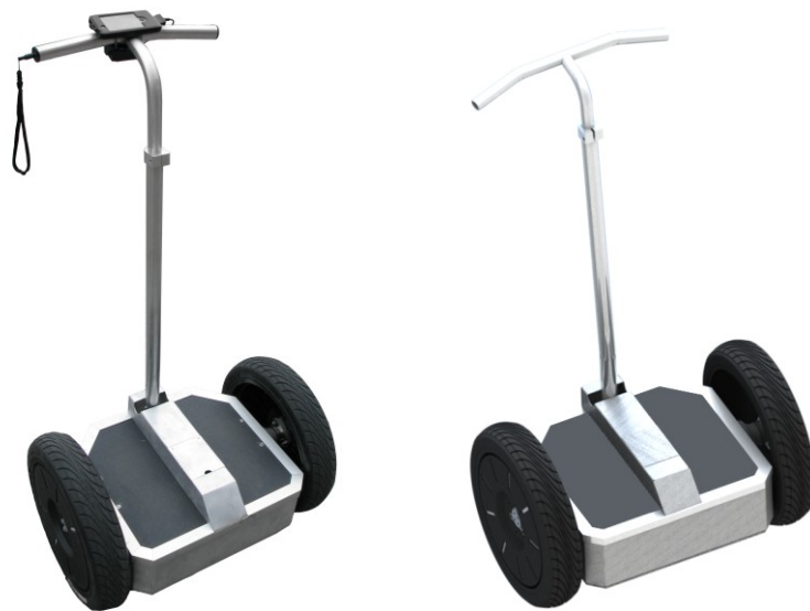
Figure 8 - The vehicle in reality to the left and the CAD-model to the right.
