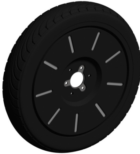
Figure 18 - The selected wheel, a 19" wheel weighing 4,6 kg.
