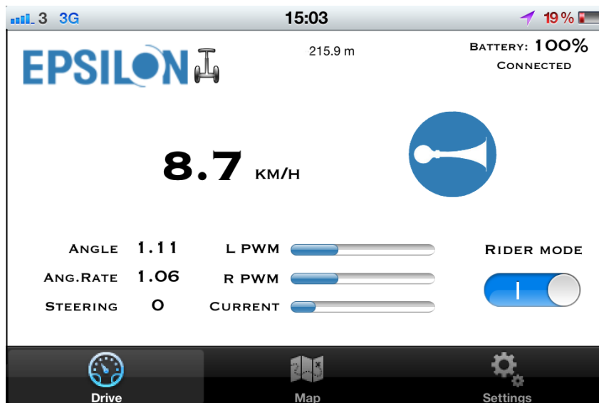
Figure 22 – The drivers tab, which updates every 50 ms with new information from the vehicle. ‘Rider mode’ is a switch that activates the controller.
