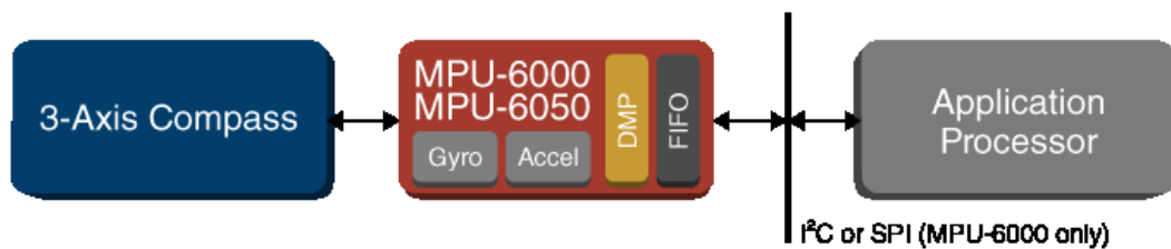
Figure 25 - Diagram over MPU-6050 integration with application processor. The compass is optional (image from www.invensense.com , retrieved 9th May 2012).
