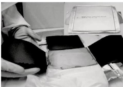
**Figure 4.1.** Inside the battery alternate layers of cathodes, anodes and separator respectively, (inset) a new battery
