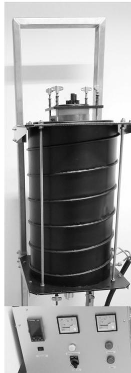
**Figure 4.2.** Vertical tube furnace with controller below
