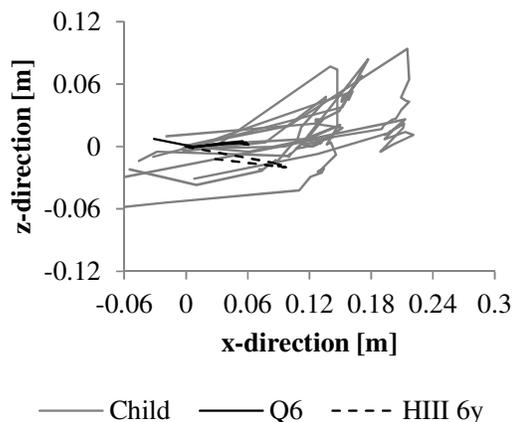
**Figure 6** Trajectories for forehead target for Q6, HIII 6y and children (grey) on highback booster seat.
