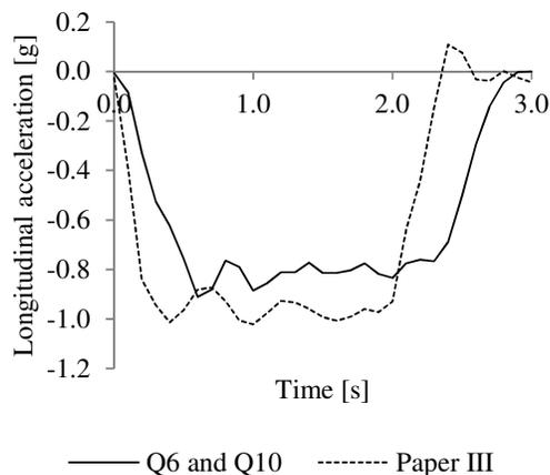
**Figure 5** The average longitudinal acceleration for the two brake manoeuvre test series. Time zero is defined as the point where brake pressure increased drastically.
