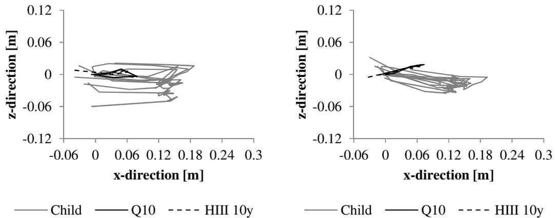
**Figure 9** Trajectories for Q10, HIII 10y and children (grey) restrained by seat belt only. Ear target to the left and forehead target to the right.
