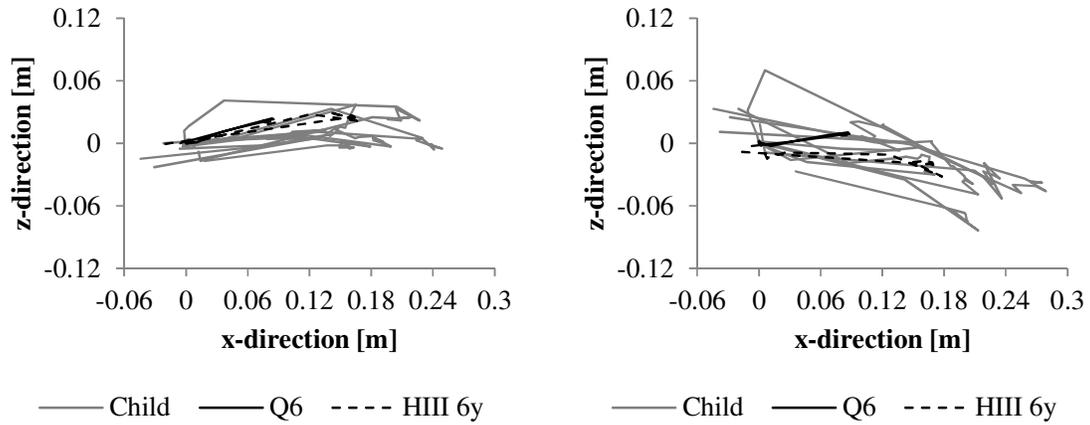
**Figure 7** Trajectories for Q6, HIII 6y and children (grey) on booster cushion. Ear target to the left and forehead target to the right.
