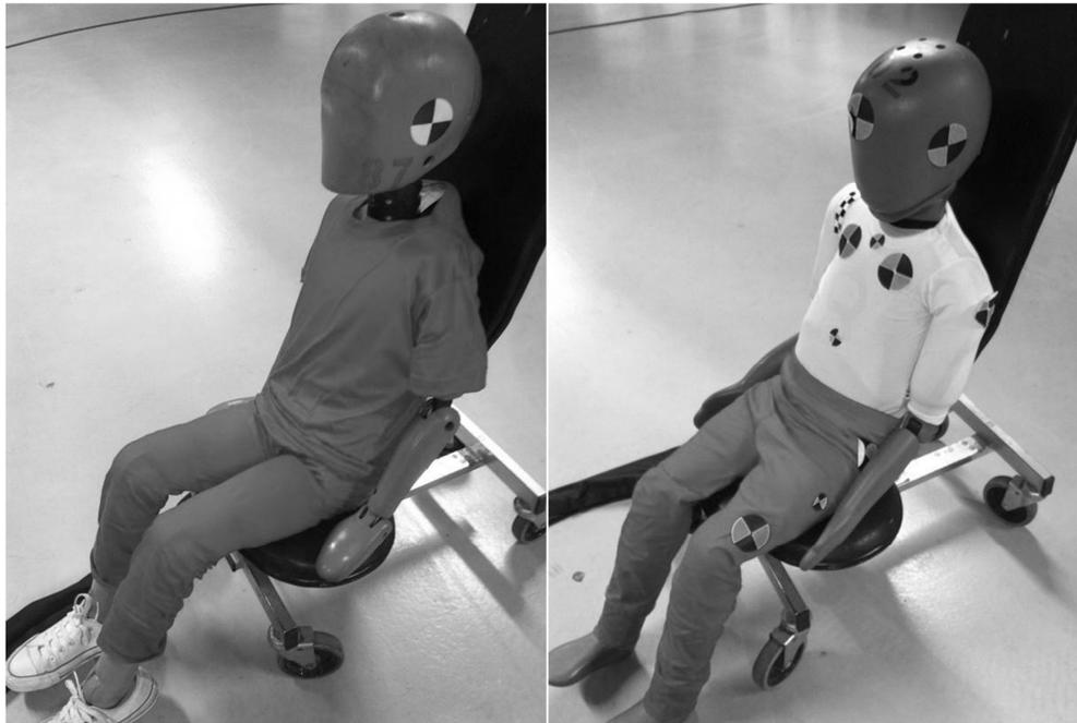
**Figure 4** The Hybrid III 6y ATD, left, and Q6 ATD, right.
