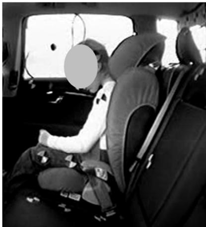
**Figure 12** Maximum forward head position of a child on a highback booster seat during an emergency braking manoeuvre.
