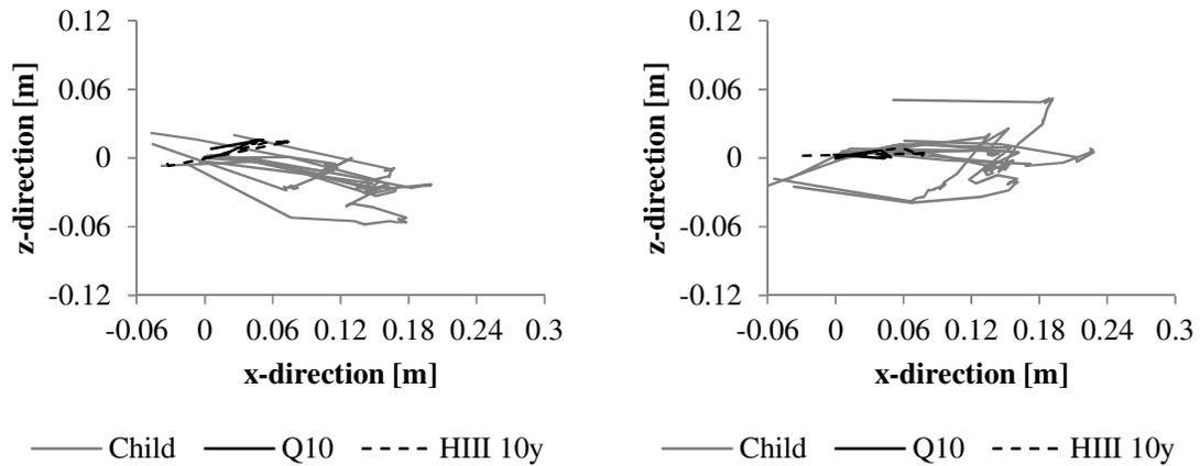
**Figure 8** Trajectories for Q10, HIII 10y and children (grey) on booster cushion. Ear target to the left and forehead target to the right.
