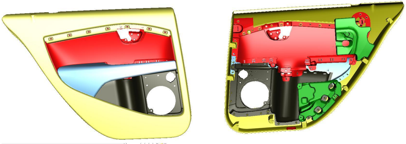
Figure 7 Rear door interior panel and its' main components
