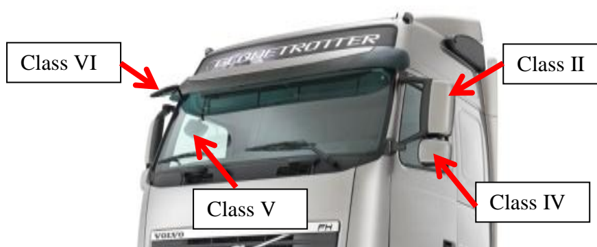
Figure 1: Different mirror types found on a Volvo FH truck (Volvo GTT, 2012)
