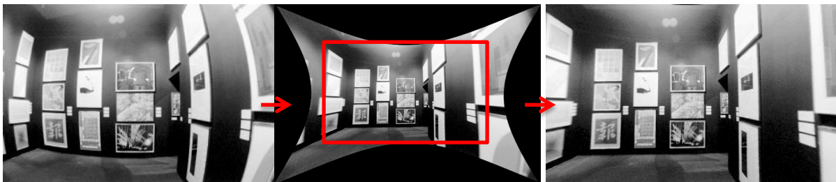
Figure 13 : Barrel distortion and reversed barrel distortion (Becker, 1994)
