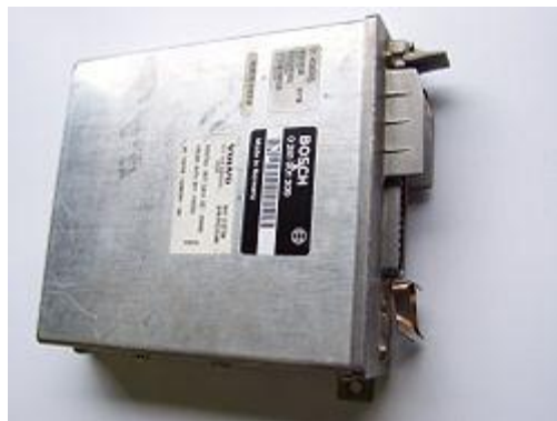
Figure 12: An ECU from BOSCH (Wikipedia, Electronic control unit, 2010)
