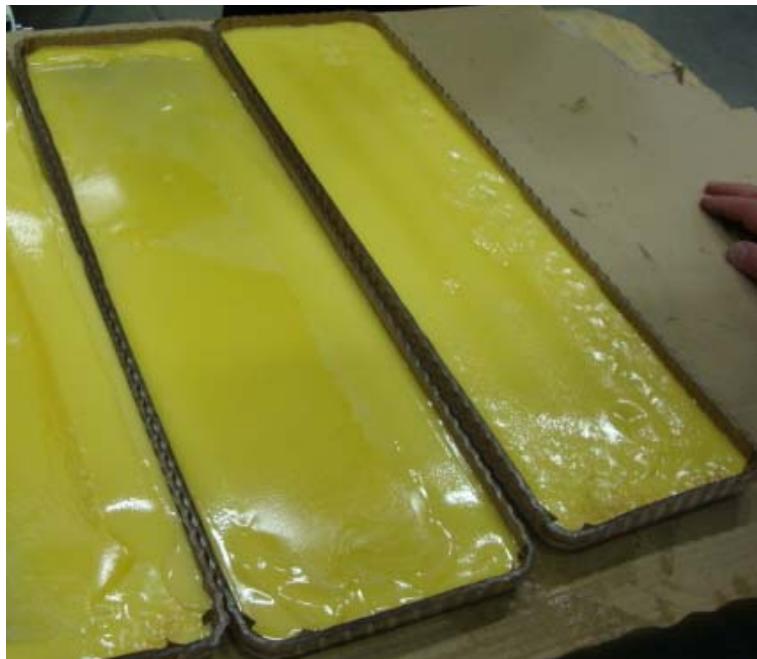
Figure 17: This picture shows BCM tray 1 (right) and BCM tray 2 (left) after the MW heating in Run 5 . The thinner dark yellow stripes in BCM tray 1 show the uncoagulated parts.
