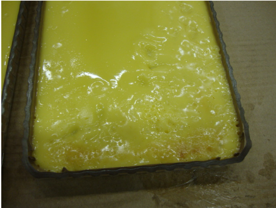
Figure 16: In this picture, the increased porosity due to trapped air bubbles during the BCM heating is visualized.
