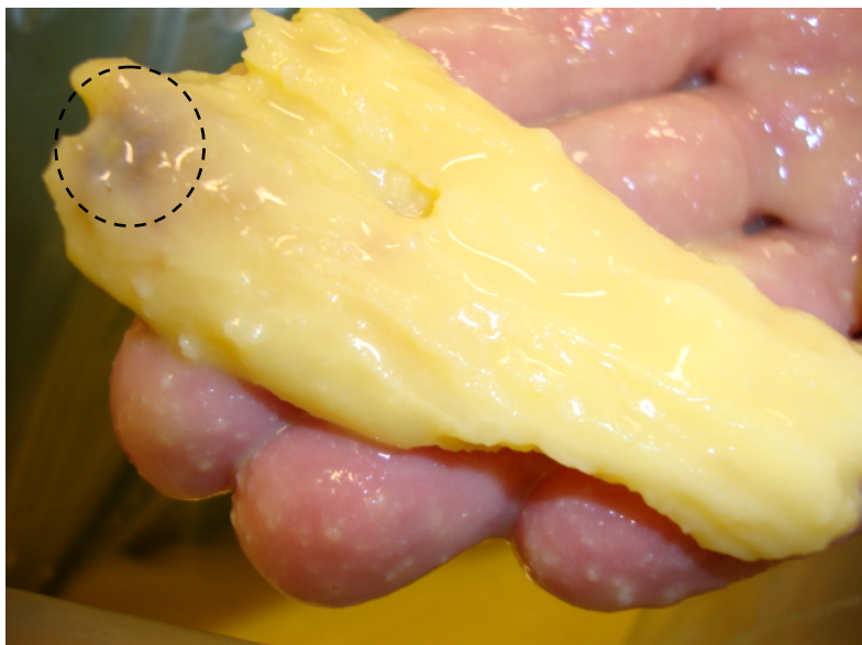
Figure 12: The picture shows the typical appearance of a coagulated BCM element, transported close to the inner surfaces of the tube, exiting from the MW heating system. The dashed circle encloses a scorched part of the coagulated BCM element, resulting from too high temperatures and possibly fouling.
