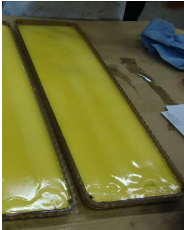
Figure 15: An illustration of the stripe pattern obtained in BCM tray 1 after the MW heating during Run 3 . The more pale yellow color in the outer and center stripes indicates a more coagulated BCM, while the darker yellow color in the other stripes indicates a more fluid BCM.
