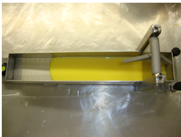
Figure 7: The picture shows one of the many viscosity measurements of BCM performed in the Bostwick device.
