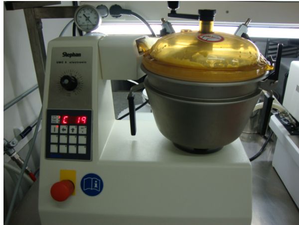
Figure 6: A photograph of the planetary mixer that was used to heat the BCM for the viscosity measurements.
