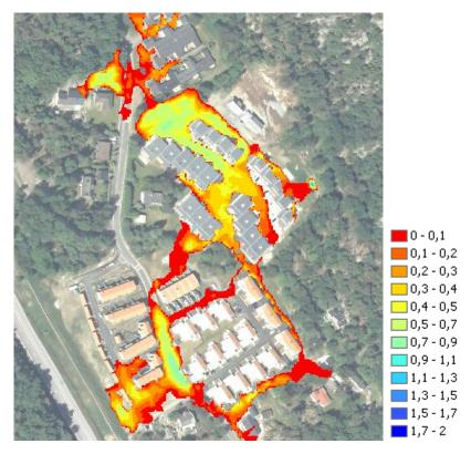
Figure 5-13. Results from final calibration showing maximum flood extent with the rain series from 14.08.2011 as input. Scale is showing flood depth in meters.
