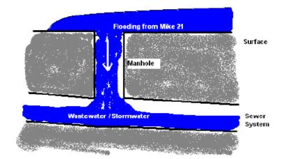
*Figure 3-5. Overland flow reaches an open manhole which leads to an interaction where water is transported from the 2D model to the 1D model (DHI, 2007).*
