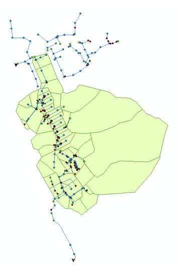
Figure 5-7. The network model for the case area during the model building process. In the figure one can see closed manholes (blue), gully pots (red) and trench intakes (green). Yellow fields are catchments used in the timearea method and the black triangles are the outlets where the model ends.
