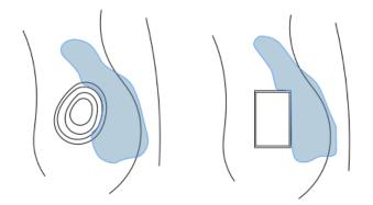
Figure 7-2. Schematic figure on surface water spread on DEM with different accuracy. For same conditions, the model to the left would be interpreted as flooded building whilst the model to the right would not.
