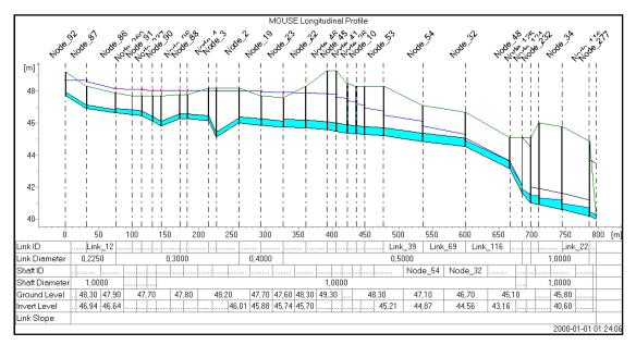
Figure 5-11. First model results from 1D network simulation, north part of stormwater system. Pressure line exceeds ground level which was according to the real rain event.
