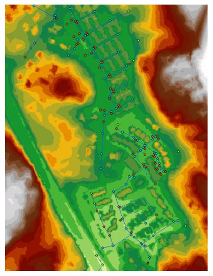
*Figure 5-9. The 1D network model coupled with the 2D elevation model.*
