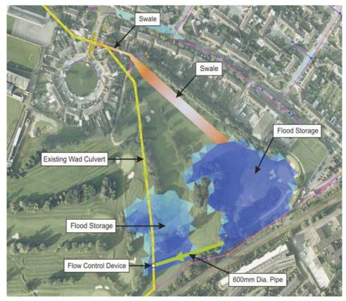
Figure 2-2. Flood alleviation scheme in Dublin. Surface flow paths is controlled and a known flood storage is established (DCC, 2010).
