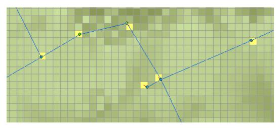
*Figure 3-7. The network models manholes coupled to the grid squares in the digital elevation model.*
