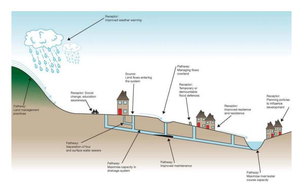
Figure 2-1. Mitigation measures that can be considered to reduce surface water flood risk (DEFRA, 2010).
