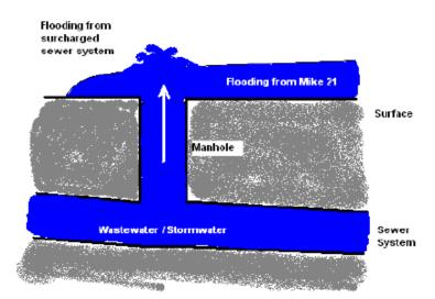
Figure 3-6. The capacity in the storm water network is reached which leads to an interaction where water is transported from the 1D model to the 2D model (DHI, 2007).
