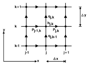
Figure 3-4. Difference grid showing the principle of the alternating technique for solving continuity and momentum conservation equations. p and q is the flux in the different directions, and h is the water level (Mike by DHI, 2011).
