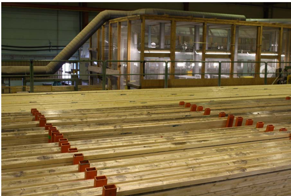
Figure 2.5: Stacked lamellae waiting to be cured by the radiation machine in the background
