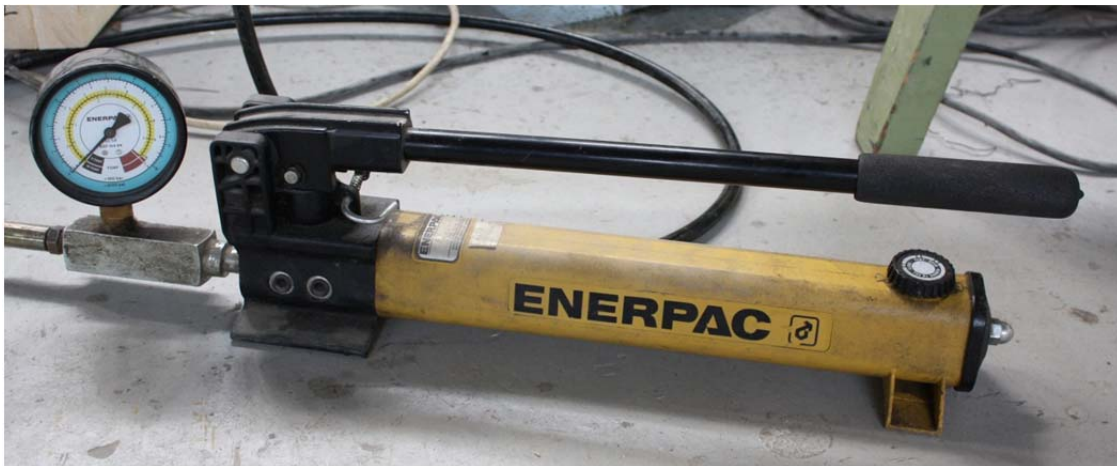
Figure 4.4: Load application by hydraulic jack
