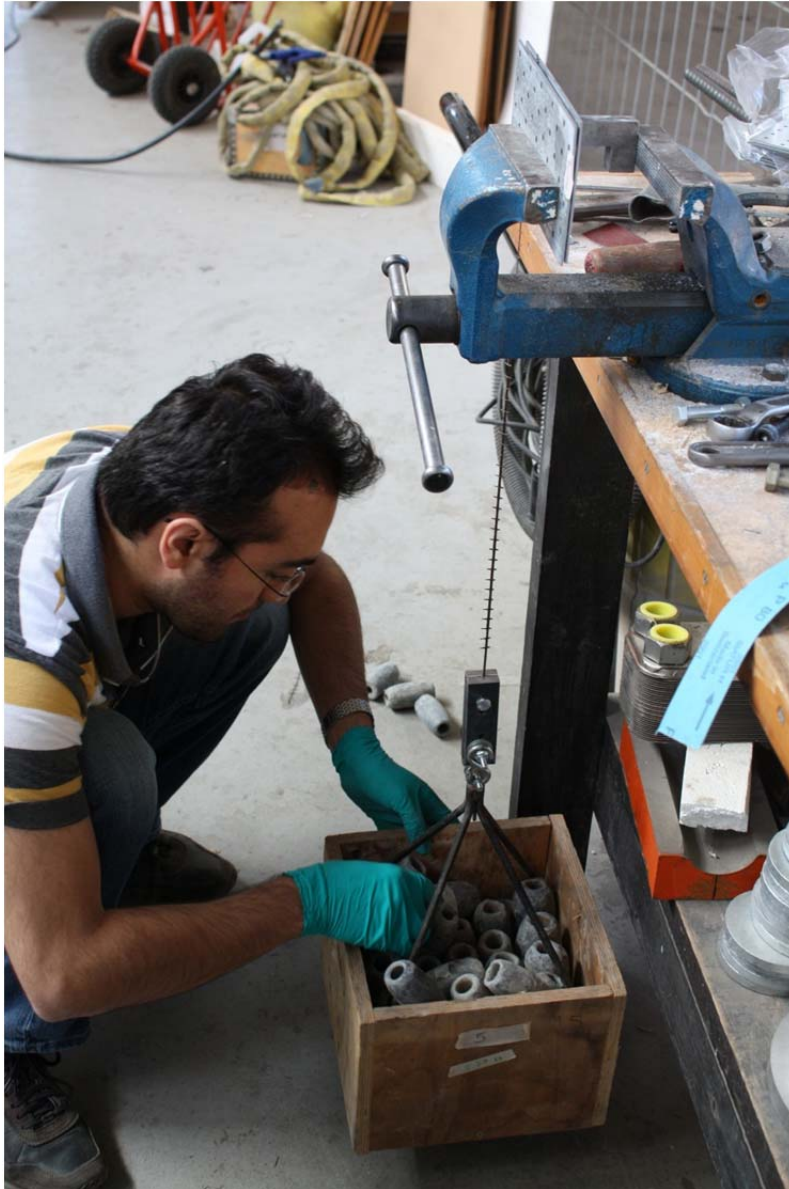
Figure 4.15: Testing of individual mesh BFRP strands
