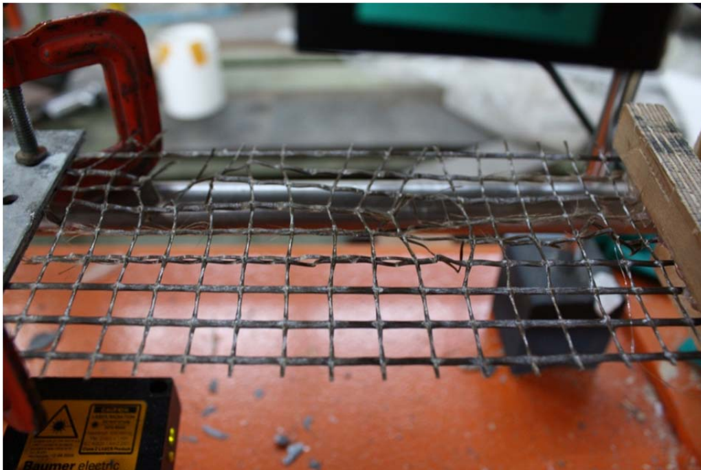
Figure 4.11: Typical results - mesh BFRP, close-up
