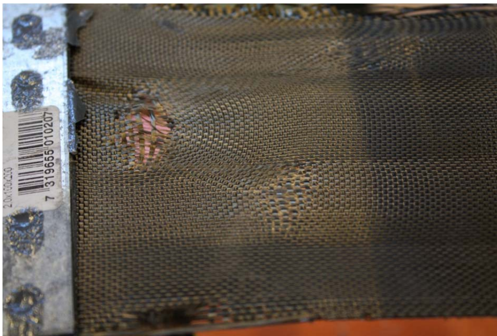
Figure 4.9: Typical results - fabric BFRP, close-up
