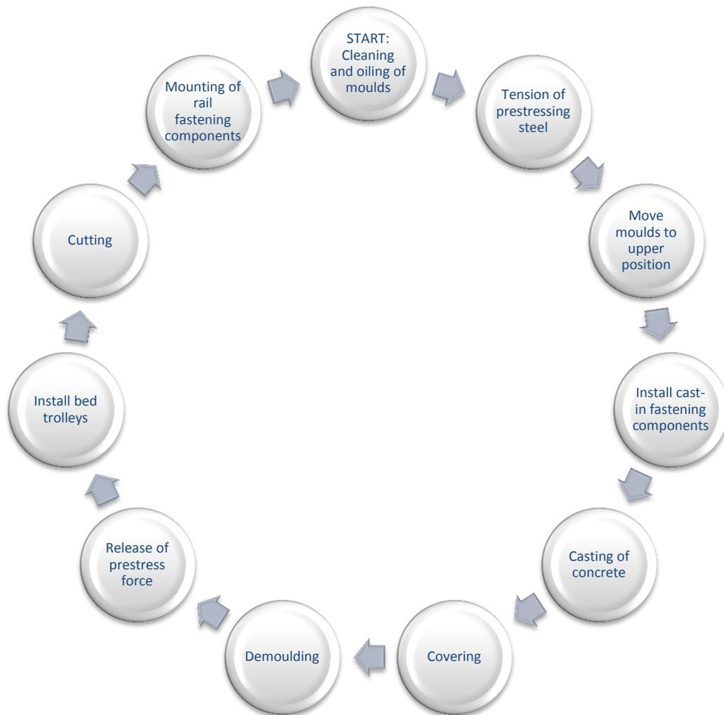
Figure 3.4 Schematic production description of “The Long Line Method”, starts at the top.
