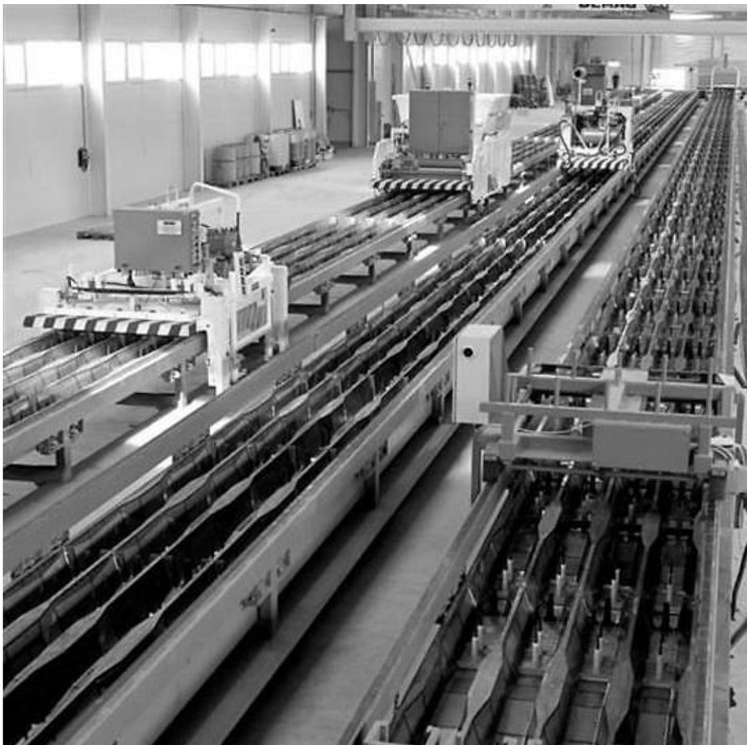
Figure 3.3 “The Long Line Method” with its production equipment, from Abetong (2012).
