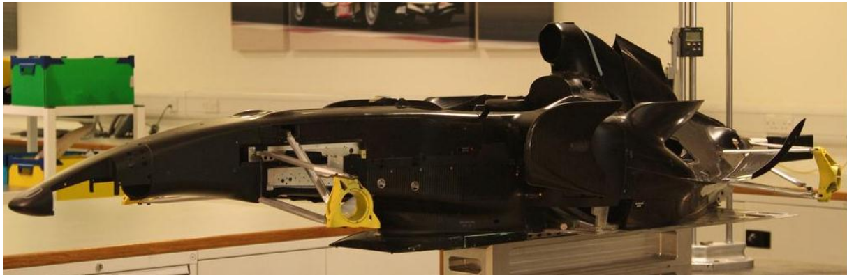
Figure 3.5 Example of a body made of carbon fibre panels
