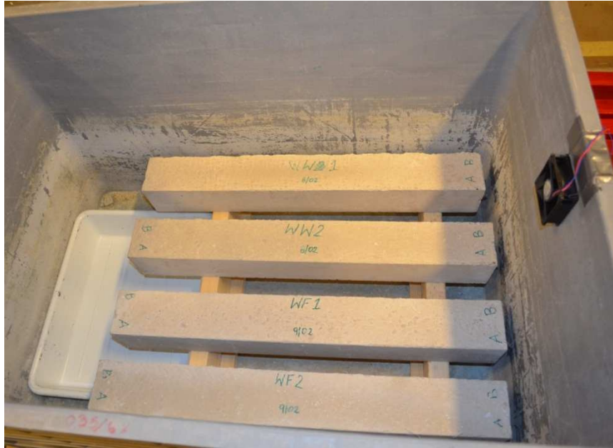
Figure 5.4 The set up to create the exposure conditions for beams from groups U and W. The container with the oversaturated NaCl solution can be seen to the left in the figure.
