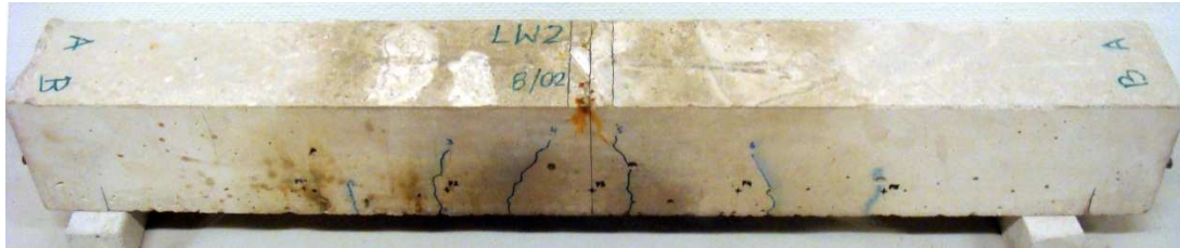
Figure 5.16 View of beam LW2 and crack patterns.
