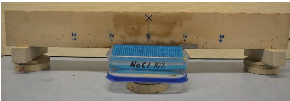
Figure 5.5 Chloride exposure setup
