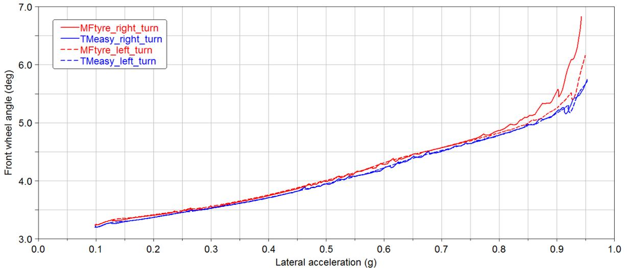
Figure 4.3.1: TMeasy vs. MFtyre constant radius cornering understeer behaviour comparison
