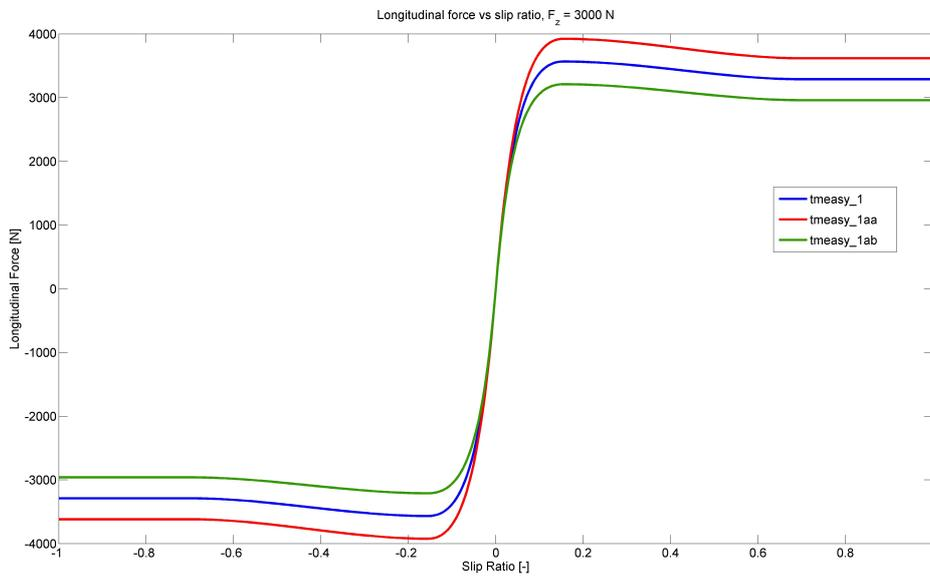
Figure 5.1.1: Longitudinal force vs. slip ratio characteristics for tires *tmeasy\_1*, *tmeasy\_1aa* and *tmeasy\_1ab*
