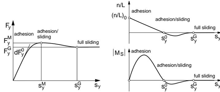
Figure 3.2.3: Typical plots of lateral force, dynamic offset and self-aligning torque
