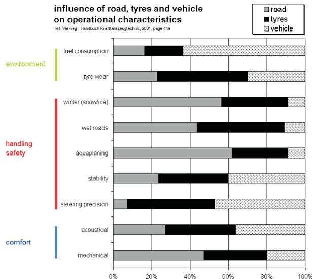
Figure 1.1.1: Influence of road, vehicle and tires on overall operational characteristics [3]
