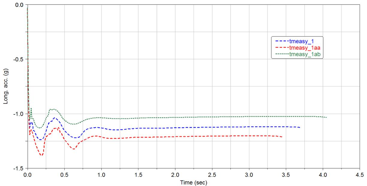
Figure 5.1.2: Longitudinal acceleration sensitivity for straight line braking events with tires *tmeasy\_1*, *tmeasy\_1aa* and *tmeasy\_1ab*
