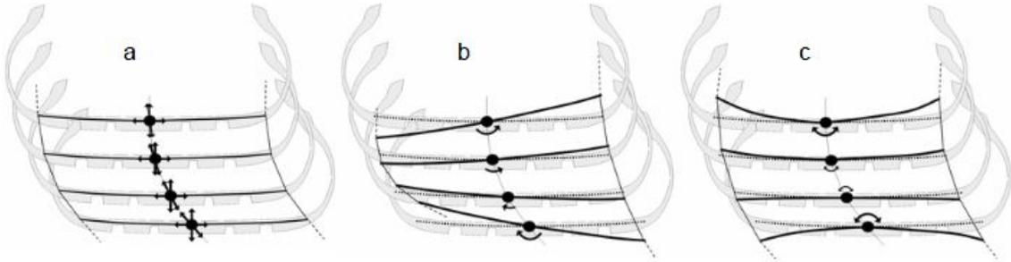
Figure A.0.1: *FTire belt segment degrees of freedom: (a) Translation, (b) Torsion and (c) Lateral bending, [16]*
