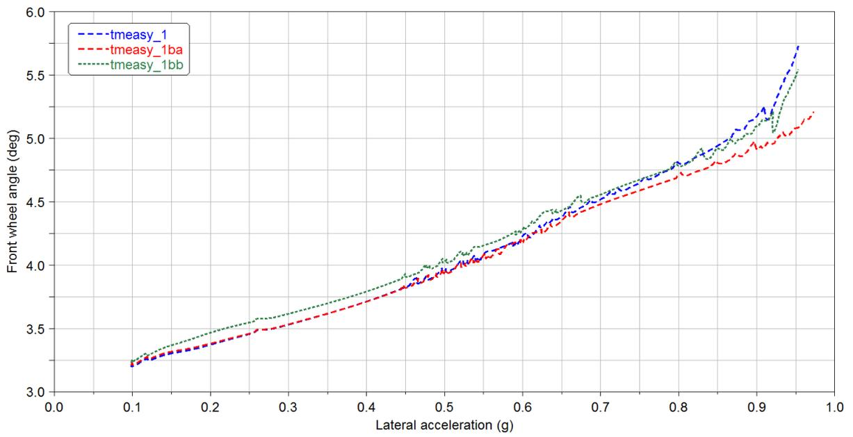
Figure 5.2.2: Understeer gradient for constant radius cornering events with tires *tmeasy\_1*, *tmeasy\_1ba* and *tmeasy\_1bb*
