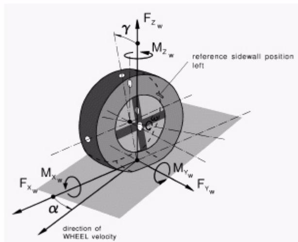
Figure B.0.3: *TYDEX-W axis system used in Adams/Tire*
