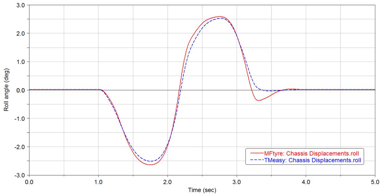
Figure 4.4.3: *TMeasy vs. MFtyre single lance change test chassis roll angle*
