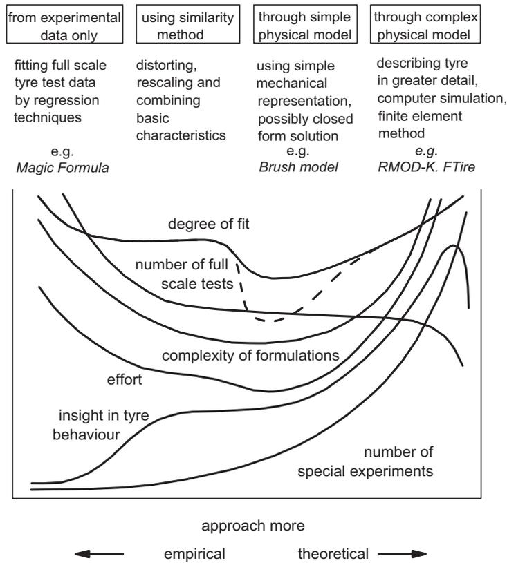
Figure 3.0.1: Four categories of possible types of approach to develop a tire model [25]
