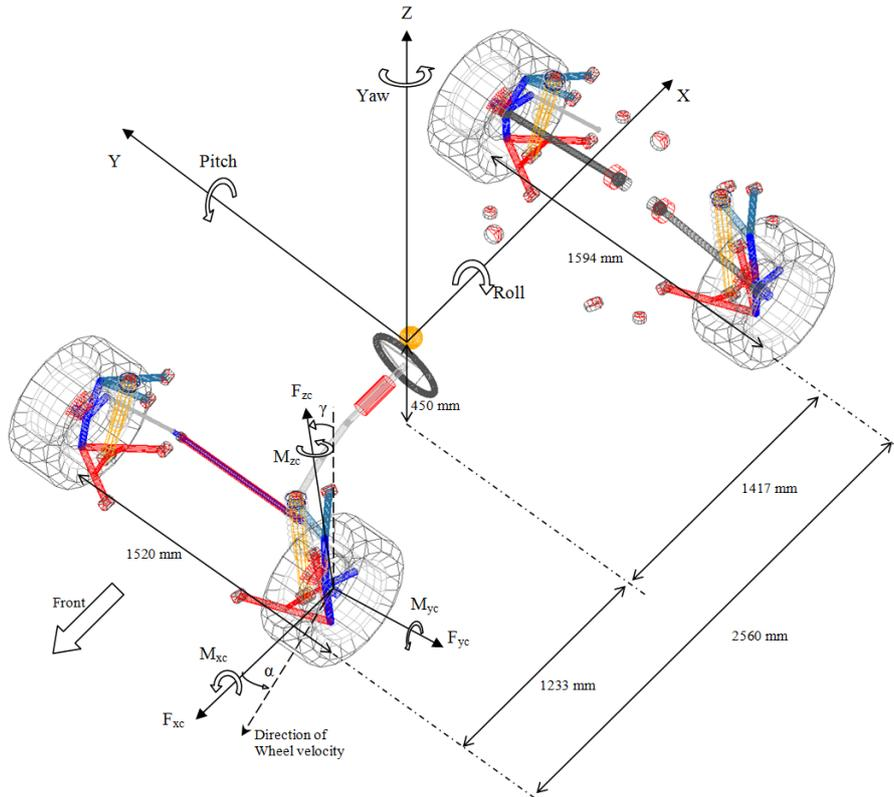
Figure 4.0.1: *Adams/Car Demo vehicle and the TYDEX-C axis system*
