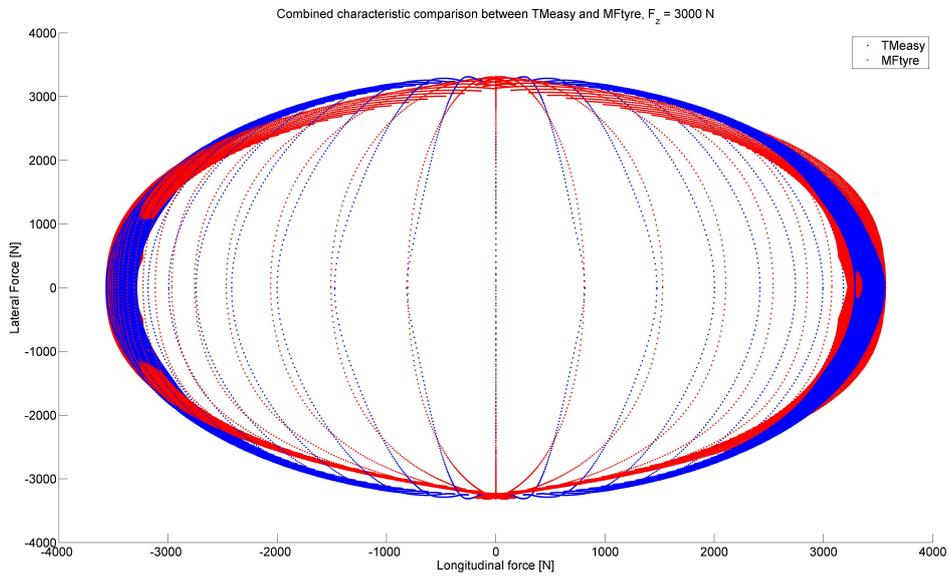
Figure 4.1.4: *Combined slip characteristics*
