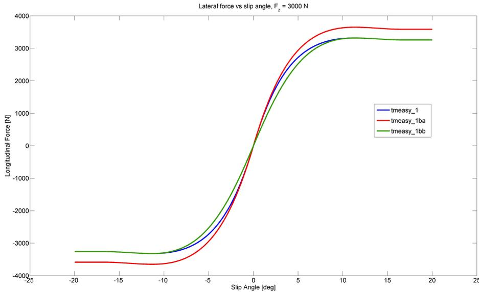
Figure 5.2.1: *Lateral force vs. slip angle characteristics for tires tmeasy\_1, tmeasy\_1ba and tmeasy\_1bb*
