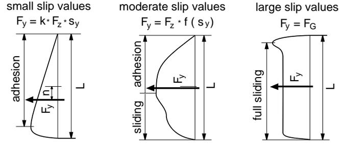
Figure 3.2.2: Lateral force distribution over the contact area for different slip values
