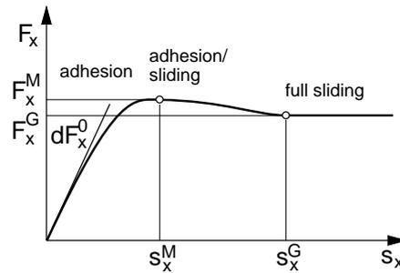
Figure 3.2.1: *Typical longitudinal force characteristics*
