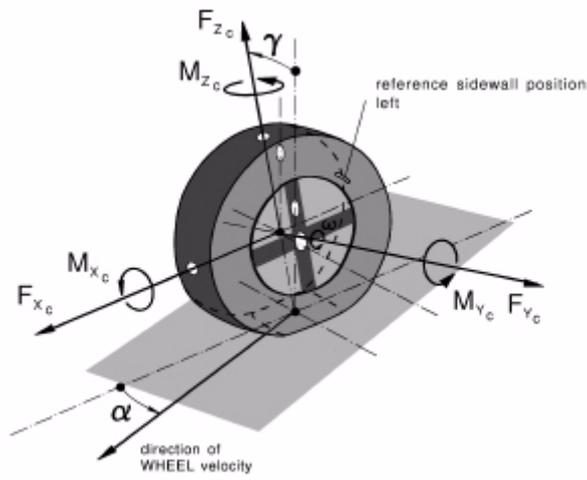
Figure B.0.2: *TYDEX-C axis system used in Adams/Tire*
