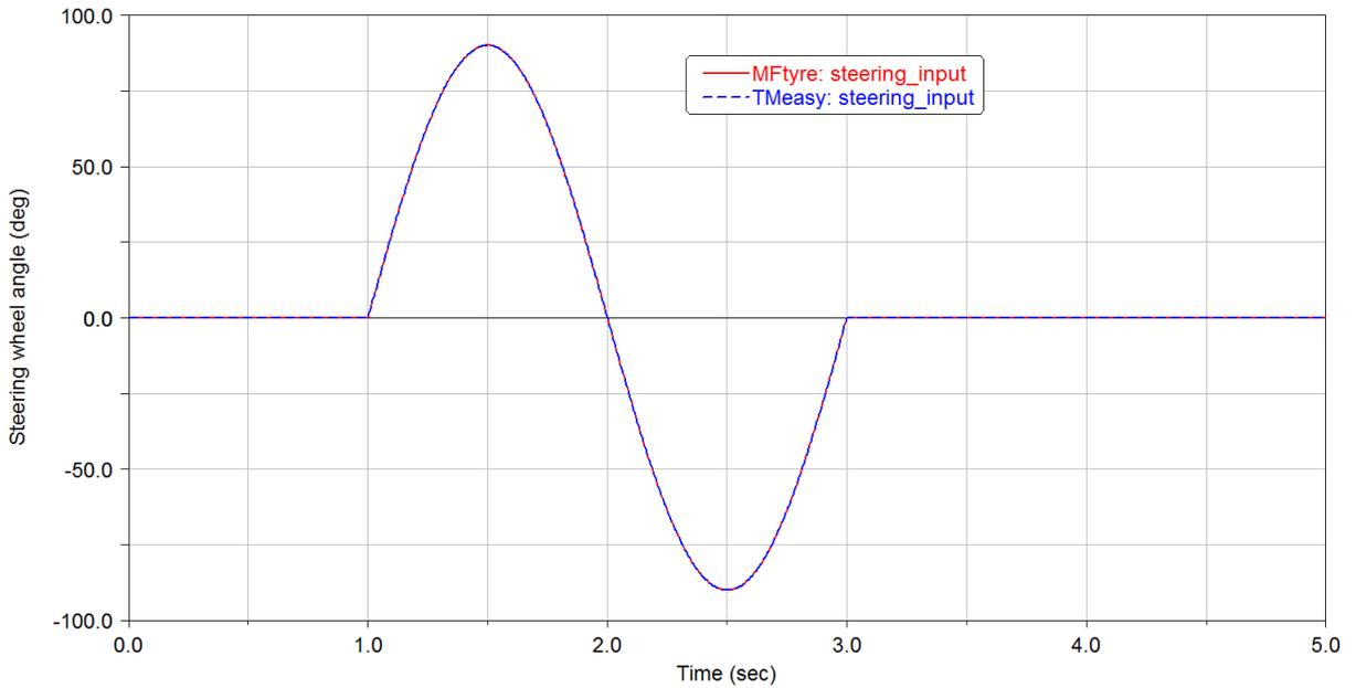
Figure 4.4.1: *TMeasy vs. MFtyre single lane change test steering input*
