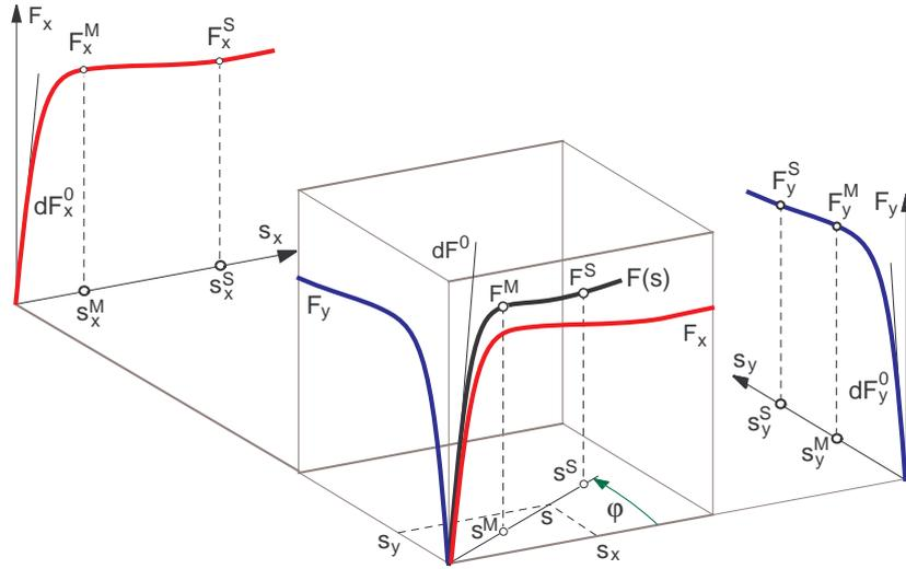
Figure 3.2.4: Generalized tire characteristics [19]
