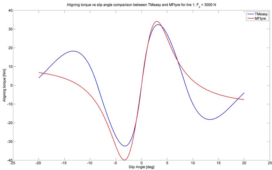
Figure 4.1.3: *Self-aligning torque characteristics*
