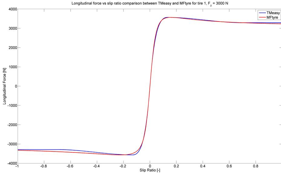
Figure 4.1.1: *Longitudinal force characteristics*
