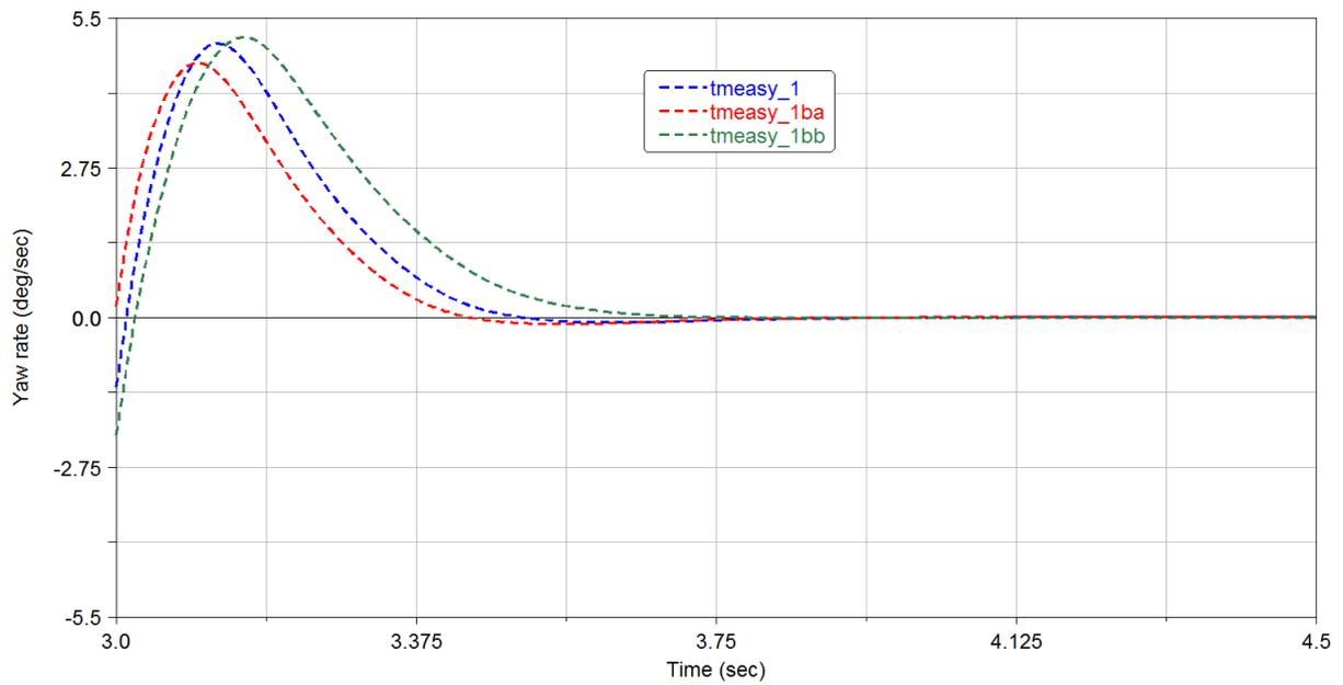
Figure 5.3.2: Yaw rate settling after  $t = 3$  sec for single lane change events with tires *tmeasy\_1*, *tmeasy\_1ba* and *tmeasy\_1bb*
