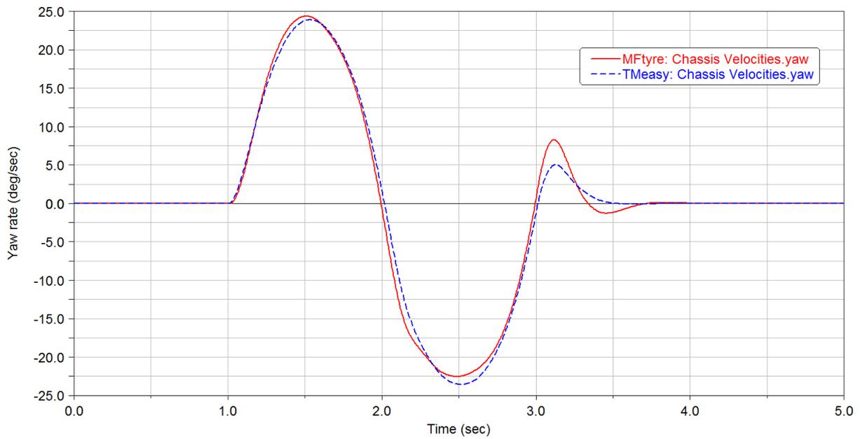
Figure 4.4.2: *TMeasy vs. MFtyre single lance change test chassis yaw rate*
