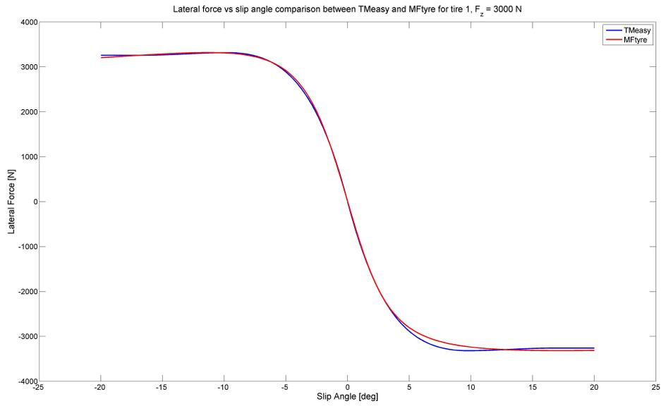
Figure 4.1.2: *Lateral force characteristics*
