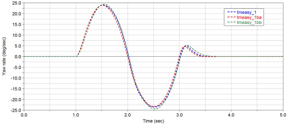
Figure 5.3.1: Yaw rate for single lane change events with tires tmeasy\_1, tmeasy\_1ba and tmeasy\_1bb
