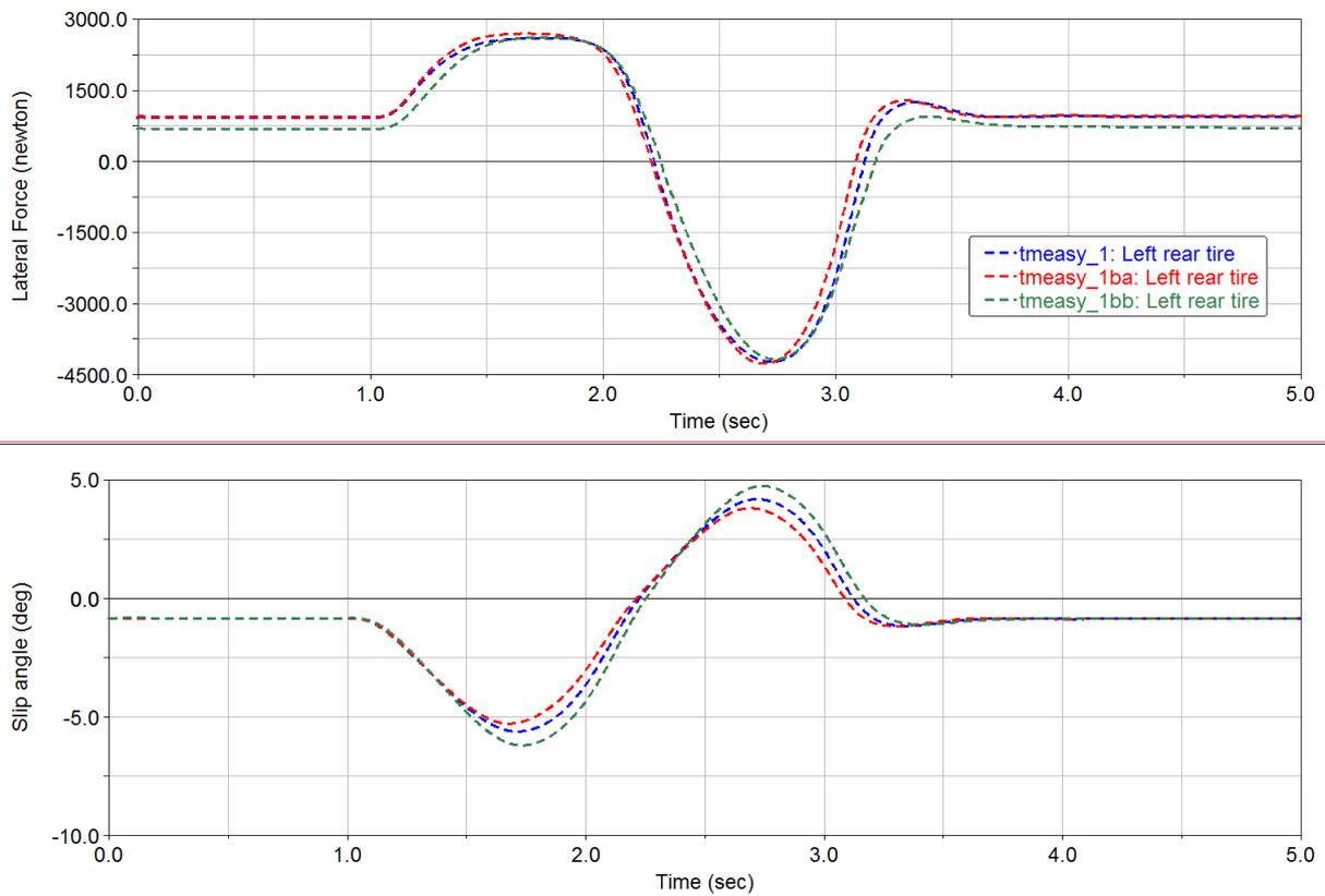
Figure 5.3.3: Lateral force on the left rear tire for single lane change events with tires *tmeasy\_1*, *tmeasy\_1ba* and *tmeasy\_1bb*
