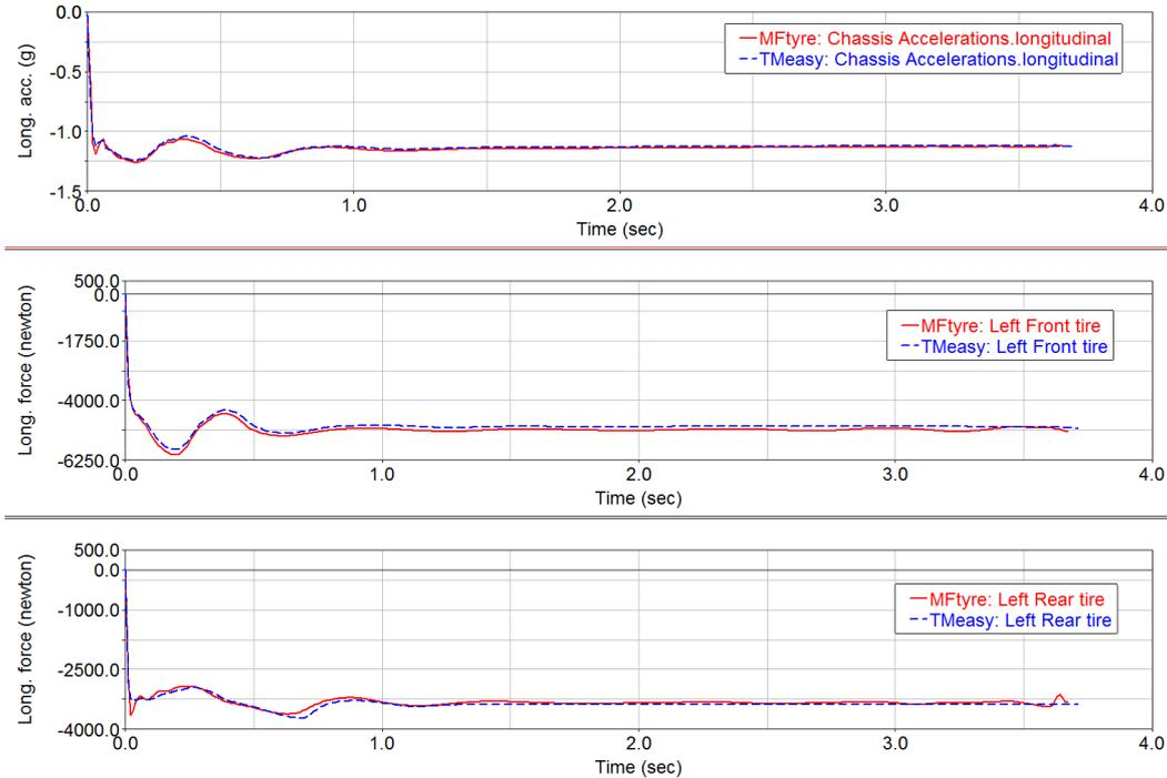
Figure 4.2.1: *TMeasy vs. MFtyre straight line braking results: (top) longitudinal acceleration (middle) longitudinal force on the left front tire (bottom) longitudinal force on the left rear tire*
