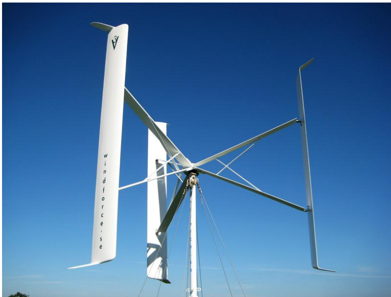
Figure 18. H-Darrieus type small vertical axis wind turbine. [15]
