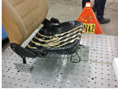
Figure 2.2.5: Measuring the geometry of the seat structure.
