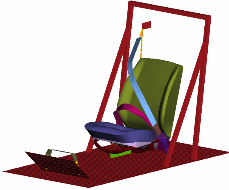
Figure 2.2.9: Simulation model of the Heidelberg sled.
