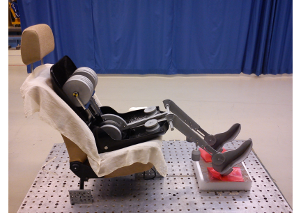
Figure 2.2.6: Measuring of the H-point with an H-point dummy.
