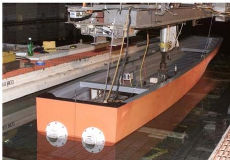
Figure 4.6 Model scale self-propulsion test setup [39]
