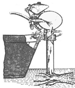
Figure 1.6 Sketch by Schult of H. J. MacCollum's (1946) Pulse Jet Outboard [5]
