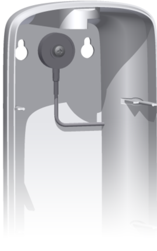
Figure 5.5: The first prototype of the donut concept. A donut shaped load cell was mounted with a screw and washer.
