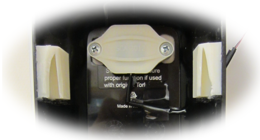
Figure 5.8: The 3D printed prototype mounted in a dispenser. The refill supports were made slightly too big and had to be cut off for the refill to fit.
