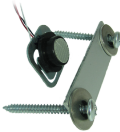
Figure 5.6: In the second prototype of the donut concept, the donut load cell was replaced by a more affordable micro load cell.
