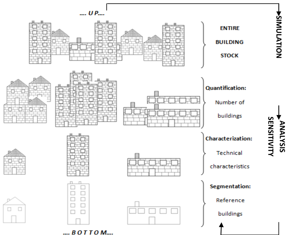
Figure 3.1: Methodology based on a bottom-up approach to describe the building stock through archetype buildings, used in this master thesis.
