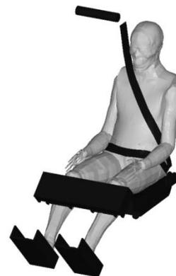
*Figure 3. THUMS in the sled test*
