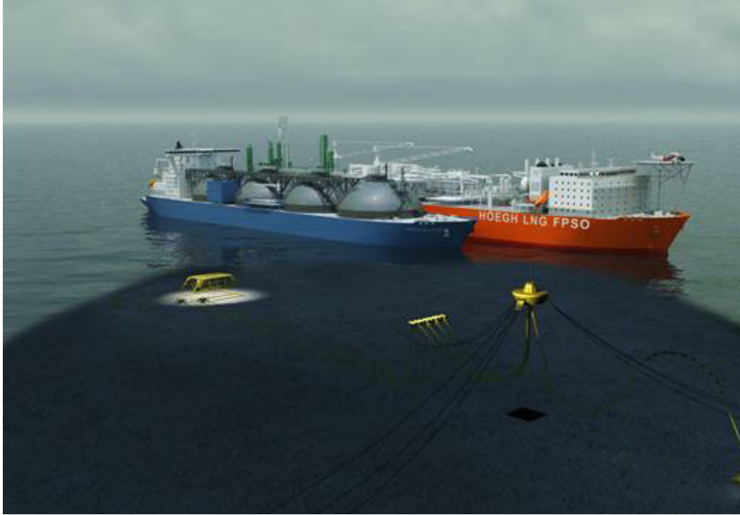
Fig. 6. Side-by-side transfer operation – Courtesy of Høegh LNG.
