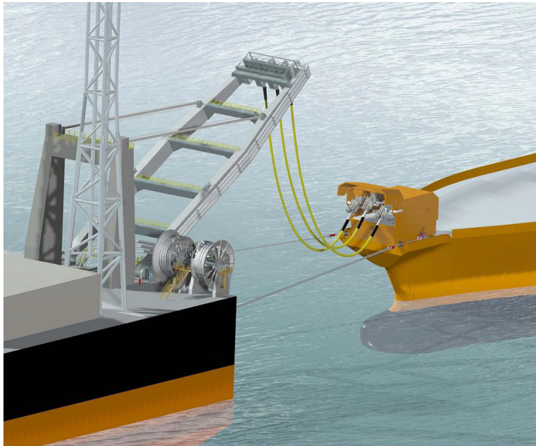
Fig. 7. Tandem offloading system – Courtesy of FRAMO.
