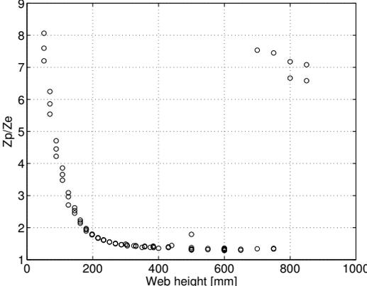
**Fig. E1.** The plastic/elastic section modulus ratio ( $Z_p/Z_e$ ) for profiles in beam database attached to plate with thickness 25mm and a frame spacing of 600mm corresponding to Ship I.
