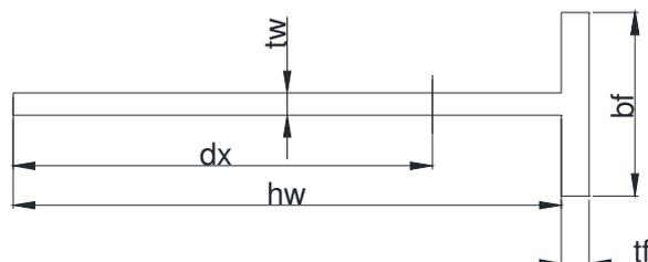
**Fig. D2.** T-profile with dimensions.
