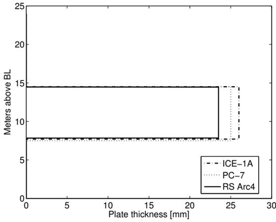
(a). Height over BL versus plate thickness.
