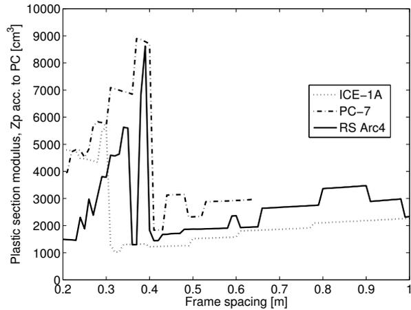
(d). Section modulus depending on frame spacing.
