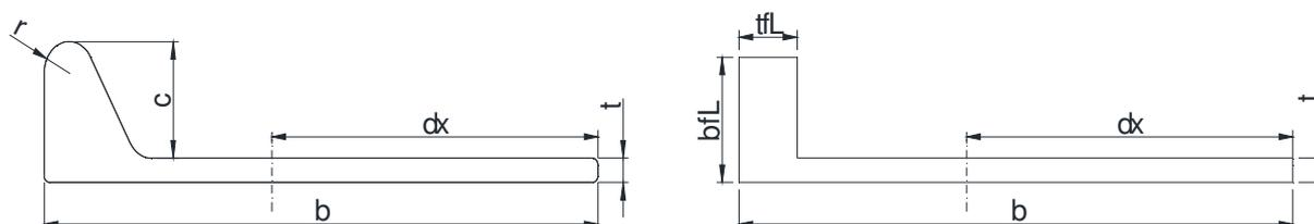
**Fig. D1.** A flat bulb steel and an L-profile with dimensions.
