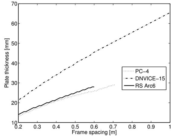
(b). Plate thickness depending on frame spacing.
