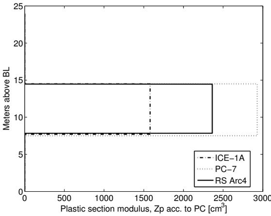
(c). Height over BL versus section modulus.
