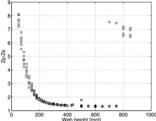
**Fig. E2.** The plastic/elastic section modulus ratio ( $Z_p/Z_e$ ) for profiles in beam database attached to plate with thickness 32mm and a frame spacing of 500mm corresponding to Ship II.
