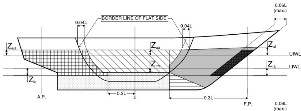
**Fig. 4.** Hull area extent of DNV ICE and DNV POLAR [5].
