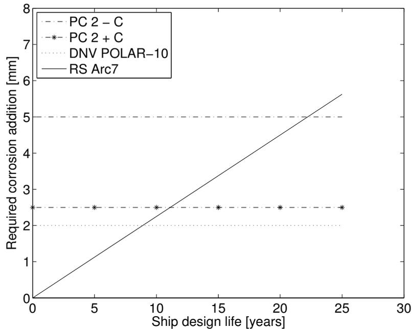
**Fig. 24.** Required corrosion and abrasion addition for notations in Case III.
