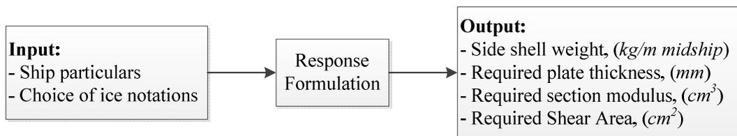
**Fig. 16.** Schematic of calculation procedure.
