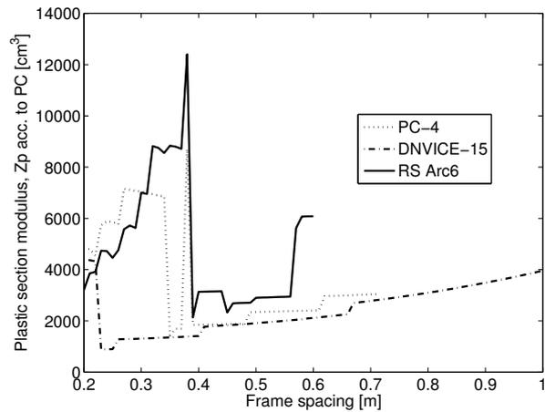
(d). Section modulus depending on frame spacing.
