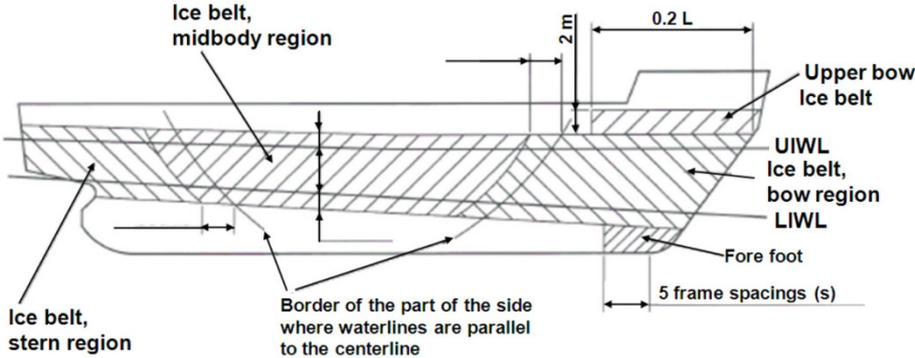
**Fig. 3.** Hull area extent of the FSICR [5].
