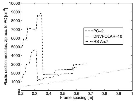
(d). Section modulus depending on frame spacing.
