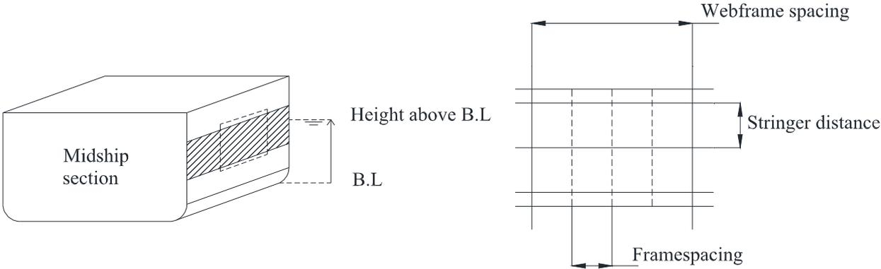
**Fig. 7.** Side shell structure of a transversely framed mid-body.
