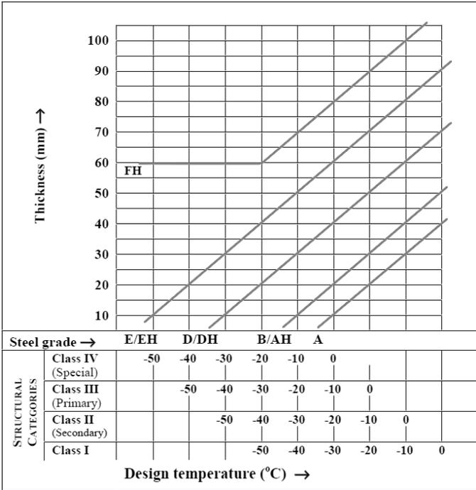
**Fig. 14.** Required steel grades according to DAT ( $-X^{\circ}\text{C}$ ) [5].
