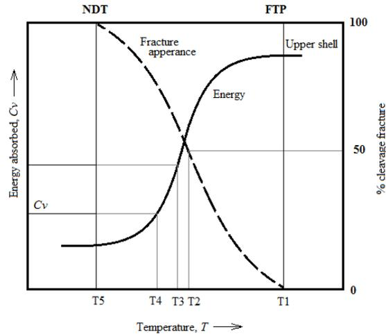
**Fig. 15.** Typical transition temperatures from Charpy V-notch tests.
