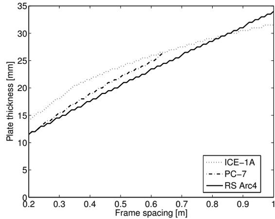
(b). Plate thickness depending on frame spacing.
