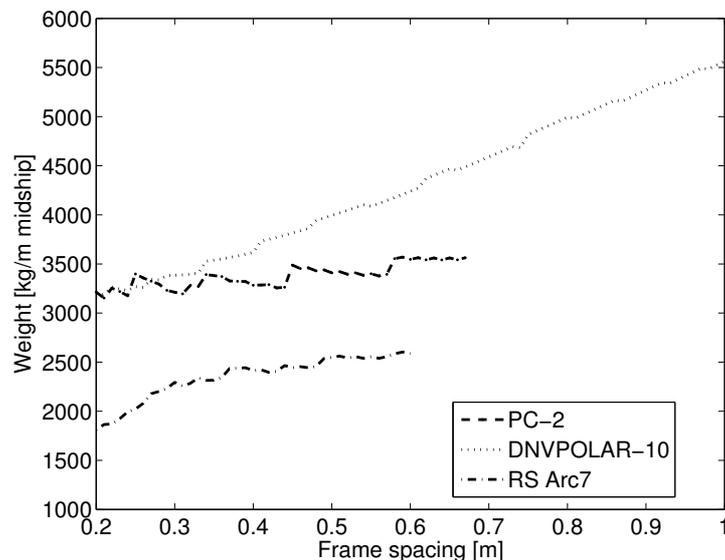
**Fig. 25.** Weight calculation for Case III depending on frame spacing.
