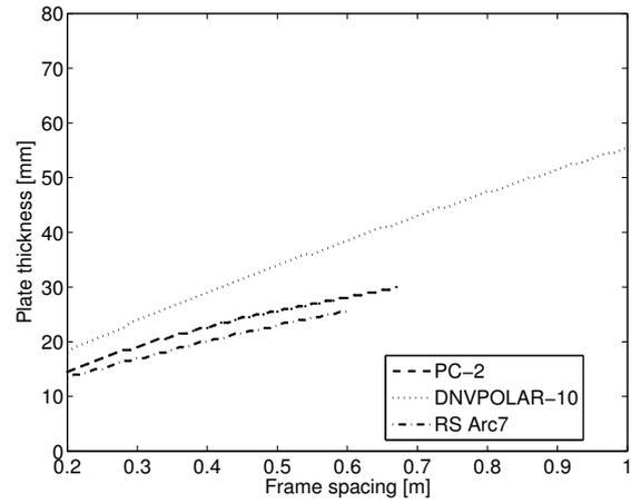
(b). Plate thickness depending on frame spacing.
