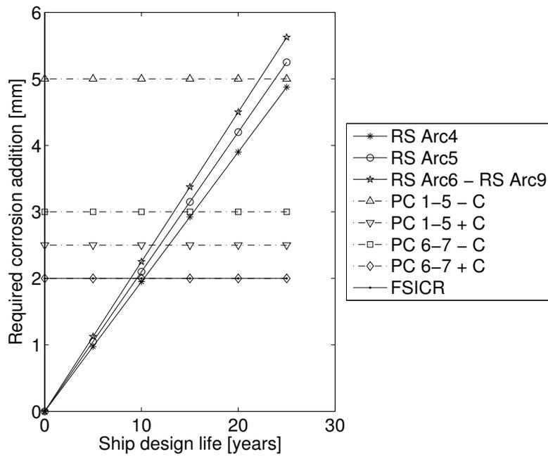
**Fig. 26.** Required corrosion and abrasion addition on structural members of each rule-set.
