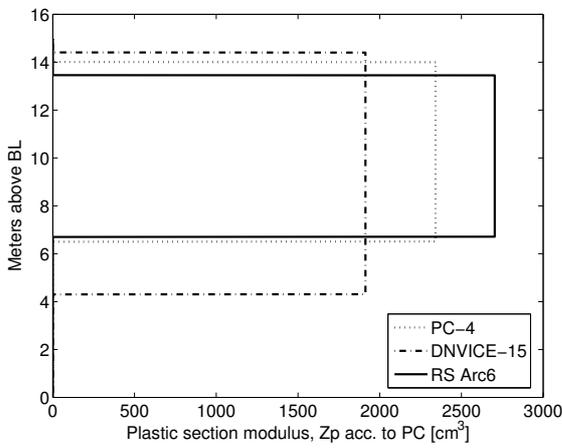
(c). Height over BL versus section modulus.
