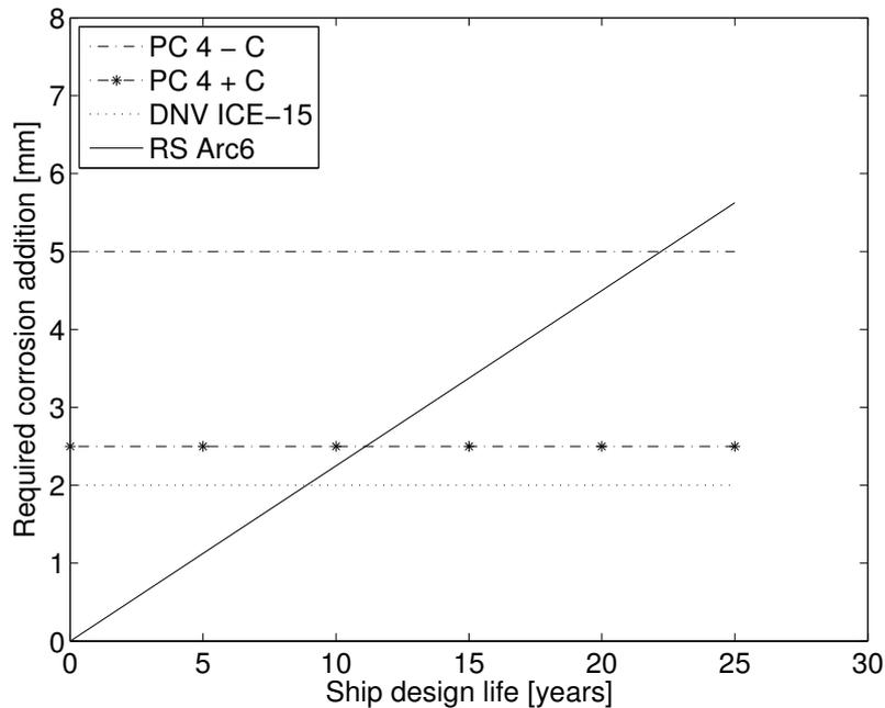
**Fig. 21.** Required corrosion and abrasion addition for notations in Case II.
