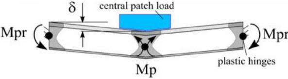
**Fig. 10.** 3-Hinge collapse (centrally loaded fixed-fixed frame) [14].
