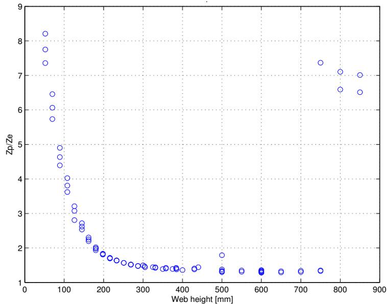
**Fig. 13.** The plastic/elastic section modulus ratio ( $Z_p/Z_e$ ) for Ship I.
