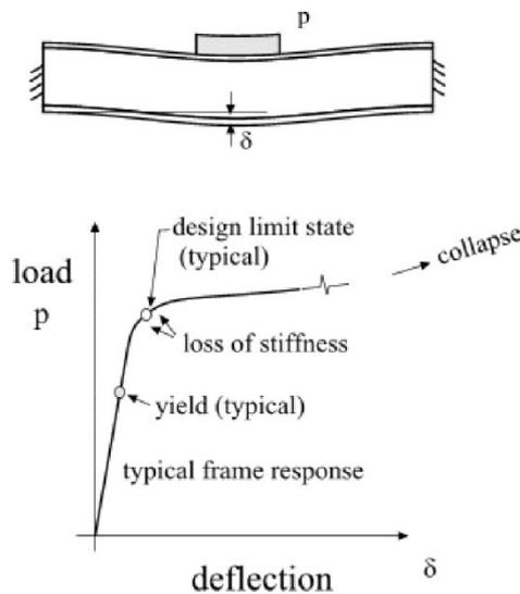
**Fig. 9.** Load-deflection curve of a frame showing design points [14].
