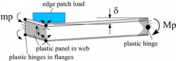
**Fig. 11.** Asymmetric shear collapse (end-loaded fixed-fixed frame) [14].
