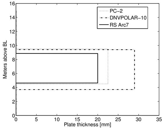
(a). Height over BL versus plate thickness.
