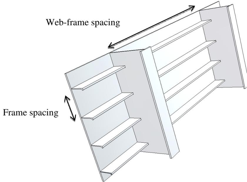
**Fig. 8.** Side shell structure with longitudinal framing.
