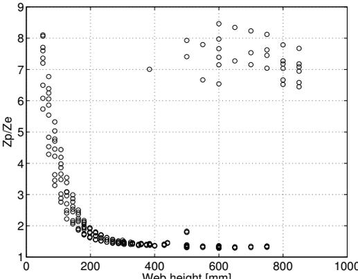
**Fig. E3.** The plastic/elastic section modulus ratio ( $Z_p/Z_e$ ) for profiles in beam database attached to plate with thickness 25mm and a frame spacing of 400mm corresponding to Ship III.
