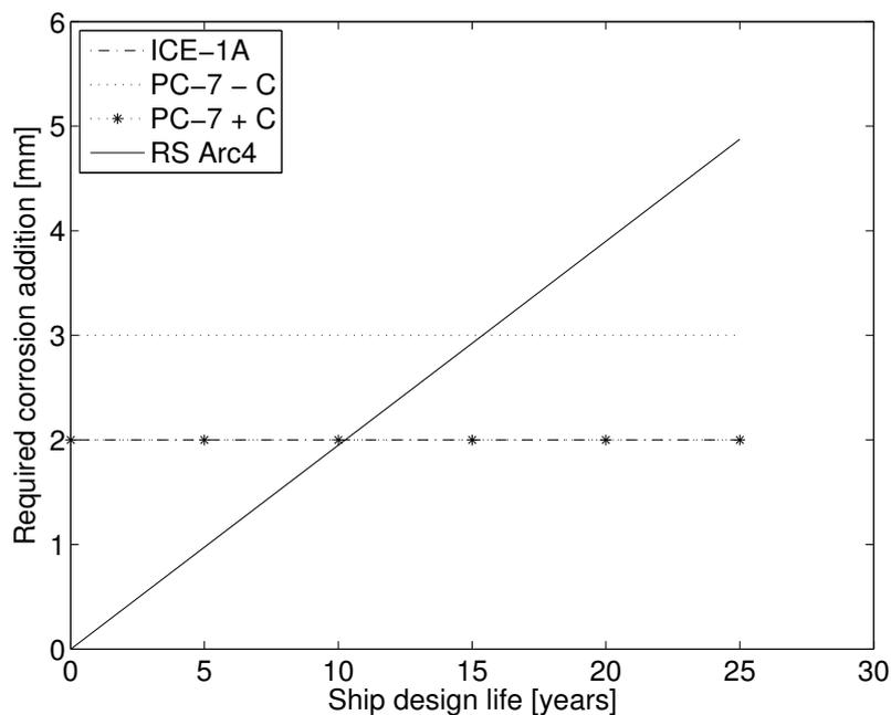
**Fig. 18.** Required corrosion and abrasion addition for notations in Case I.
