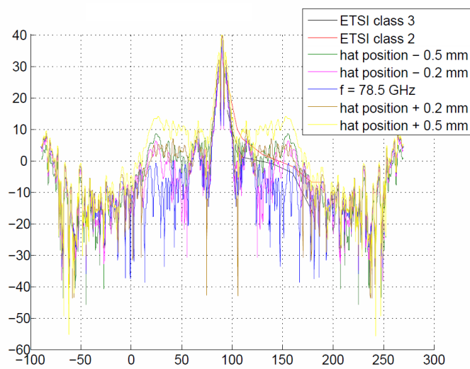
Figure 5.6: Radiation pattern of the one dimensional reflector inside the parallel plate, by changing the position of the hat 0 - 0.5 mm, upwards and downwards
