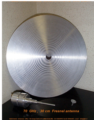
Figure 2.2: Fresnel flat reflector [5]
