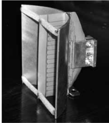
Figure 2.3: Cylindrical parabolic reflector, fed by printed antenna array [8]
