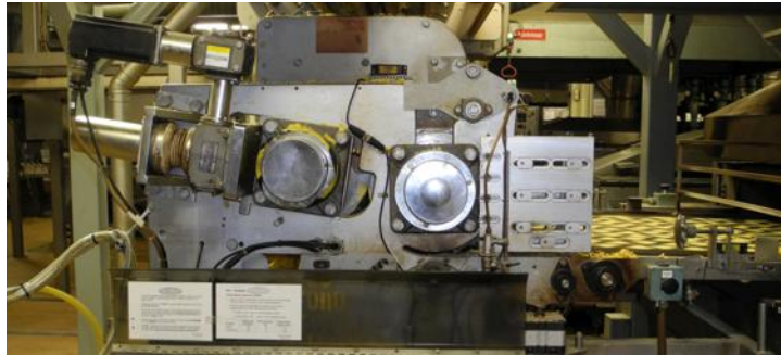
Figure 17: Chips leaving the forming operation during the manufacturing.
