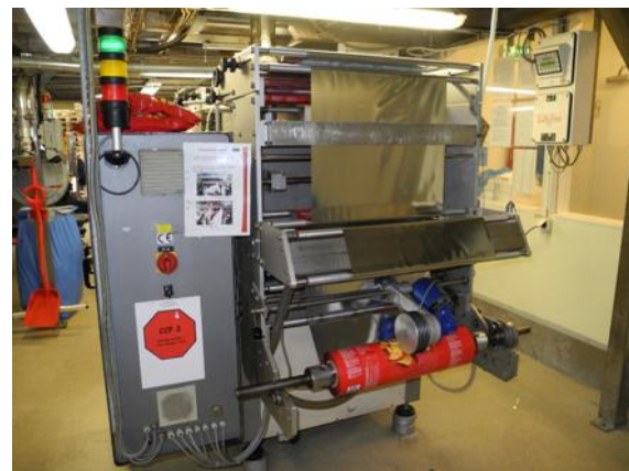
Figure 11: Foil roll mounted in the sealing equipment.
