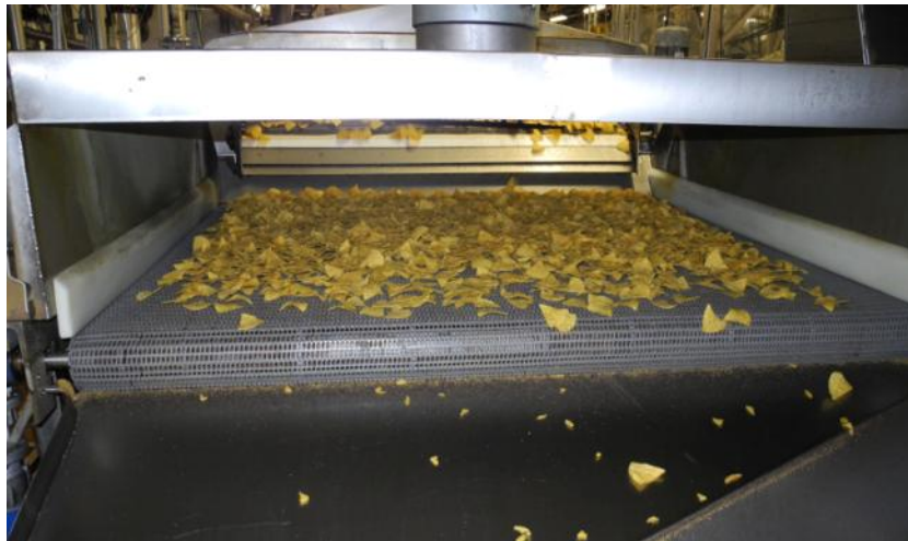
Figure 20: Chips on a cooling conveyor leaving the frying process.
