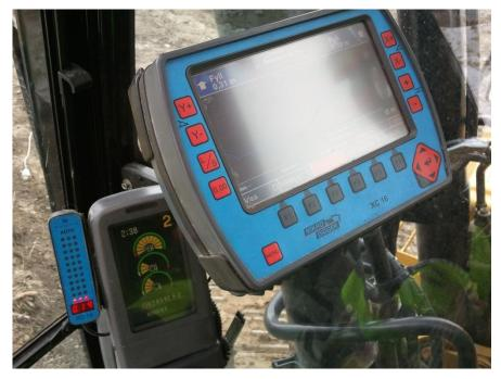
Figure 8: Shows the computer used by the operator, where the DTMs are controlled.
