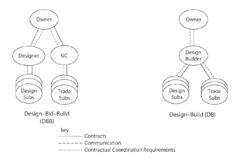
Figure 4: Schematic diagram of Design-Bid-Build and Design-Build processes (modified from Eastman, et al. 2011)
