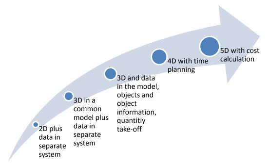
Figure 9: The different stages in the "BIM-ladder" with an increasing level of BIM to the right.
