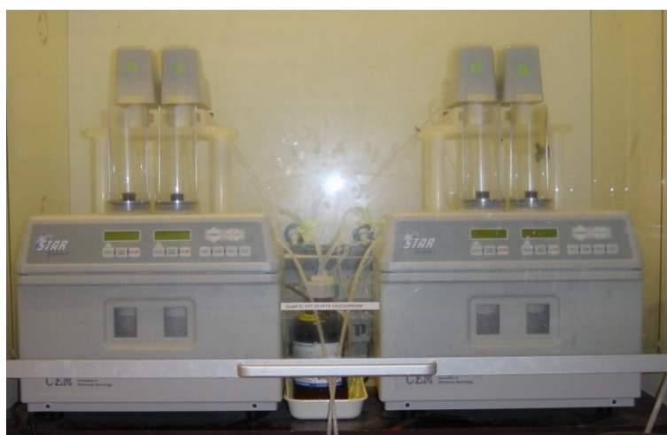
Figure 4. The two microwave ovens connected to the two chemical bottles, nitric acid and hydrogen peroxide (lying in between the two ovens).
