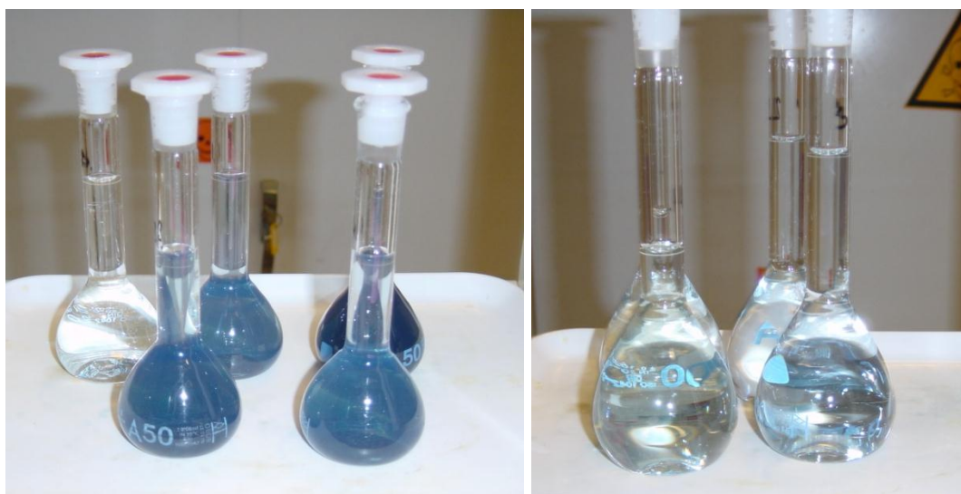
Figure 5. These are an image of when samples from 1 st chlorination reactor (left) and 2 nd chlorination reactor (right) were processed. The colorless flask (left image) is the blank that was done.
