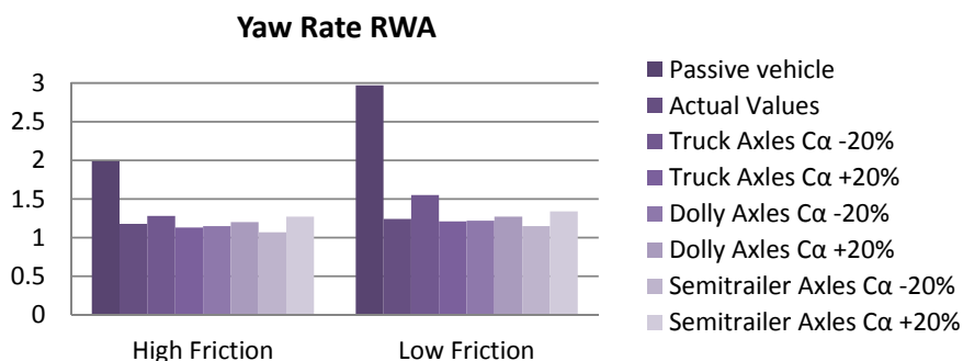
Figure 5.4 Effect of tire cornering stiffness ( C\alpha ) uncertainties on the achieved yaw rate RWA
