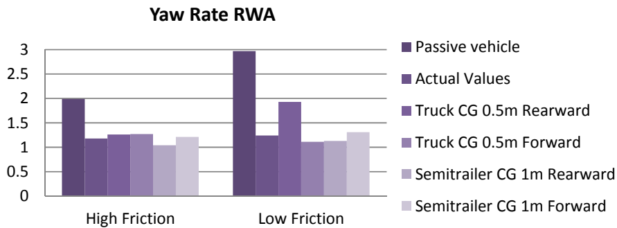
Figure 5.10 Effect of CG location uncertainties on the achieved yaw rate RWA
