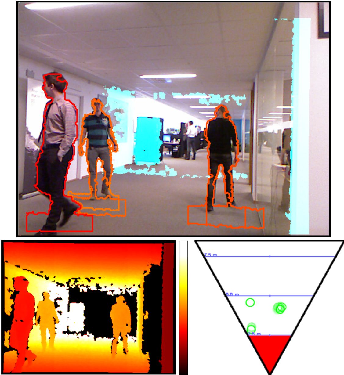
Figure 4.3.1: The figure shows a screen capture of the proof of concept display. In the top image, found humans are marked with their contour in a color corresponding to their distance from the camera. The color coded depth map is shown in the bottom left image and an overview position display is shown in the bottom right image. The color bar in the middle corresponds to the distances shown in the position overview. Marked distances are 2.5 m, 5 m and 7.5 m respectively. The red region in the overview and teal regions in the top image are outside of the detection area.
