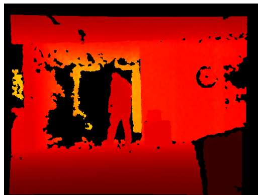
(d) The depth map created from the Kinect.
