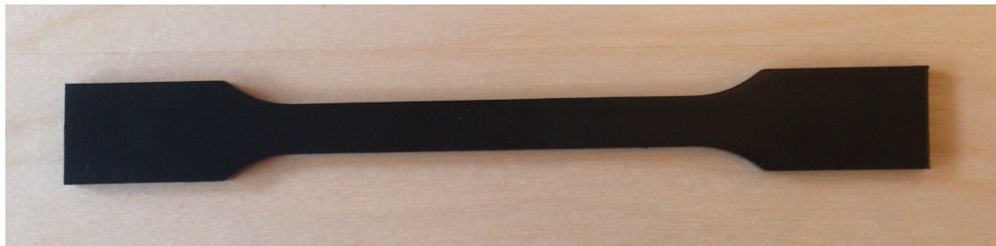
Figure 1.1.2: Injection moulded test piece used for tensile testing.
