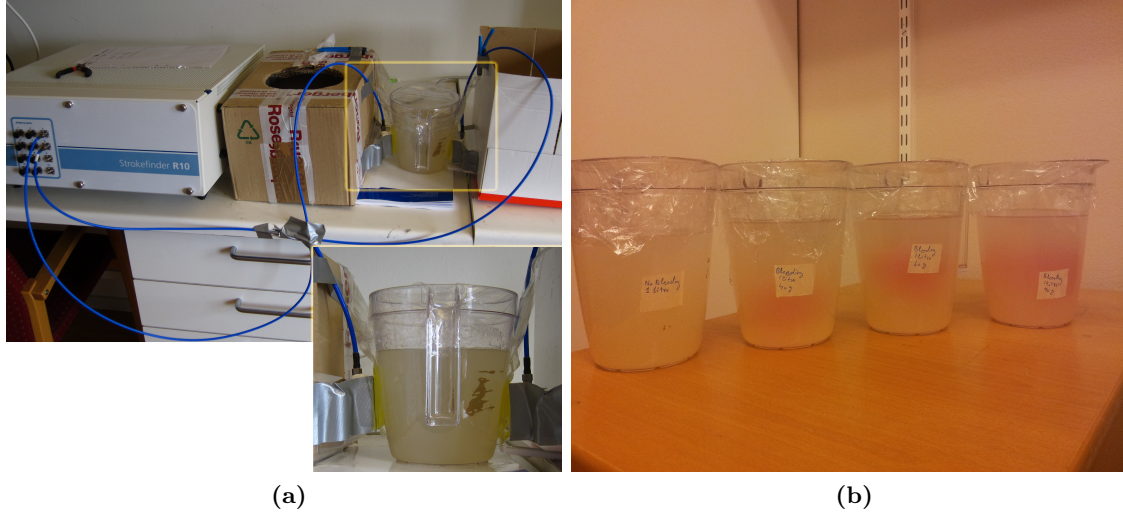
Figure 2.6: (a) Experimental setup used. (b) Shows four buckets, one without bleeding and other contains 40, 60 and 90 grams of bleeding.
