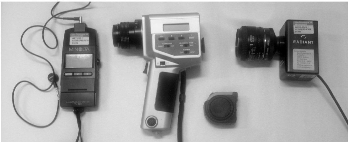
Figure 16: Equipment, from left, Illuminance meter, Luminance meter, Photospectrometer
