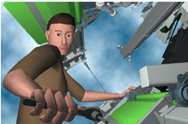
Figure 20. Usage of human mannequin in ergonomics simulation (Dassault Systemes, 2012).
