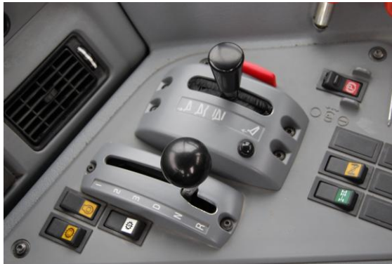
Figure 31. Side console in an articulated hauler.
