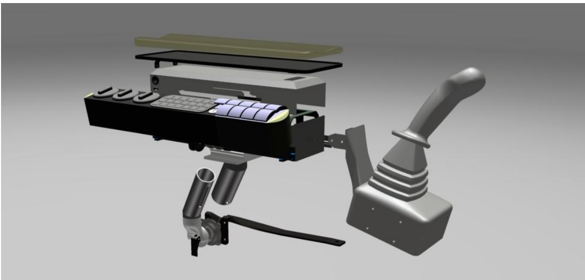
Figure 55. Exploded view of the side console.
