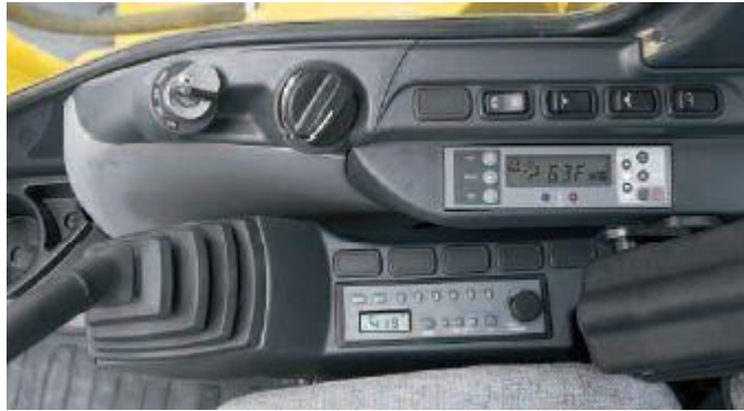
Figure 32. Side console in a Kobelco excavator (Kobelco, 2009).
