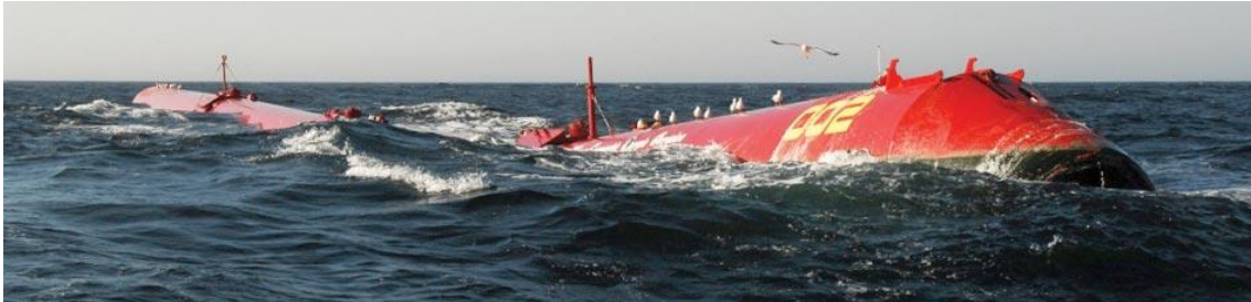
Figure 4.18: Snake shaped wave turbine of Pelamis (2012) © 2012 Pelamis Wave Power.
