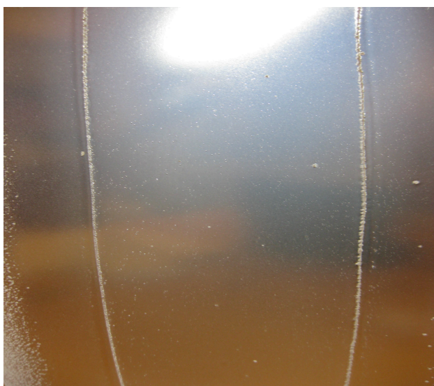
Figure 28: Image of the EC10/HPC-SSL film. Some dried particles visible on the film surface together with small bubbles.
