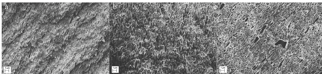
Figure 19: Images of the cross sections of a HPC-SSL film. a) is a cross-sectional image of a film that was not in contact with water, b) is a image of a film that was exposed to water in the diffusion cell and c) is a image of a film where the cross section was exposed to water. All images are of 10 000 times magnification and the scale bar show 1 \mu\text{m} .
