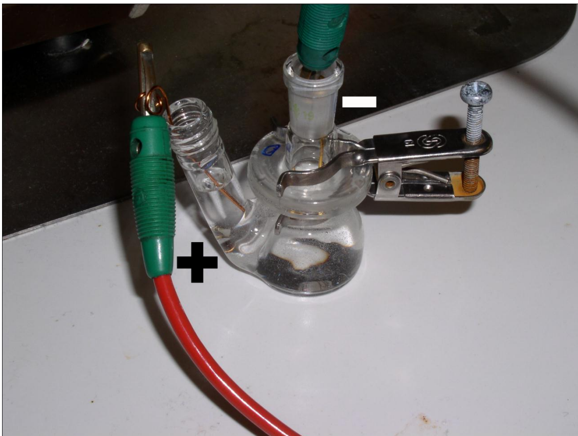
Figure 8 - A picture of how the iontophoresis equipment was setup during the experiment.
