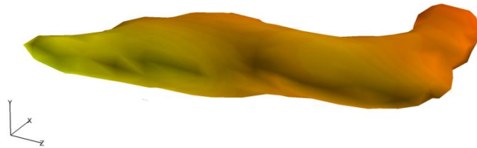
Figure 16. Plot of iso-surface of a vortex contained in the domain \Omega \in [-13,1] \times [-21,-7.5] \times [110,145] mm, for which a FTLE field was calculated. The vortex is colored by velocity magnitude.
