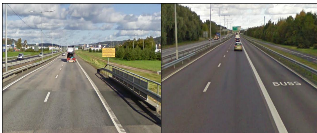
Figure 2.6. The picture to the left demonstrate the present situation. On the right hand side it is demonstrated how the additional bus lane will look. (Google Maps, 2009)
