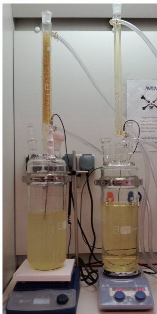
Figure 12: 3 l reactor vessel
