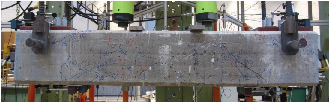
Figure 3.15 Final crack pattern of west side of beam M5.
