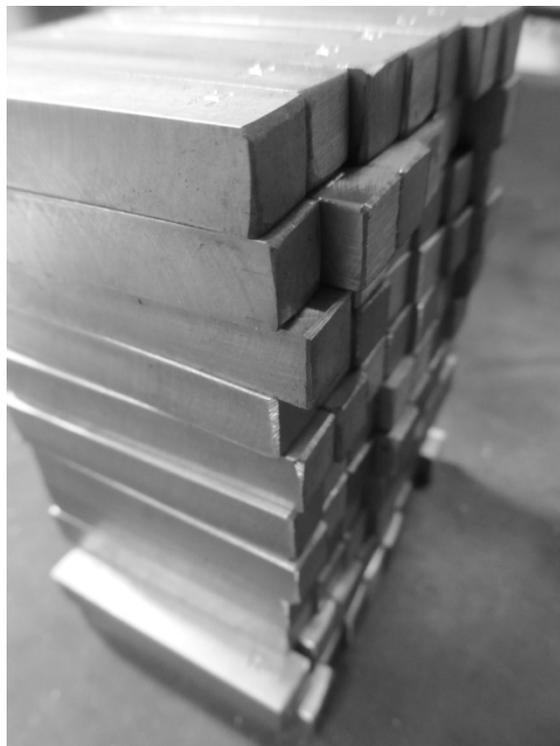
Figure 3.16. Unnotched impact testing bars.
