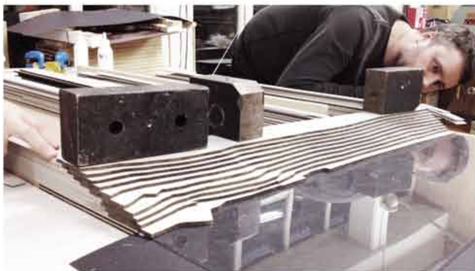
Image sequence showing the process of building the 1:200 scale model. Overlapping altitude curves are glued in layers over the glass water.
