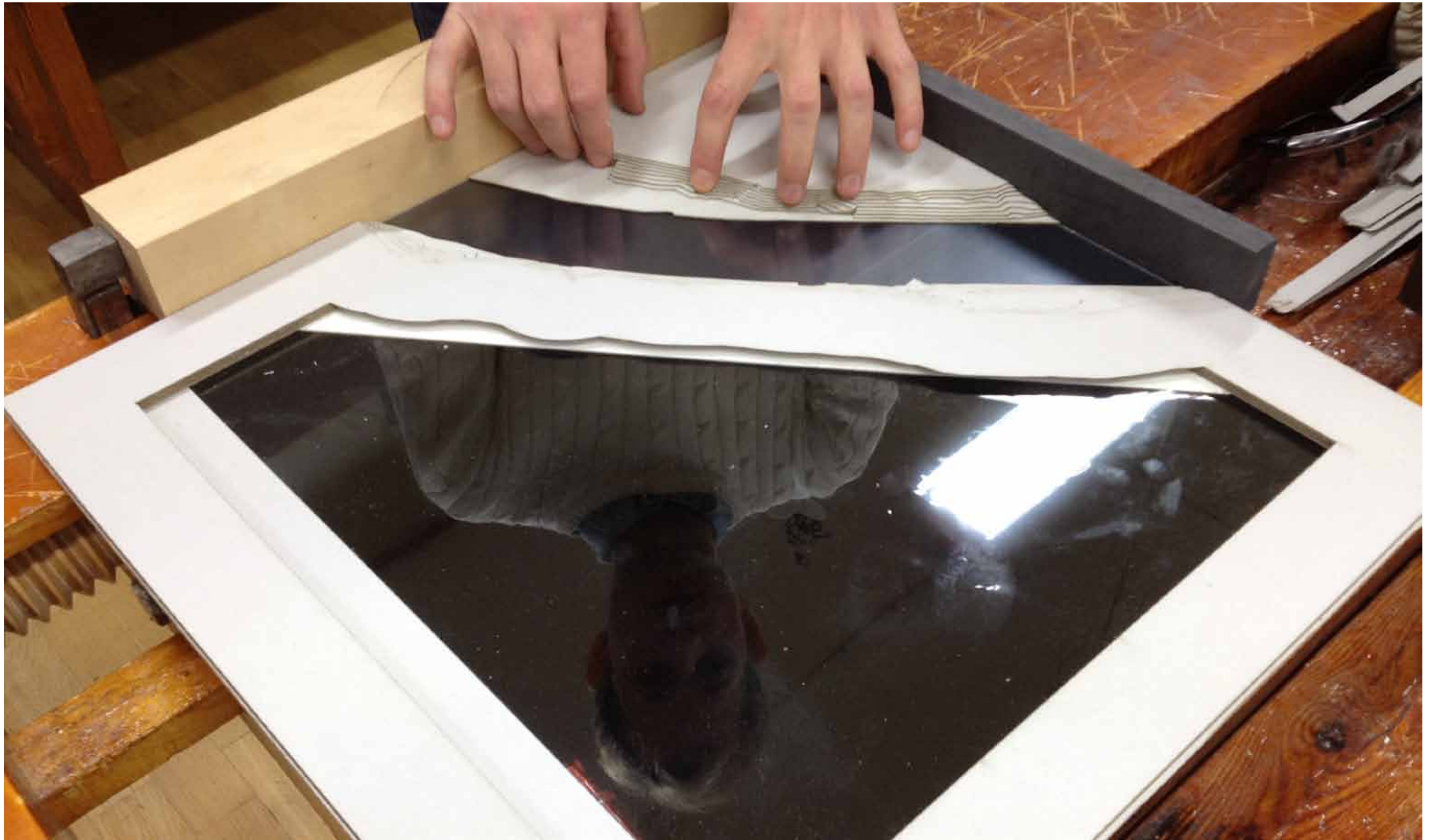
The 1:1000 site model is glued together. The sheets are hollow to save material and reduce the weight of the finished model.
